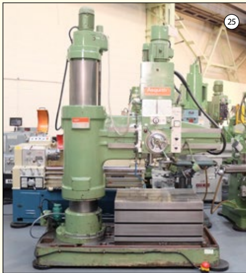
ASQUITH Type OD1 MK2 14/54: Radial Arm Drill. Radius 4'6". Spindle 4 MT (2"). Speeds 40-2040rpm. Power Locking. Box Table 40" x 30" x 20". DC Telescopic Safety Brake. £7,950
