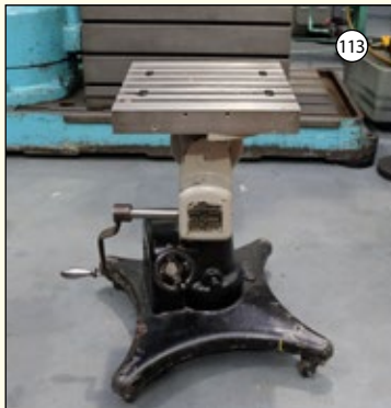
DEAN, SMITH & GRACE Tiltturn: Fitters Stand. Tilting, Turning and Rise and Fall Table. Tee Slotted Table 18" x 18".
