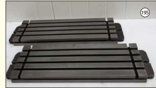
CAST IRON TEE Slotted Table(s): 76mm x 250mm x 57mm High.
