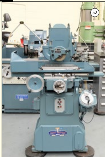
JONES & SHIPMAN 540AP: Tool Room Surface Grinder. Cap 18" x 6". Imperial Dials. Power Rise & Fall. Auto Down Feed. £4,750
