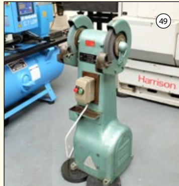
RJH Model M: Double Ended Pedestal Tool Grinder. Wheel Size 10" x 1". £225
