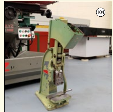
STANL: Bench Type Toggle Press. Daylight 5 1/4". Throat 3 1/4". Stroke 1 1/8". Table Size 7 3/4" x 6".
