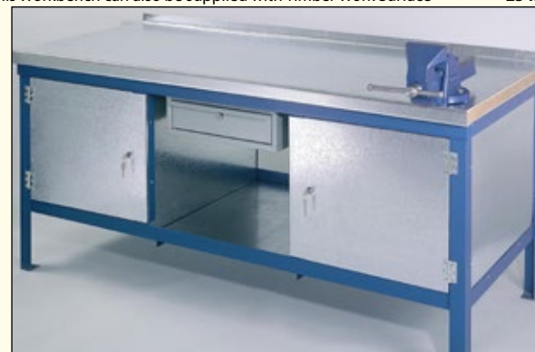
NEW WORK BENCH Model SHD2075TV: 45mm Timber with Galvanised Top, Two Cupboards, Draw and 6" Vice. 2000mm Length x 750mm Depth. £920
