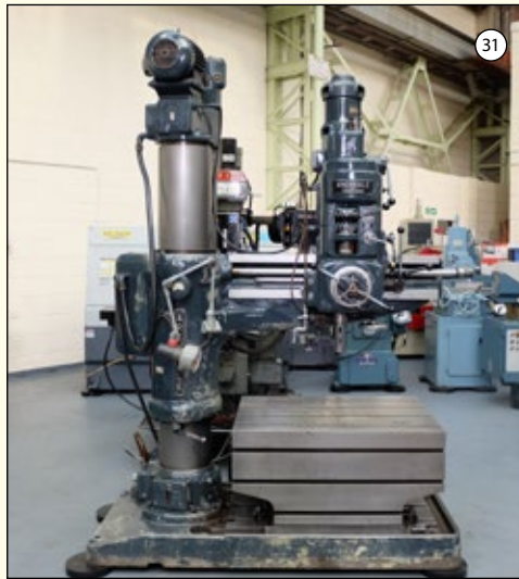
ARCHDALE: 3'6" Radial Arm Drill. 2" Drilling Capacity. Box Table 40" x 30" x 20" High. Spindle Taper No. 4 Morse. £3,750
