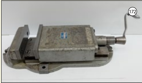
JONES & SHIPMAN: Machine Vice. Max Opening 7 3/4". Jaw Width 8 1/2". Jaw Depth 3 1/2". £325
