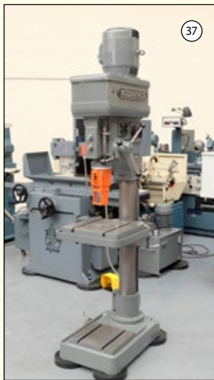
MEDDINGS: Heavy Duty Pillar Drill. Table 17" x 15". Speeds 90-1570rpm. Throat 11". 4MT. Power Feed. £2,950
