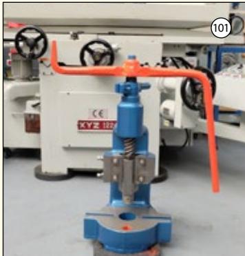
SWEENEY & BLOCKSIDE: Fly Press. Daylight 6 1/4". Throat 4 1/2". Stroke 4 1/4".
