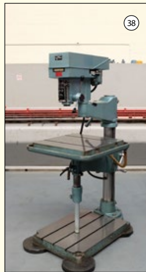
MEDDINGS A10: Articulated Arm Drill. 2 MT. Throat 24". Speeds 80-4000rpm. Rise & Fall Table. £1,950
