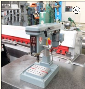
WORNER Type B4: High Speed Bench Drill. Drill Size 0-5/32". Speeds 650-12,000rpm. Drilling Depth 50mm. 180 x 160mm. £625
