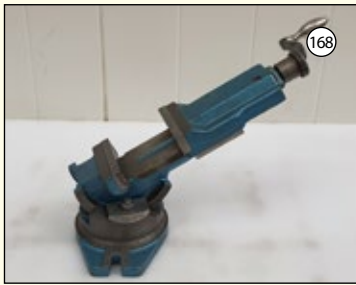
Tilting & Rotating Vice: Max Jaw Opening 850mm. Jaw Width 100mm. £275
