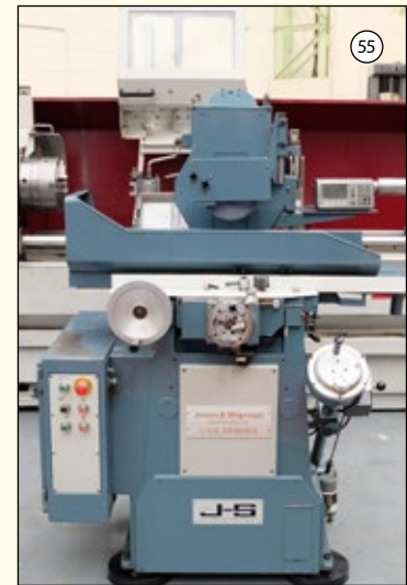
JONES & SHIPMAN 540P: Surface Grinder. Capacity 18" x 6". Power Rise & Fall. DRO on Cross Travel. £6,250
