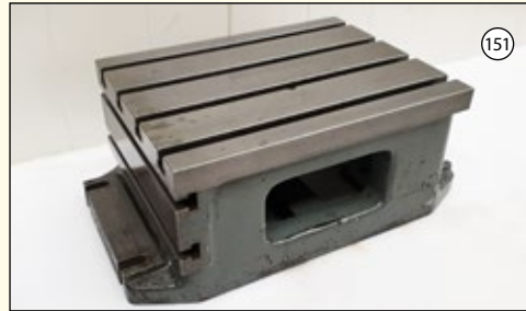
TEE Slotted Riser Block: 400mm x 300mm x 200mm High.
