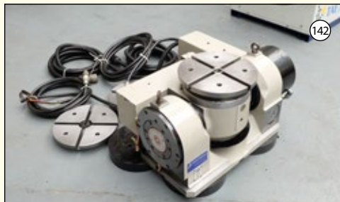
JONES & SHIPMAN: 4th AXIS Tilting Rotary Table. Size 260mm. 310mm High. ype 8414-009DC/306.
