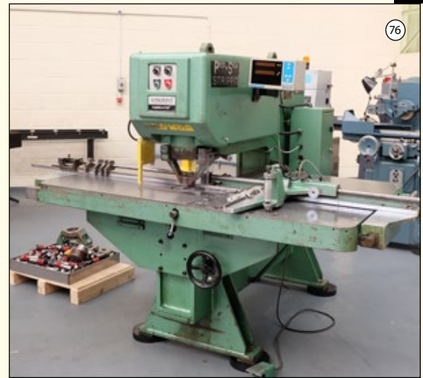
STRIPPIT SUPER 30/30/30 FABRICATOR: Capacity Punching Table 48" x 40". Copying Table 40" x 32". New Punching Guard. 2 Axis DRO. Selection of Tooling. £4,250
