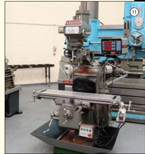
KRV 2000: Turret Milling Machine. Table Size 48" x 10". Long Travel 28". Spindle Taper R8. Speeds 60 - 4200rpm. 3 HP Variable Speed Head. Acu-Rite III 3 Axis DRO. £3,750
