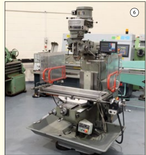
BRIDGEPORT J Type: Turret Milling Machine. Table 42" x 9". Spindle Taper R8. Spindle Speeds 67-4600rpm. Power Feed to Spindle & Table. Newall 2 Axis DRO.
