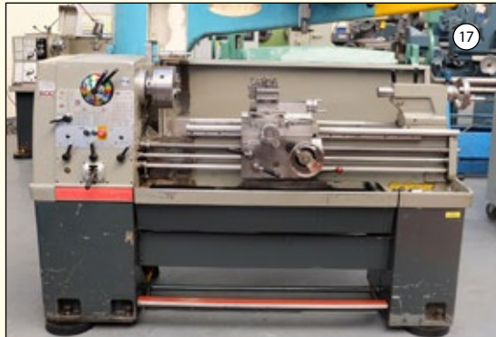
COLCHESTER STUDENT 1800: Gap Bed Centre Lathe. Swing Over Bed 13". Distance Between Centres 24". Spindle Bore 1 1/2". QCTP. 3 & 4 Jaw Chucks. £4,250
