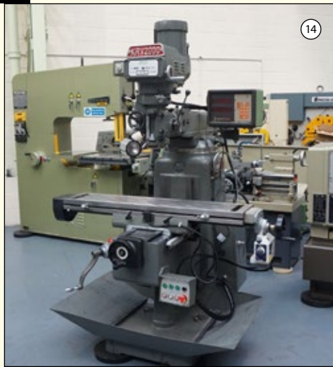
KRV 2000: Turret Milling Machine. Table Size 43" x 10". Variable Speeds 60-4200rpm. R8 Spindle Taper. Power to Table. 3 Axis DRO. Arriving Soon
