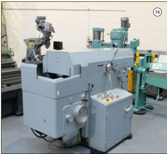
SNOW Model RT 400: Ring Grinder. Table Size 400mm Diameter. Max Height Under Wheel 200mm. Grinding Wheel Size 350mm x 25mm. Table Speeds 70- 250rpm. With 400mm Electro Mag Chuck. £8,750
