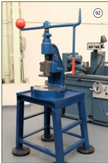
EDWARDS No. 8: Fly Press on Stand. Throat 7". Daylight 9". Stroke 6".
