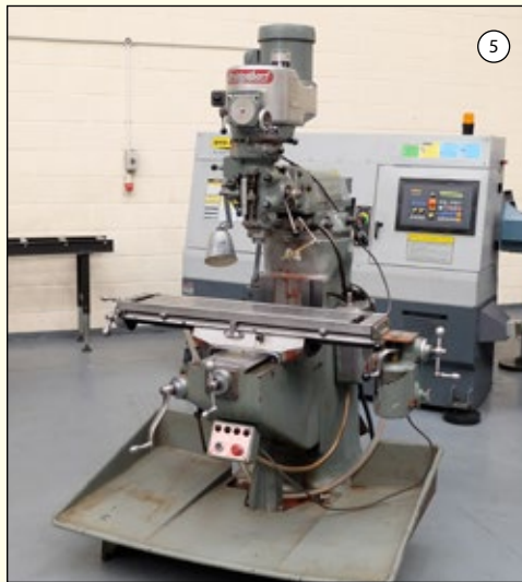
BRIDGEPORT Type BR2J2: Varispeed Turret Milling Machine. Spindle Taper R8. Table 42" x 9". Speeds 50 - 3750rpm. Swivel & Tilt Head. Power Feed to Table.
