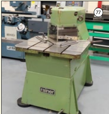
RAINER Type 300/3: Sheet Metal Hydraulic Corner Notcher. Cap 300mm x 3mm. Table Size 680mm x 840mm. Foot Control. £2,950
