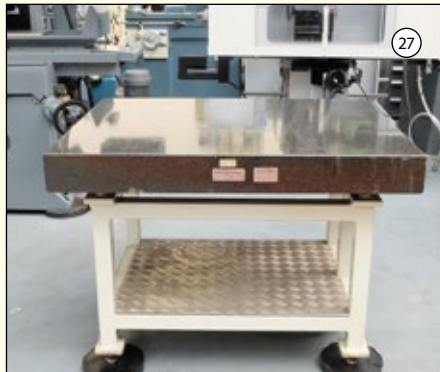
WBJ: Granite Surface Table. Surface Size 4' x 3'. Grade 1. On Leveling Stand. £1,250
