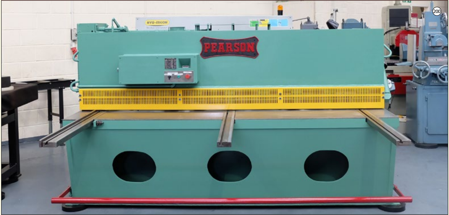
PEARSON TYPE 8 x 25: Hydraulic Guillotine. Capacity 8' x 1/4". Power Back Gauge.
