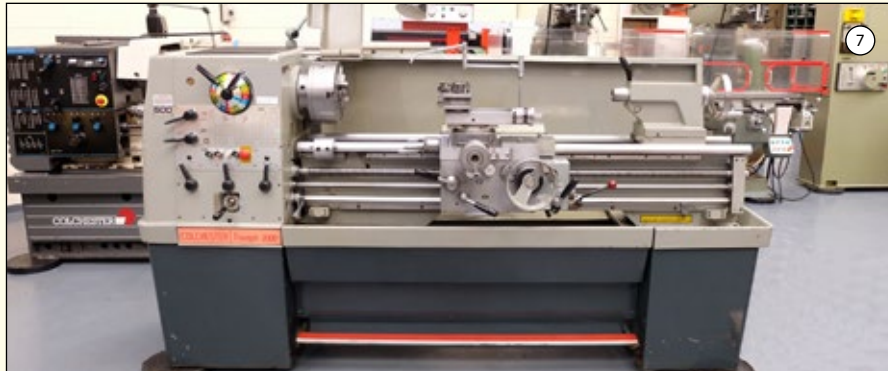
COLCHESTER TRIUMPH 2000: Gap Bed Centre Lathe. Swing Over Bed 15". Swing in Gap 22". Distance Between Centres 50". Spindle Bore 2". Spindle Speeds 25-2000rpm. 10" 3 Jaw Chuck. QCTP.
