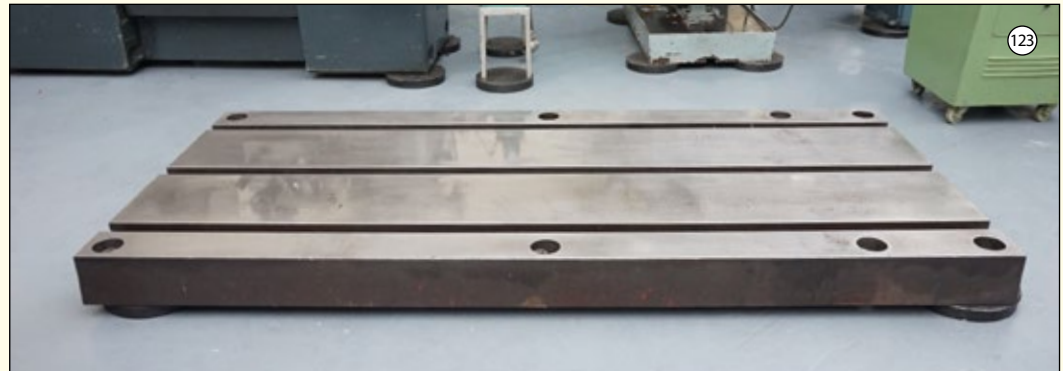
TEE SLOTTED: Bed Plates: Size 96" x 43" x 6" Deep. 3 Tee Slots. Tee Slot Sizes: 1 1/2" Width x 3" Deep. Choice of Two.
