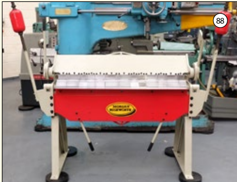
MORGAN RUSHWORTH Model BPC 1270/2.5: Manual Box & Pan Folding Machine. Capacity 1270mm x 2.5mm. 13 Pieces of Tooling: Total Length 1300mm. Year 2009.
