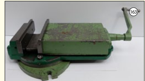
SWIVELLING MACHINE VICE: Max Jaw Opening 250mm. Jaw Width 300mm. Jaw Height 90mm. £475
