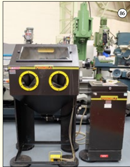
GUYSON Formula F1400: Shot Blast System. Internal Dimensions 800mm x 500mm x 500mm High. With Guyson F21 DC Single Phase Dust Extractor.
