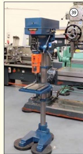
MEDDINGS Type MF5: Pillar Drill. Table 14" x 13". 3MT. Speeds 100-3000rpm. £1,450
