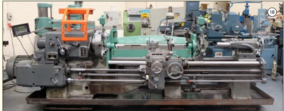
DEAN SMITH & GRACE Type 21 x 84: Gap Bed Centre Lathe. Swing Over Bed 22 1/2". Distance Between Centres 84". Swing Over Gap 30". Spindle Bore 3 1/2". Spindle Speeds 11 - 900rpm. With 3 & 4 Jaw Chucks. 3 Point Steady, QCTP. 2 Axis DRO. £9,750
