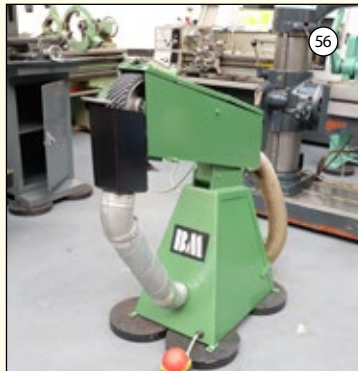
MULTITOOL MODEL BM7552: Pedestal Linisher. Belt Width 75mm. 3 Phase Motor. £850
