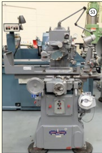
JONES & SHIPMAN 540AP: Tool Room Surface Grinder. Cap 18" x 6". Imperial Dials. Power Rise & Fall. Auto Down Feed. £4,250
