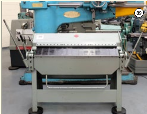
SELSON BESCO Model B&P 416: Manual Box & Pan Folding Machine. Capacity 1270mm x 1.5mm or 50" x 16swg. 16 Pieces of Tooling: Total Length 1270mm.
