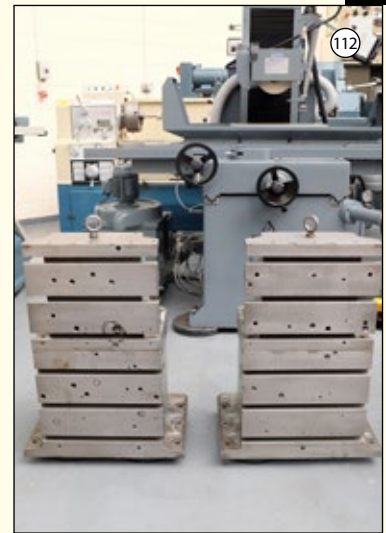
HERBERT DEVLIEG: Pair of Split Angle Plates. Lower Half: 2 off 400 x 400 x 350mm. Top Half: 2 off 420 x 350 x 330mm.
