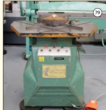
COMACA: Sheet Metal Corner Notcher. Capacity 220mm x 4mm.
