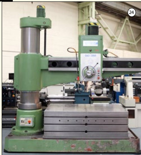
KITCHEN & WALKER Type G63 - 2000: Radial Arm Drill. Radius 2000mm. Spindle 5 MT (3"). Speeds 20 - 1600rpm. Box Table Size 70" x 43" x 23". £11,250
