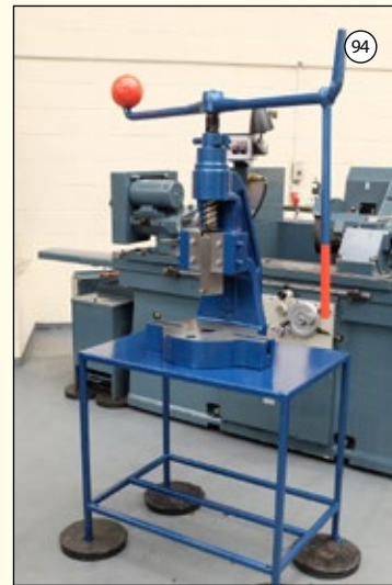
NORTON No. 6S: Fly Press on Steel Stand. Throat 6". Daylight 9".
