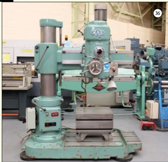
MASTYEV R2: 3' Radial Arm Drill. Spindle Taper No. 3 Morse. Speeds 90-4500rpm. Drilling Depth 8 1/4". Power Feed to Spindle. Box Table 20" x 16" x 16".
