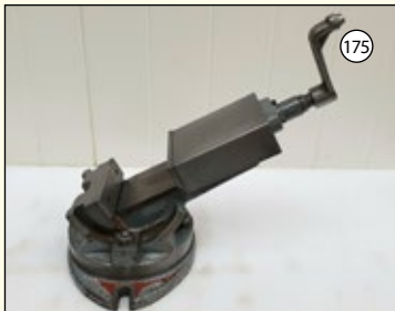
ABWOOD: Tilting & Rotating Vice. Jaw Width 6". Jaw Height 2". £475
