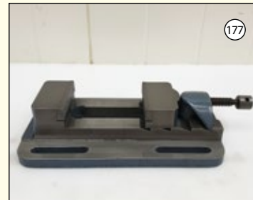
JONES & SHIPMAN: Rack Vice. Max Opening 5". Jaw Width 4". Jaw Depth 1 1/2". £425
