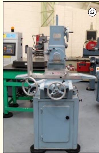
EXE: Toolroom Precision Manual Surface Grinder. Table Capacity 12" x 6". Fitted to EXE Pedestal Cabinet. £2,750
