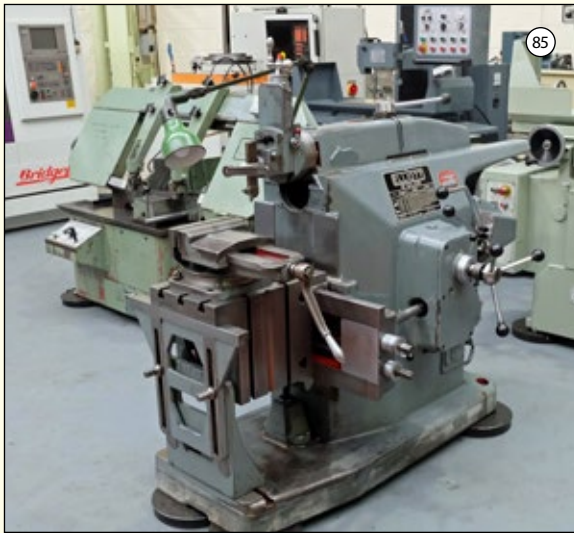
ELLIOTT 18" MAJOR: Shaping & Slotting Machine. Capacity 18". Strokes 12-110/min. 6 Speeds 4-125 fpm. Feeds 0 - 0.060. Table Size 18" x 12". Swivel Vice 9 1/4".
