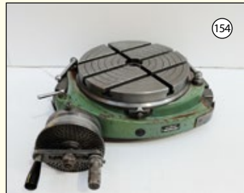
WALTER: Tee Slotted Rotary Table. 380mm Diameter. 120mm Height.
