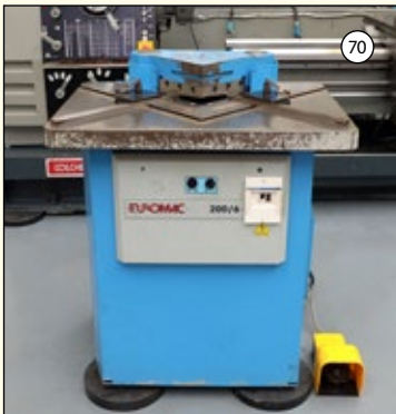
EUROMAC Type 200/6: Hydraulic Sheet Metal Corner Notcher. Capacity 200mm x 6mm (8" x 1/4").
