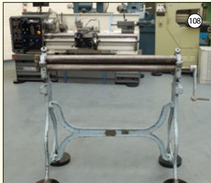
EE Co. Ltd: Initial Pinch Sheet Metal Rolls. Length of Rolls 41 1/2". Diameter of Rolls 2 1/2".
