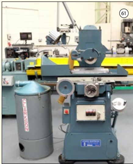
JONES & SHIPMAN 540: Surface Grinder. Capacity 18" x 6". With Dust Extractor. £3,750
