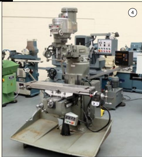
BRIDGEPORT Type BR2J2: Varispeed Turret Milling Machine. Spindle Taper R8. Spindle Speeds 50-3250rpm. Table 42" x 9". Power Feed to Table. 2 Axis DRO.
