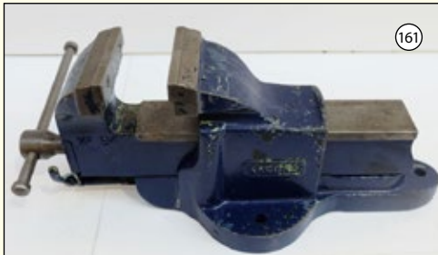
RECORD No.24: Quick Release Bench Vice. Max Opening 7 1/4". Jaw Width 5 1/4". Jaw Height 4". £275
