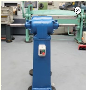
CANNING Type L53L: Double Ended Polishing Machine. Spindle Diameter 1 3/4". Motor 3 HP. 2020rpm. £1,650
