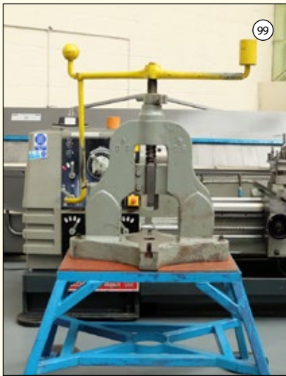
DENBIGH 6 DS: Double Sided Fly Press. 12" Between Sides. 9" Daylight. Centre to Side 6". Bar Press Holes.
