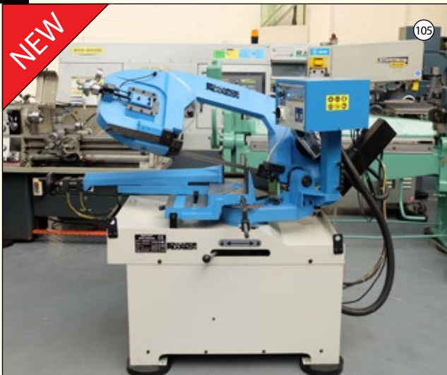
EDWARDS PEARSON MBS370SA: Semi-Auto Double Swivel Bandsaw. Power Rise & Fall Bow. Variable Down Feed. Hydraulic Cycle Vice Clamping Up to 60 Deg Right Angle Cutting by Manual Movement of Bow. Capacity Round 270mm. £6,250
