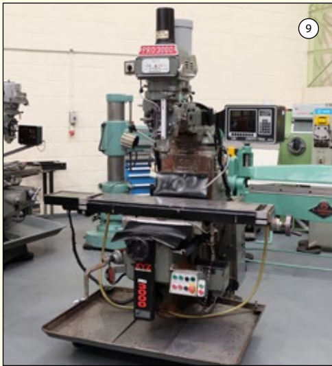
XYZ PRO3000: Turret Mill. With Prototrak MX2 Two Axis Programmable Control. Table 54" x 12". Long Travel 32". Speeds 70-3600rpm. Taper 40 ISO. Power Drawbar. £7,250
