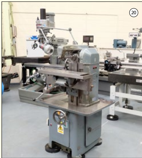
ACIERA F3: Horizontal Milling Machine. Table 700mm x 190mm. Spindle Speeds 155 - 2500rpm.
