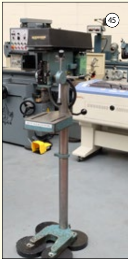
MIDDINGS Model DTF: Pillar Drill. Speeds 500-4000rpm. Throat 7 1/2". 1/2" Drill Chuck. 3 Phase. £750
