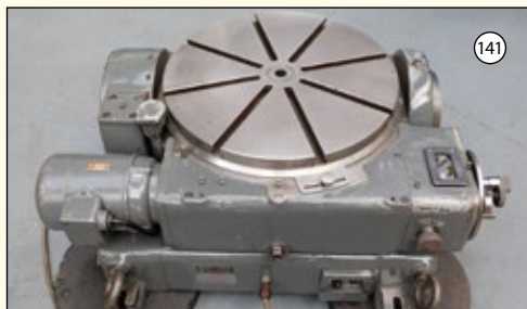
HERBERT LINDLER: Precision Tool Room Motorised Rotary Table. 440mm Diamater. Motor 0-15kw/110 Volt.
