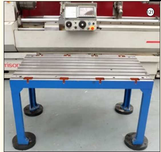
TEE SLOTTED: Light Duty Work Table. Size 48" x 27". 9 Tee Slots.
