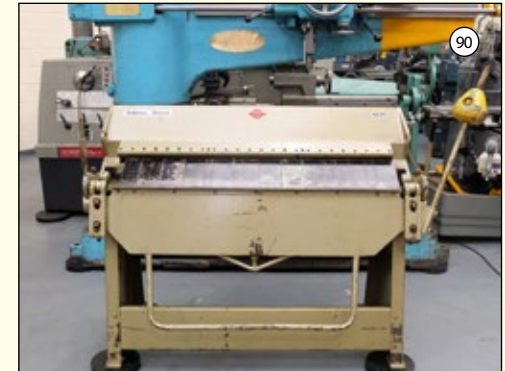
SELSON BESCO Model B&P 416: Manual Box & Pan Folding Machine. Capacity 1250mm x 1.6mm or 50" x 16swg. 16 Pieces of Tooling: Total Length 1240mm.
