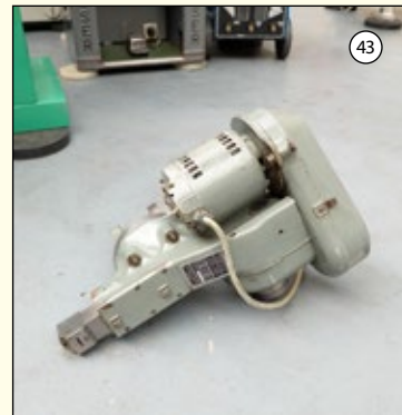
BRIDGEPORT: Slotting & Shaping Head. Stroke: 1/8 - 4". 6 Speeds: 60 - 350 s/min. £1,250
