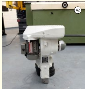
BRIDGEPORT: Slotting & Shaping Head. Stroke: 1/8 - 4". 6 Speeds: 60 - 350 s/min. £950
