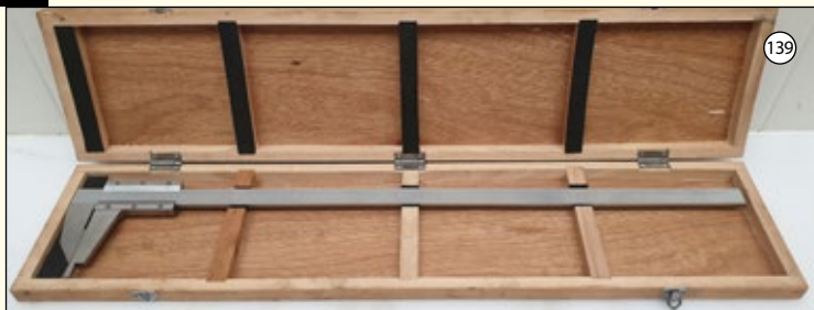
STAINLESS HARDEND STEEL: Vernier Caliper. Metric and Imperial. Capacity 24". 600mm.
