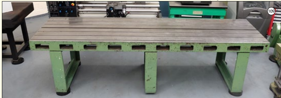
CAST IRON: Surface Table With Central Tee Slot. Size 11' 11 1/2" x 40". Thickness 7". Work Height 38". One Tee Slot in Centre. Six Straight Slots.
