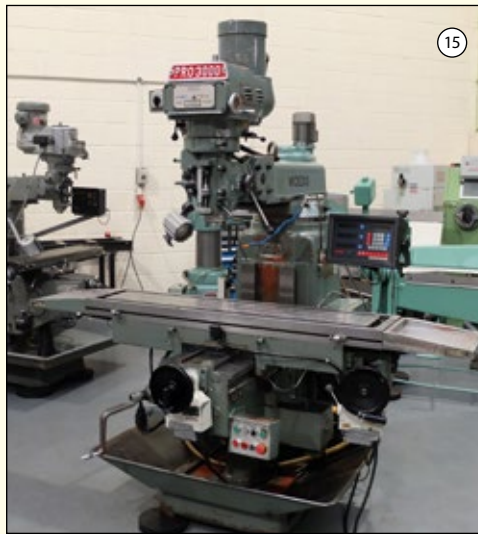
KRV PRO 3000 SLV: Varispeed Turret Milling Machine. Table 58" x 12". Long Travel 40". Spindle Taper 40 ISO. Speeds 70-3600rpm. Power Feeds & Rapids to X & Y. £2,750
