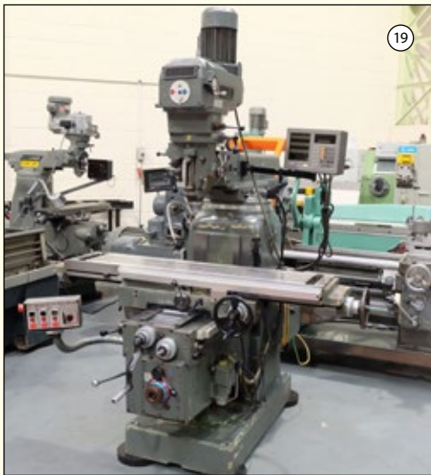
AJAX Model AJT4: Turret Milling Machine. Table Size 54" x 11". Axis: Longitudinal 31 1/2", Cross 13 1/2", Vertical 16". Taper 40 ISO. Speeds 75-4000rpm. Metric Dials. 3 Axis DRO. £3,250
