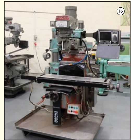
KRV PRO 2000: Turret Milling Machine. With ProtoTrak A.G.E. 2 Control. Table 50" x 10". Travel: Long 30", Cross 16". Taper R8. Speeds 60-4200rpm. 3HP Variable Speed Head. £2,250
