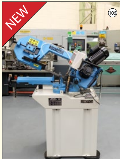
EDWARDS PEARSON MBS270FHE: Gravitational Bandsaw. Hydraulic Down Feed. Quick Release Vice Clamping. Capacity Round 220mm. £2,950
