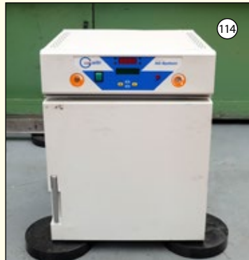
FRATELLI GALLI Model G-2100: Oven. Appature 300mm x 300mm x 250mm Deep. Max Temp 300 Deg, Single Phase.
