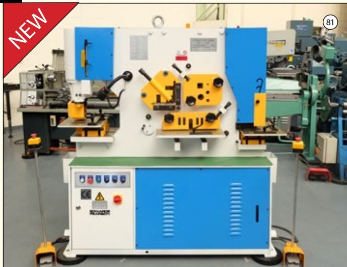
EDWARDS PEARSON Q35Y-16: Hydraulic Steelworker. Section Cutting: 45mm Round. 40mm Square. Punching: 25mm Dia x 16mm Thickness. Notching: 100 x 57 x 10mm Thickness Shearing: 16 x 250mm or 8 x 400mm Right Angle: 125 x 125 x 12mm. £10,250
