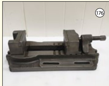
RACK VICE: Max Opening 9 1/2". Jaw Width 6". Jaw Depth 3 1/2". £125
