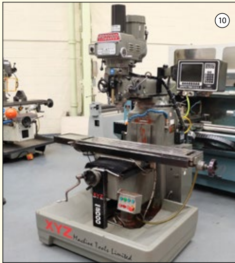
XYZ PRO2000: Programmable Turret Mill. 2 AXIS AGE 2 Control. Table Size 50" x 10". Spindle Taper R8. Speeds Variable 60 - 4200rpm. Power Drawbar. Arriving Soon
