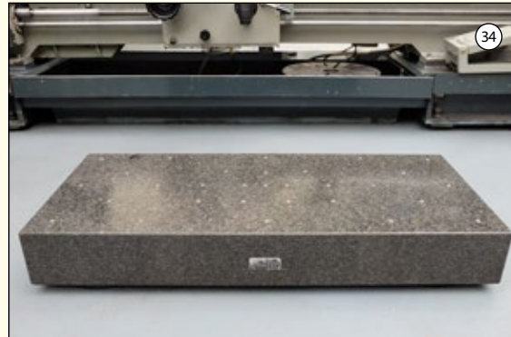
GRANITE TABLE: Surface Size 59" x 26". Thickness 7 1/2". Grade A. With 30 Clamp Studs. £600
