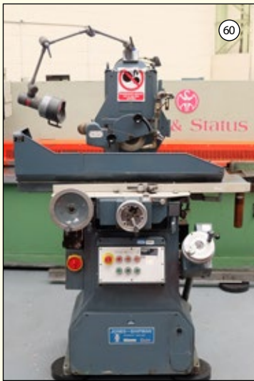
JONES & SHIPMAN 540P: Surface Grinder. Capacity 18" x 6". Power Rise & Fall. Magnetic Chuck 14" x 6". £4,950
