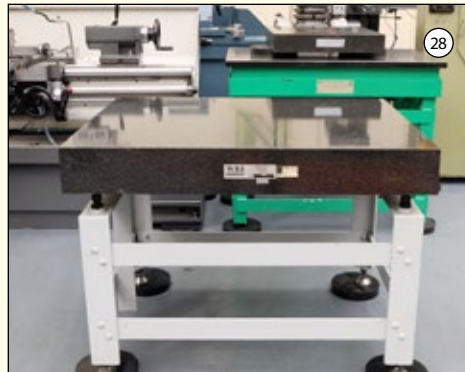
WBJ: Granite Surface Table. Grade 1. Surface Size 48" x 36". Thickness 6". On Leveling Stand. £1,250
