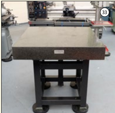
WBJ METROLOGY: Granite Surface Table. Surface Size 1000mm x 1000mm. Thickness 150mm. £950
