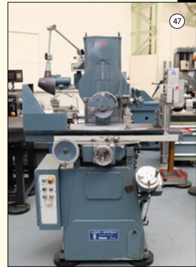
JONES & SHIPMAN 540L: Tool Room Surface Grinder. Grinder. Cap 8" x 6". Height Under Wheel 16". Long Column. Power Rise & Fall. £5,950
