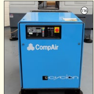
COMPAIR Model Cyclon 111: Rotary Air Compressor. Max Pressure 7.5 Bar. Flow Rate 1.77m 3 /Min. Motor Power 13.59kw.
