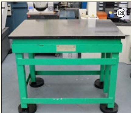
SURFACE FLATNESS: Cast Iron Surface Table. Surface Size 48" x 30". Grade 1.
