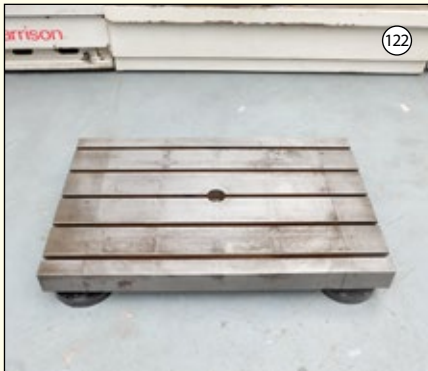
TEE SLOTTED: Machine Table. 5 Tee Slots. Size 48" x 30".
