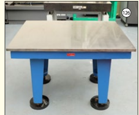
CAST IRON: Surface Table. Surface Size 4' x 3'. Grade B.
