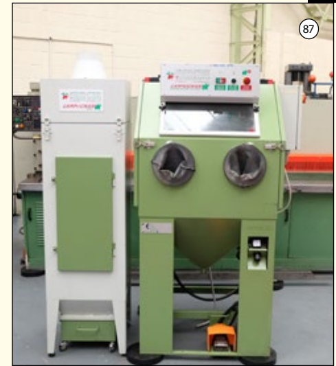
LAMPUGNANI LC-05: Sand Blasting Machine. Max Pressure 8 Bar. Internal Dimensions 800 x 600 x 700mm. Extraction Unit. Dust Collection Cabinet. Work Hours 211.
