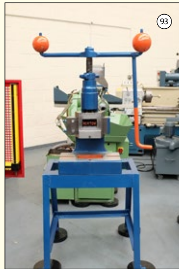
NORTON No. 4GP: Fly Press On Stand. Table Size 19" x 10". Throat 5". Daylight 7". Table Throughhole 8" x 3".
