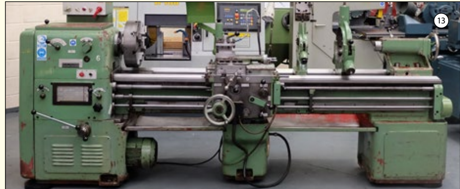
WAFUM Model 50/2000: Centre Lathe. Swing Over Bed 500mm. Distance Between Centres 2000mm. Spindle Bore 55mm. Spindle Speeds 18 - 1800rpm. 3 Jaw Chuck. 4 Jaw Chuck. 2 & 3 Point Steadies. £4,750
