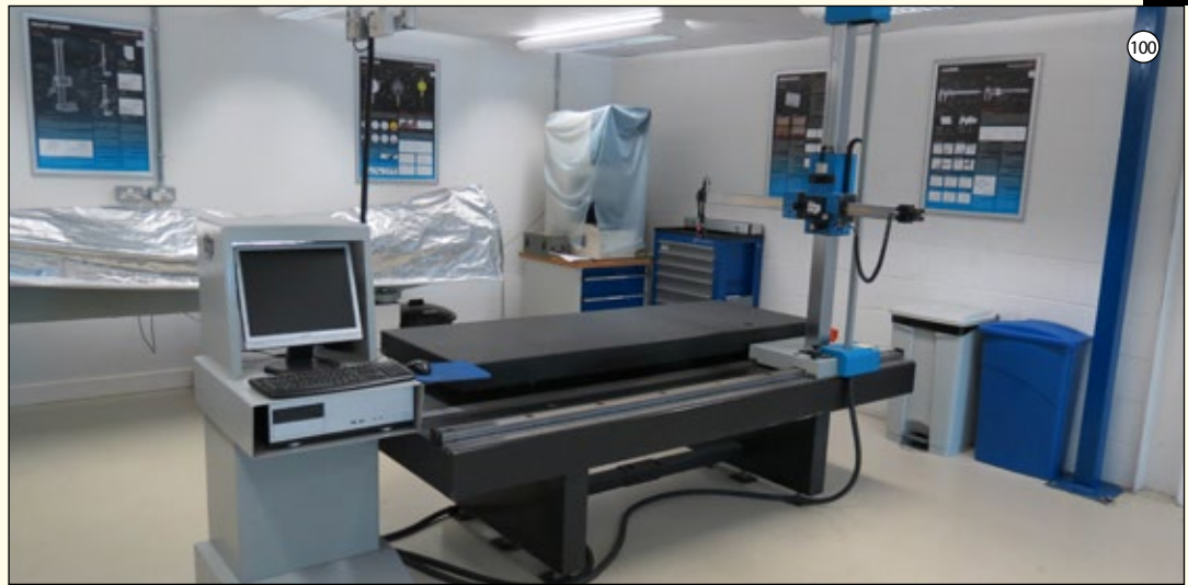
ITP Type HA8: Coordinate Measuring Machine. Fixed to Granite Table Size 2500 x 1150mm. Measuring Table 2000 x 700mm. X Axis 2000mm, Y Axis 700mm, Z Axis 1000mm. Reinshaw Probes MH20i & TP20. Software - Axel.
