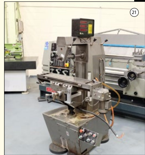
VICEROY AEW: Horizontal Milling Machine. Table 35" x 8". Power Feed in X Axis. Spindle Taper 30 ISO. 2 Axis DRO. £1,650
