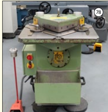
BOSCHERT PN4: Sheet Metal Corner Notcher. Capacity: 225mm x 225mm x 4mm Mild Steel. 225mm x 225mm x 3mm Stainless Steel. £1,950
