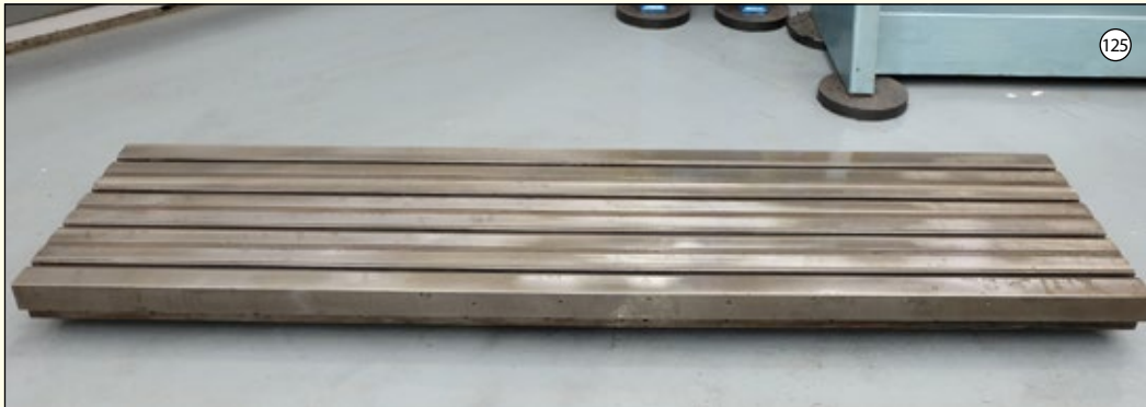
TEE SLOTTED: Steel Bed Plate. Size 8' x 2'. Thickness 4 1/2". 4 Tee Slots.
