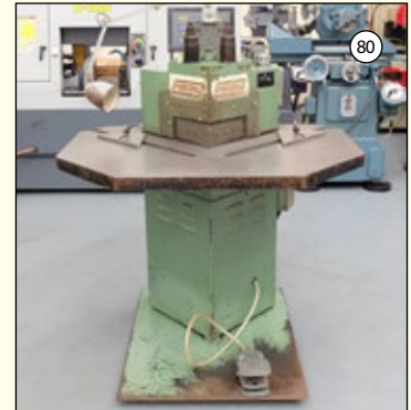
PIERCEALL: Sheet Metal Corner Notcher. Capacity: 200mm x 200mm x 3mm. Table Size 42" x 27". Foot Control. £1,250
