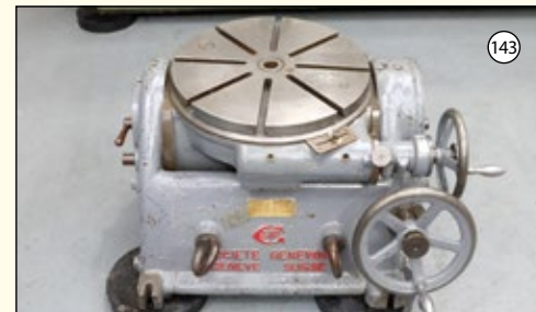
SIP Type P1-5B. Tilting Rotary Table. Diameter 450mm. Work Height 400mm. Tee Slotted.
