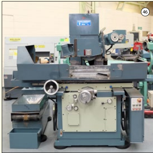
JONES & SHIPMAN Type 1415: Toolroom Surface Grinder. Capacity 27" x 12". Distance Under New Wheel 1 1/4". Power Rise & Fall to Wheelhead. With Magnetic Chuck & Coolant Tank. £12,750
