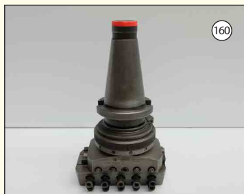
WOHLHAUPER UPAS: Universal Boring & Facing Head. 50 ISO Taper. 22mm Tool Size.
