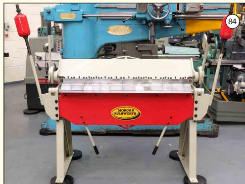
MORGAN RUSHWORTH BPC 1270/2.5: Sheet Metal Box & Pan Folder. Capacity 1270 x 2.5mm. Year 2000. 13 Pieces of Tooling Total Length 1300mm.
