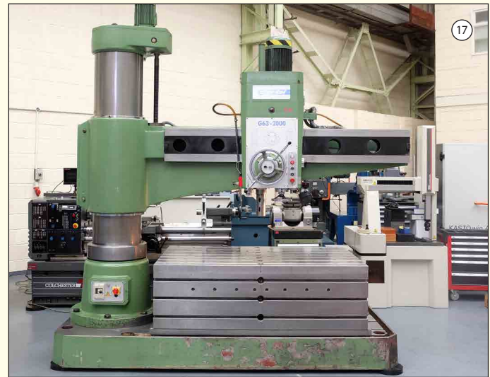
KITCHEN & WALKER Type G63 - 2000: Radial Arm Drill. Radius 2000mm. Spindle 5 MT. Speeds 20-1600rpm. Drilling Capacity 63mm. Box Table Size 70" x 43" x 23".
