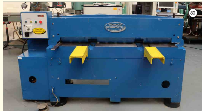
MORGAN RUSHWORTH Model SC1500/6: Electric Power Guillotine. Capacity 1550mm x 6mm. Strokes 40 Per Min. Front Operated Power Back Gauge. Metric Readout. Foot Control. Motor 7.5kw, Rear Interlocking Gates.
