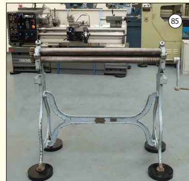
EE Co. Ltd: Initial Pinch Sheet Metal Rolls. Diameter of Rolls 2 1/2". Length of Rolls 41 1/2".
