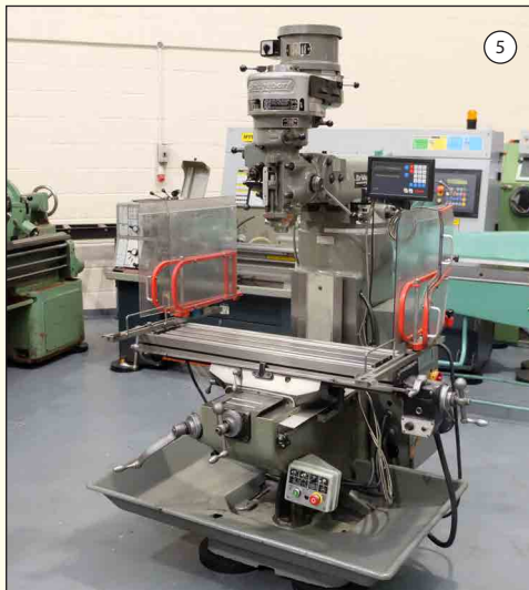
BRIDGEPORT J Type: Turret Milling Machine. Table 42" x 9". Spindle Taper R8. Spindle Speeds 67-6400rpm. Power Feed to Spindle & Table. Newall 2 Axis DRO.
