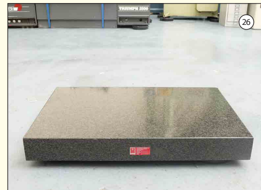
SURFACE FLATNESS: Granite Surface Plate. Size 3' x 2'. Thickness 4".
