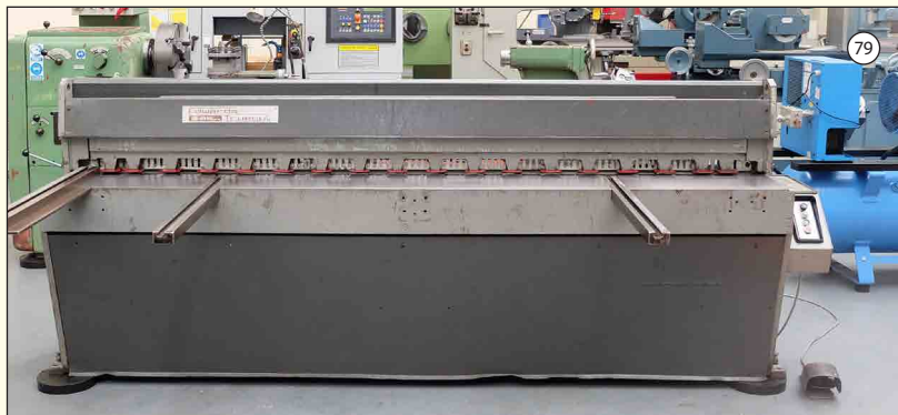
EDWARDS PEARSON Type DD: Power Guillotine. Capacity 2540mm x 3.25mm. Blade Gap Adjustment. Manual Back Gauge. Front Supports.
