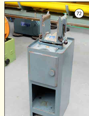
J&S 2101/0G1: Wheel Balancing Unit. 145mm Between Blades. 160mm Deep. With Stand.
