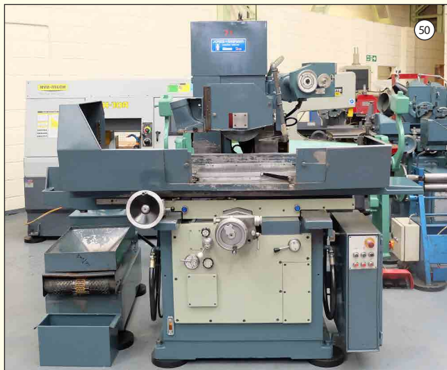
JONES & SHIPMAN Type 1415: Toolroom Surface Grinder. Capacity 27" x 12". Distance Under New Wheel 11 3 / 4 ". Power Rise & Fall to Wheelhead. Mag Chuck & Coolant Tank.
