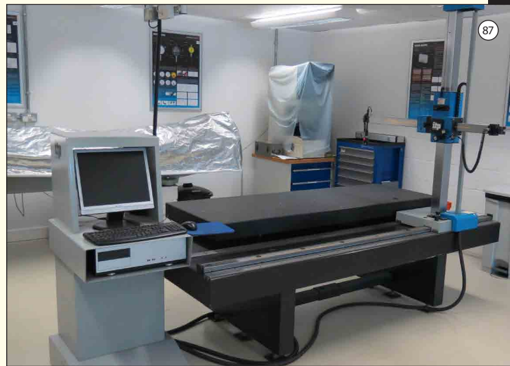
ITP Type HA8: Coordinate Measuring Machine. Fixed to Granite Table Size 2500 x 1150mm. Measuring Table 2000 x 700mm. X Axis 2000mm, Y Axis 700mm, Z Axis 1000mm. Reinshaw Probes MH20i & TP20. Software - Axel. £13,750
