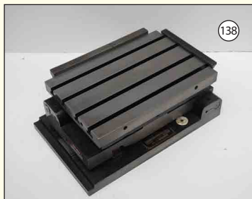
CROWN: Tee Slotted Two Way Sine Table. Size 300mm x 200mm x 130mm High. £525
