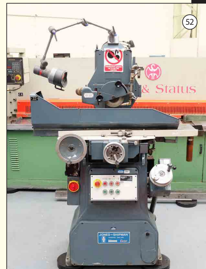
JONES & SHIPMAN 540P: Surface Grinder. Capacity 18" x 6". Power Rise & Fall. Magnetic Chuck 14" x 6".
