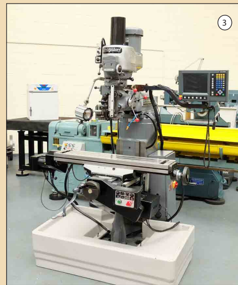
BRIDGEPORT BR2J2: Varispeed Turret Milling Machine With Acu-Rite PWR 2 Axis CNC System. Taper R8. Table Size 42" x 9". 3 Axis DRO. Rebuilt in 2005.
