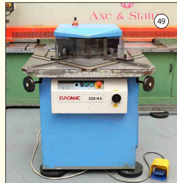
EUROMAC Type 220/4S: Sheet Metal Hydraulic Corner Notcher. Capacity 200mm x 200mm x 4mm. Variable Angle. £2,500
