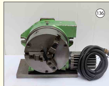
YAMATOKOKI: Model PDX 10. Power Rotary 3 Jaw Chuck. Vertical/Horizontal. £1,750
