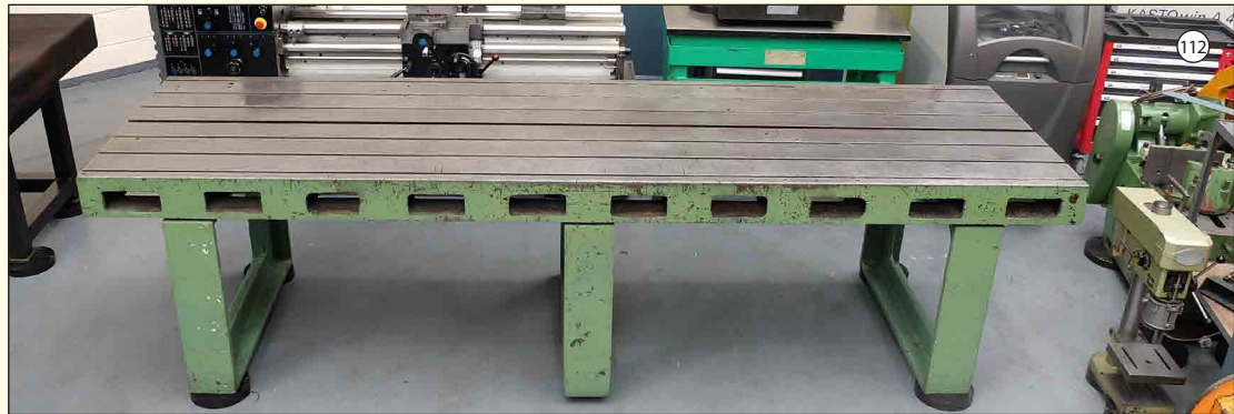
CAST IRON: Surface Table With Central Tee Slot. Size 11' 11 1/2" x 40". Thickness 7". Work Height 38". One Tee Slot in Centre. Six Straight Slots.
