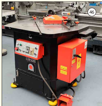
AMADA Type CSW-220: Hydraulic Sheet Metal Corner Notcher. Cap 200mm x 2mm. Rear Square Notcher: 100mm x 50mm. £2,750
