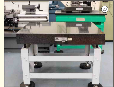
WBJ: Granite Surface Table. Grade 1. Surface Size 48" x 36". Thickness 6". On Leveling Stand.
