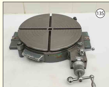
TAYLOR - HOBSON: Tee Slotted Rotary Table. 12" Diameter.
