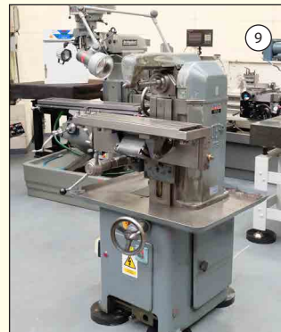
ACIERA F3: Horizontal Milling Machine. Spindle Speeds 155-2500rpm. Table Size 700mm x 190mm.
