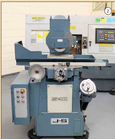
JONES & SHIPMAN 540P: Surface Grinder. Capacity 18" x 6". With Coolant Tank. Power Rise & Fall to Wheel Head.
