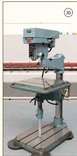
MEDDINGS A10: Articulated Arm Drill. 2 MT. Throat 24". Speeds 80-4000rpm.
