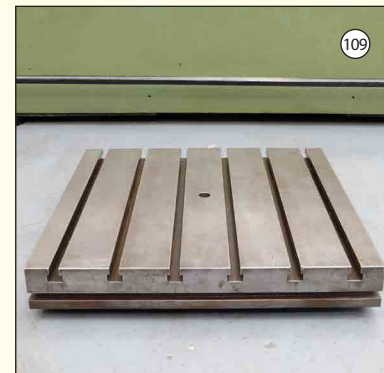
TEE SLOTTED: Cast Iron Plate. Size 36" x 36" x 5". 6 x Tee Slots.
