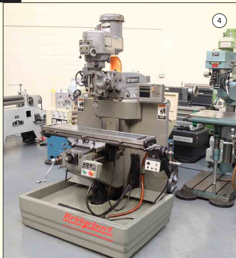
BRIDGEPORT BR2J2: Varispeed Turret Milling Machine. Spindle Taper R8. Spindle Speeds Up to 3250rpm. Table 48" x 9". Power Feed to Table. 2 Axis DRO.
