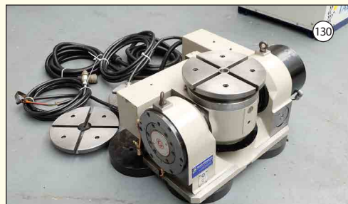
JONES & SHIPMAN: 4th AXIS Tilting Rotary Table. Size 260mm. 310mm High. ype 8414-009DC/306.
