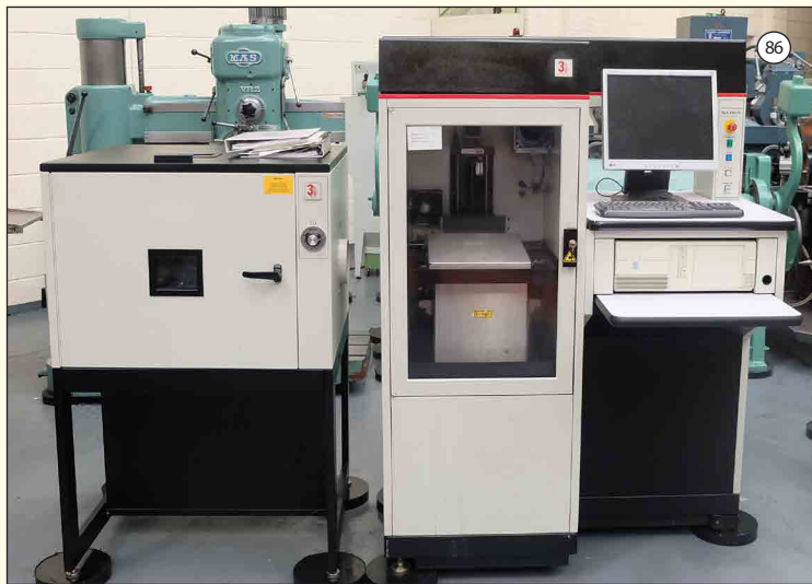
3D SYSTEMS MODEL SLA 250/50 HR: Stereolithography System. Laser Type HeCd/325nm. Part Capacity 250mm x 250mm x 250mm. Software 3D Lightyear. Max Part Weight 9kg. Power 6MW. Recoating Process: Zephyr. VAT Capacity 32.2 LtL. Year 2004. £5,750
