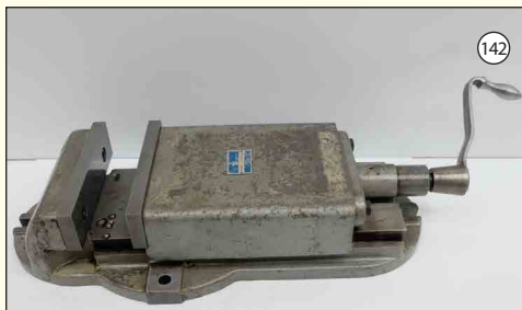
JONES & SHIPMAN: Machine Vice. Max Opening 7 3/4". Jaw Width 8 1/2". Jaw Depth 3 1/2". £325
