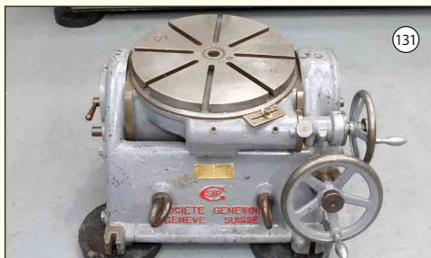
SIP Type P1-5B. Tilting Rotary Table. Diameter 450mm. Work Height 400mm. Tee Slotted.
