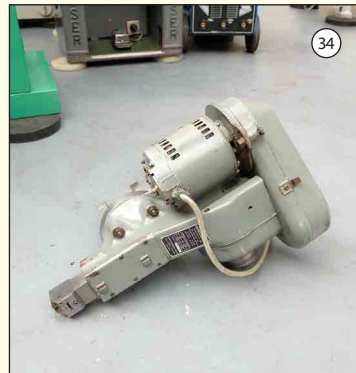
BRIDGEPORT: Slotting & Shaping Head. 6 Speeds: 60 - 350 s/min. Stroke: 1/8 - 4".
