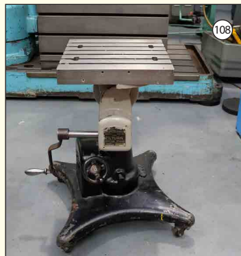
DEAN, SMITH & GRACE Tiltturn: Fitters Stand. Tilting, Turning and Rise and Fall Table. Tee Slotted Table 18" x 18". £1,250
