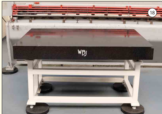
WBJ: Granite Surface Table. Surface Size 1500mm x 1000mm. On Leveling Stand.
