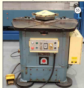
AMADA Type CSW-220: Hydraulic Sheet Metal Corner Notcher. Cap 200mm x 2mm. Rear Square Notcher: 100mm x 50mm.
