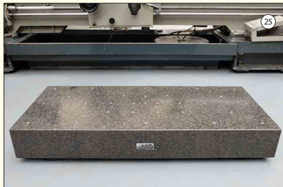
GRANITE TABLE: Surface Size 59" x 26". Thickness 7 1/2". Grade A. With 30 Clamp Studs.
