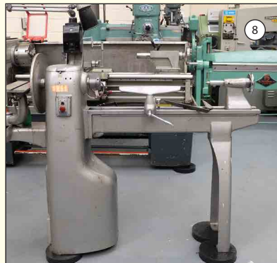
UNION GRADUATE: Pedestal Wood Turning Lathe. Swing Over Bed 12". Between Centres 30". Speeds 425-2250rpm. 14" Dia Disk Sander.
