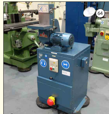
RJH: Vertical Bandfacer on Dust Extractor. Belt Size 100mm x 915mm. Motor 0.75kw. 3 Phase 415V. £1,175
