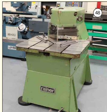
RAINER Type 300/3: Sheet Metal Hydraulic Corner Notcher. Cap 300mm x 3mm. Table Size 680mm x 840mm. Foot Control. £2,750
