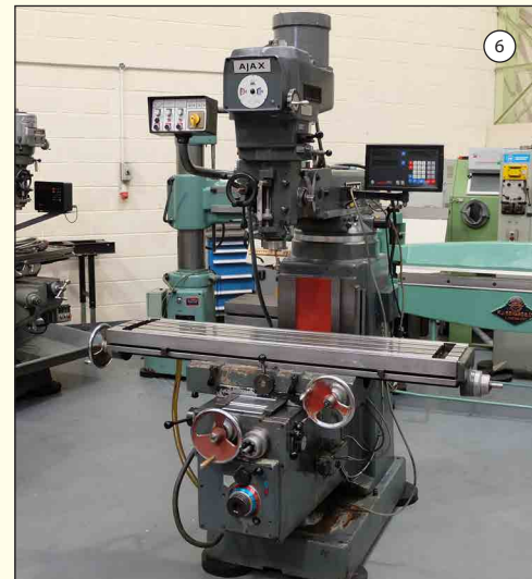
AJAX Model AJT4: Turret Milling Machine. Table Size 54" x 11". Axis: Longitudinal 31 1/2", Cross 13 1/2", Vertical 16". Taper 40 ISO. Speeds 75-4000rpm. Metric Dials. 2 Axis DRO.
