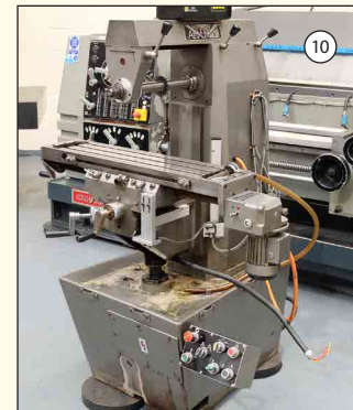
VICEROY AEW: Horizontal Milling Machine. Table 35" x 8". Taper 30 ISO. Power Feed in X Axis.
