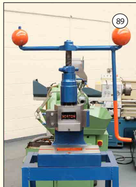
NORTON No. 4GP: Fly Press On Stand. Table Size 19" x 10". Throat 5". Daylight 7". £950
