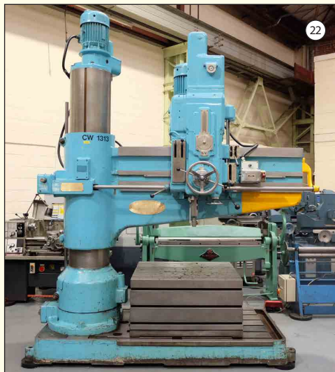
KITCHEN & WADE Type E27 HD: 6' Radial Arm Drill. Arm Radius 72". Drilling Cap 3". 5MT. Speeds 8.5-800rpm. Drilling Depth 18". Box Table 42" x 36" x 22" High. Telescopic Brake.
