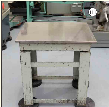
CAST IRON SURFACE TABLE: 30" x 24" x 31 1/2" High.
