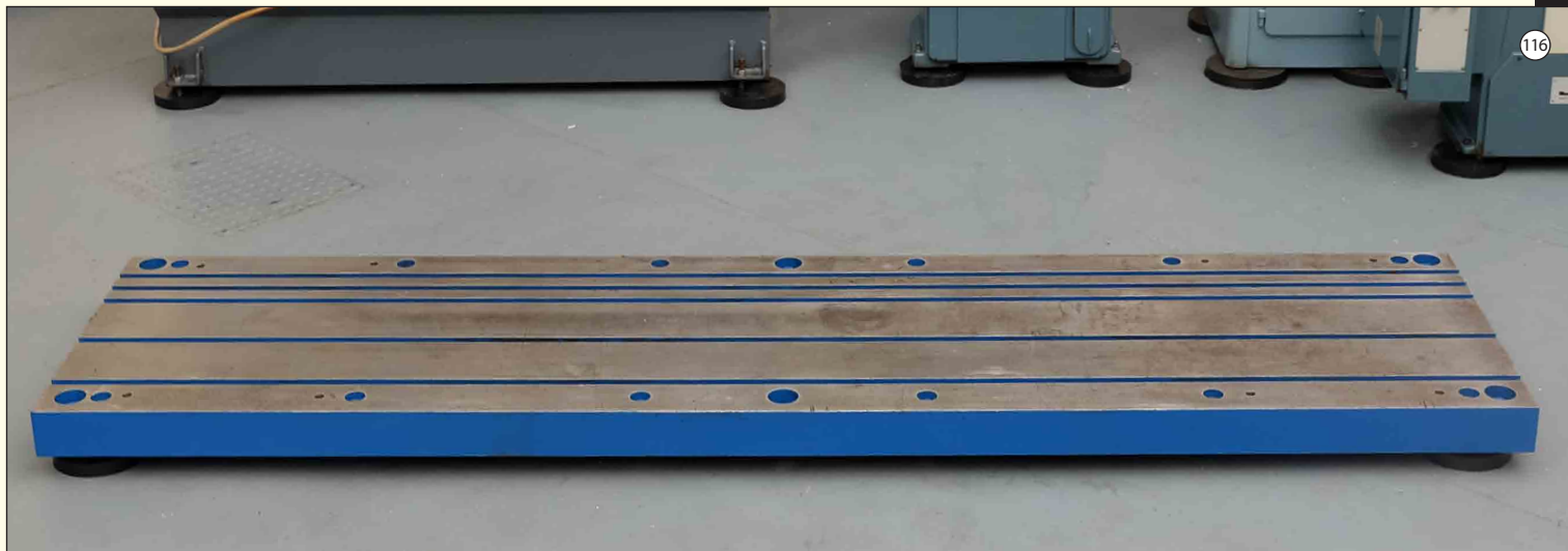
TEE SLOTTED: Floor Plate: Size 146" x 35" x 5" Thickness. 5 x Tee Slots.
