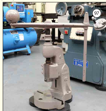
DENBIGH No4: Fly Press. Throat 4 1/2". Daylight 7 1/2". Approx Tonnage 4. £425
