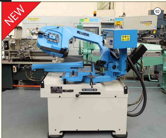
EDWARDS PEARSON MBS370SA: Semi-Auto Double Swivel Bandsaw. Power Rise & Fall Bow. Variable Down Feed. Hydraulic Cycle Vice Clamping Up to 60 Deg Right Angle Cutting by Manual Movement of Bow. Capacity Round 270mm. £6,250
