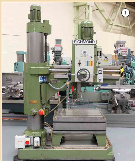
RICHMOND ENVOY: 48" Radial Arm Drill. Radius 48". Spindle Speeds 20-928rpm. Spindle To Base 50". Spindle 4 MT. Spindle Guard. Telescopic Brake.
