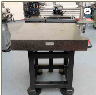
WBJ METROLOGY: Granite Surface Table. Surface Size 1000mm x 1000mm. Thickness 150mm.
