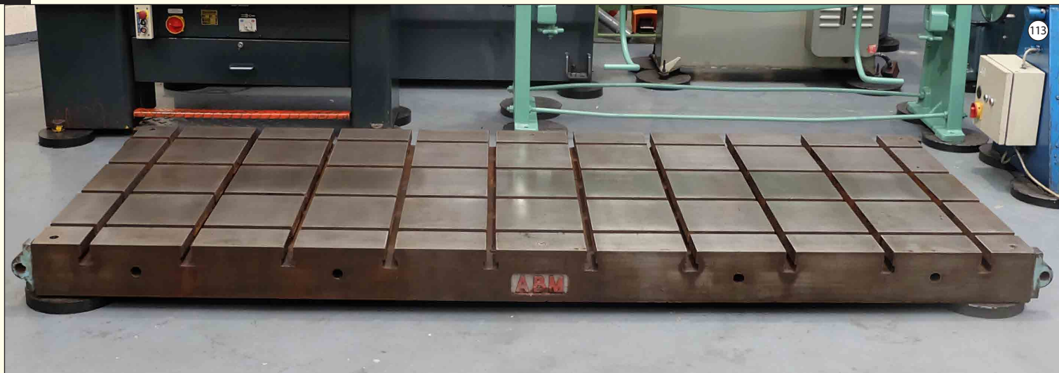
ABM: Tee Slotted Floor Plate. Size 10' x 4'. Thickness 7". 1" Tee Slots. Tee Slotted Both Ways.
