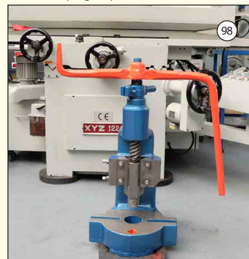
SWEENEY & BLOCKSIDGE: Fly Press. Daylight 6 1/4". Throat 4 1/2". Stroke 4 1/4". £375
