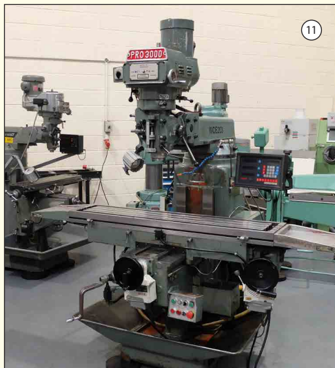
KRV PRO 3000 SLV: Varispeed Turret Milling Machine. Table 58" x 12". Long Travel 40". Spindle Taper 40 ISO. Speeds 70-3600rpm. Power Feeds & Rapids to X & Y. £4,750
