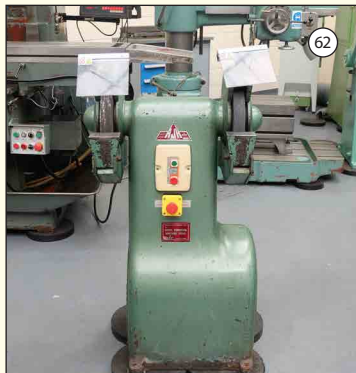
RJH BISON: Double Ended Tool Grinder. Wheel Size 300mm x 38mm x 35mm. 35mm Bore. With Wheel Guards. £750
