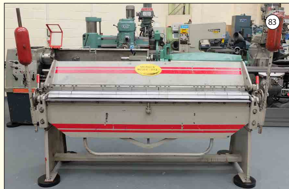
MORGAN RUSHWORTH: Sheet Metal Box & Pan Folder. Capacity 80" x 14swg.
