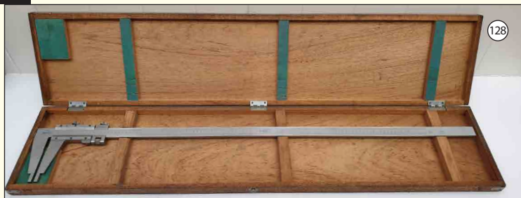
MITUTOYO: Vernier Caliper. Stainless Steel. 1000mm Capacity.
