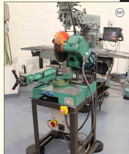
PEDRAZZOLI TYPE BROWN 300: Bench Top Chop Saw. Blade Diameter 300mm.
