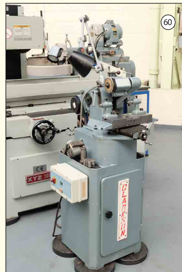
CLARKSON MKII: Tool & Cutter Grinder. Cap 12" x 6". Pair of Centres. Universal Head. £1,250
