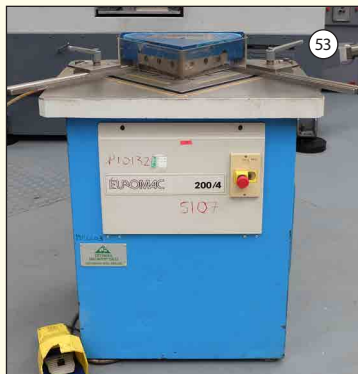
EUROMAC Type 200/4: Hydraulic Sheet Metal Corner Notcher. Cap 200mm x 2mm. 2 x Angle Guides. Rear Depth Stop.
