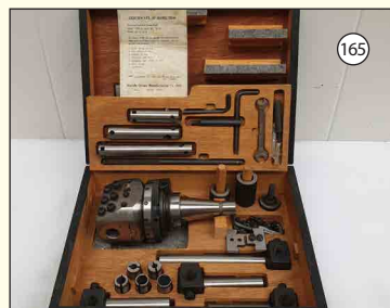
KURODA UFB-4: Boring & Facing Head. 40 Int Taper, 5 1/8" Drawbar Thread
