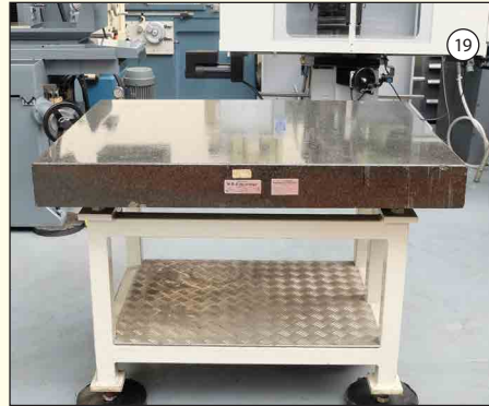
WBJ: Granite Surface Table. Surface Size 48" x 36" Grade 1. On Leveling Stand.
