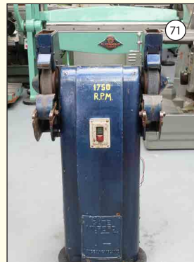
GATE MILFORD: Double ended Tool Grinder. Wheel Size 12" x 1 1 / 2 ".
