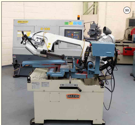
BAILEIGH Type BS350M: Horizontal Metal Cutting Bandsaw. Capacity Round 240mm.
