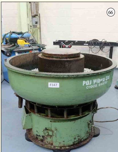
PDJ VIBRO Ltd: Vibratory Circular Bowl Finisher. Capacity 200ltr. Size 1300mm Diameter. Trough Size 300mm. Bowl Height 950mm.
