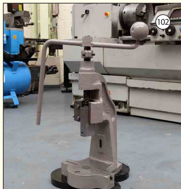
NORTON Type 2L: Fly Press. Daylight 10". Throat 5".
