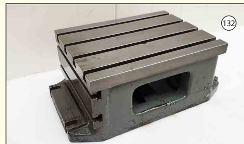
TEE Slotted Riser Block: 400mm x 300mm x 200mm High.
