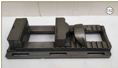
JONES & SHIPMAN: Rack Vice. Max Opening 385mm. Jaw Width 205mm.
