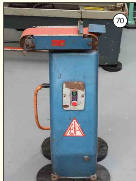
RJH: Horizontal Belt Sander. Belt 4" x 12". Fitted to Pedestal Stand.
