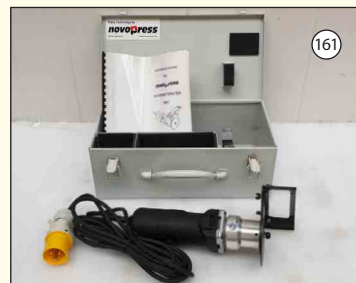
GEBRIT MAPRESS: Deburrer. No-Load Linear Speed 10000-29000r/Min.
