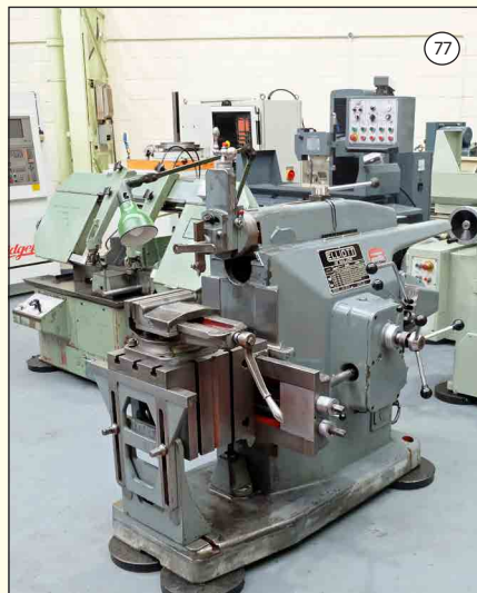
ELLIOTT 18" MAJOR: Shaping & Slotting Machine. Cap 18". Strokes 12-110/min. 6 Speeds 4-125 fpm. Feeds 0-0.060. Table 18"x12". Swivel Vice 9 1/4".
