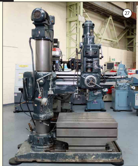
ARCHDALE: 3'6" Radial Arm Drill. 2" Drilling Capacity. Spindle Taper No. 4 Morse. Box Table 40" x 30" x 20" High.
