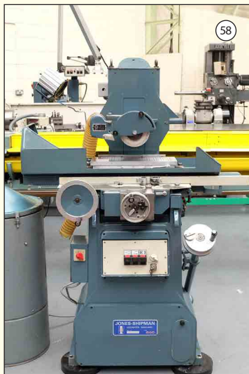
JONES & SHIPMAN 540: Surface Grinder. Capacity 18" x 6". Dust Extractor. £3,750
