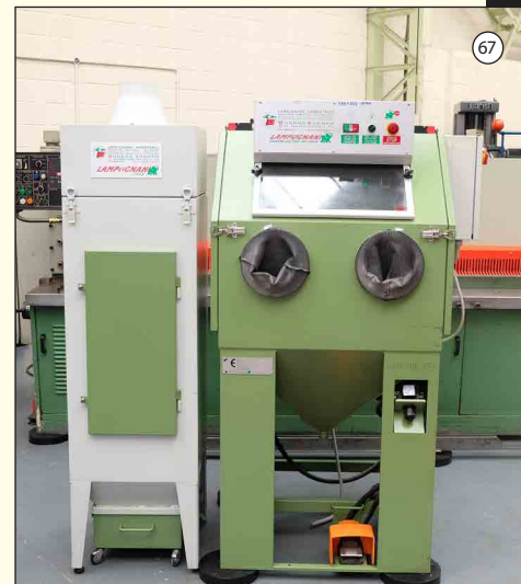
LAMPUGNANI LC-05: Sand Blasting Machine. Max Pressure 8 Bar. Internal Dimensions 800 x 600 x 700mm. Extraction Unit. Work Hours 211.
