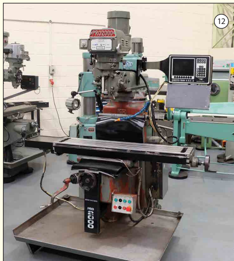
KRV PRO 2000: Turret Milling Machine. With ProtoTrak A.G.E 2 Control. Table 50" x 10". Travel: Long 30", Cross 16". Taper R8. Speeds 60-4200rpm. 3HP Variable Speed Head. £5,250
