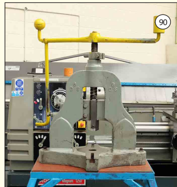
DENBIGH 6 DS: Double Sided Fly Press. 12" Between Sides. 9" Daylight. Centre to Side 6". Bar Press Holes. £750
