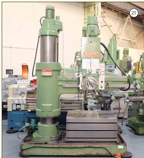
ASQUITH Type OD1 MK2 14/54: Radial Arm Drill. Radius 4'6". Spindle 4 MT. Speeds 40-2040rpm. Box Table 40" x 30" x 20". Power Locking. DC Telescopic Safety Brake.
