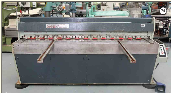
EDWARDS TRUECUT MODEL 3.25/2000 DD: Power Guillotine. Capacity 2015mm x 3.25mm. Motor Size 7.5kw. 3 Phase.
