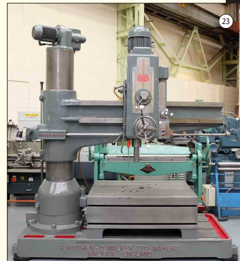
KITCHEN & WALKER Type E3: Radial Arm Drill. Radius 6'. Drilling Cap 1/4" - 3". Spindle 5MT. Speeds 12-1000rpm. Table 50" x 36" x 20" High. DC Brake. Coolant System.
