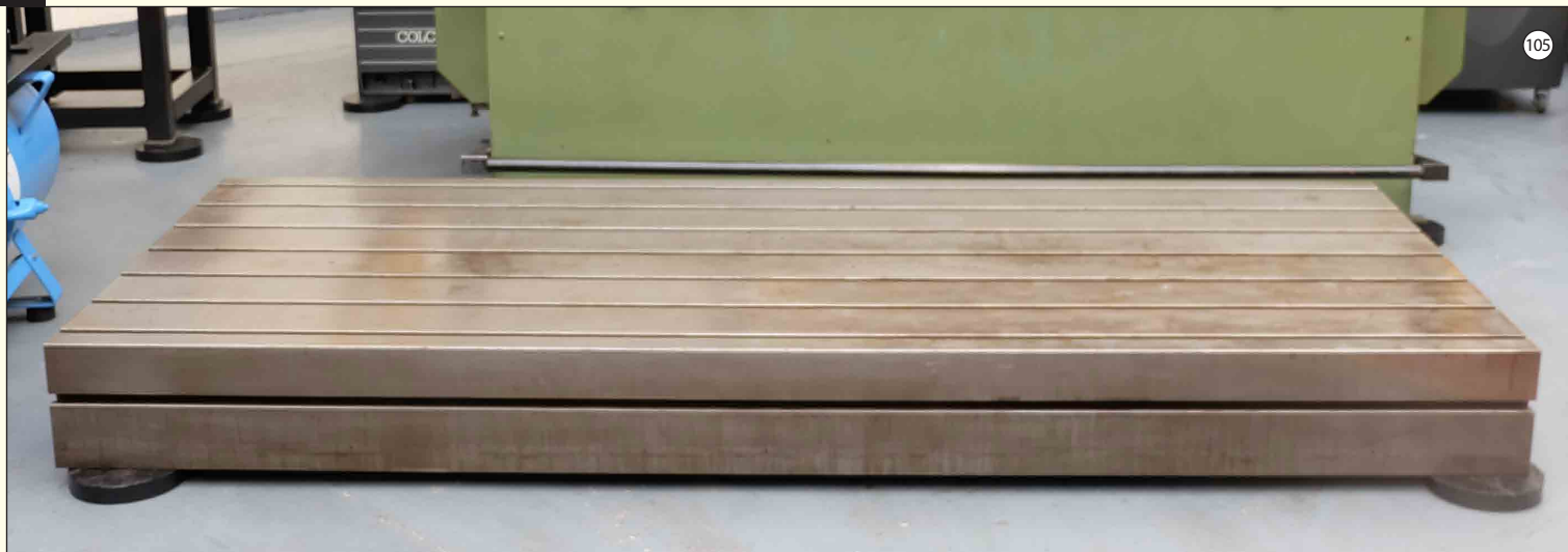
TEE SLOTTED: Machined Floor Plate/Base Plate. 7 x Tee Slots on Surface. 1 x Tee Slot on Front. Size 3300mm x 1200mm x 270mm Thickness.
