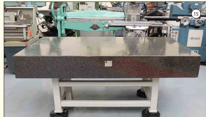
ELEY METROLOGY: Granite Surface Table on Leveling Stand. 2000mm x 1000mm x 260mm.
