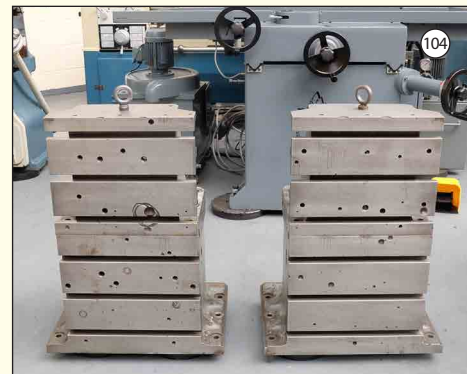
HERBERT DEVLIEG: Pair of Split Angle Plates. Lower Half: 2 off 400 x 400 x 350mm. Top Half: 2 off 420 x 350 x 330mm.
