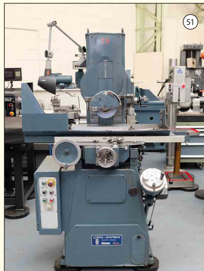
JONES & SHIPMAN 540L: Tool Room Surface Grinder. Capacity 18" x 6". Power Rise & Fall. Height Under Wheel 16". Long Column.
