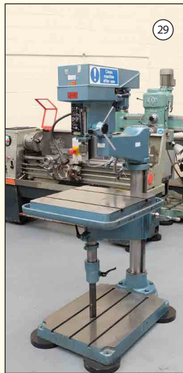
MEDDINGS A10/3: Articulated Arm Drill. 3 MT. Throat 24" Speeds 80-4000rpm.
