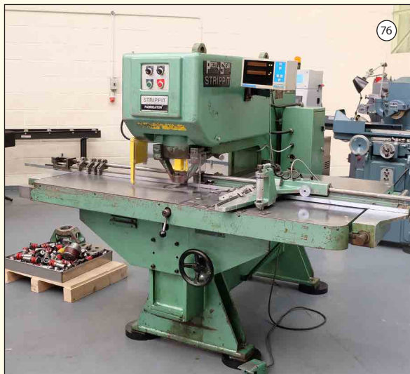
STRIPPIT SUPER 30/30/30 FABRICATOR: Made by Press & Shear. Capacity: Punching Table 48" x 40". Copying Table 40" x 32". New Punching Guard. 2 Axis DRO. Selection of Tooling.
