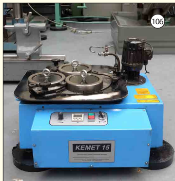
KEMET 15VS: Bench Top Diamond Flat Lapping/Polishing Machine. 380mm Diam Lapping Table. 240v, Variable Speed. £2,750
