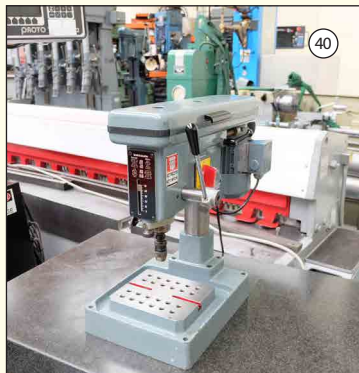
WORNER Type B4: High Speed Bench Drill. Drill Size 0-5/32". Speeds 650-12,000rpm. Drilling Depth 50mm. 180 x 160mm. £575
