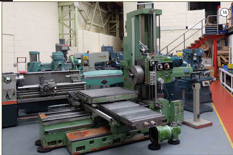
CERUTI TYPE ABC 75: Wide Bed Horizontal Boring, Milling & Facing Machine. Speeds 15-1500rpm. Spindle Dia 75mm. Table Size 850 x 1100mm. Cross Traverse 1600mm. Long Traverse 1500mm. Facing Head 450mm. With Swiveling Vertical Milling Head & Tooling.
