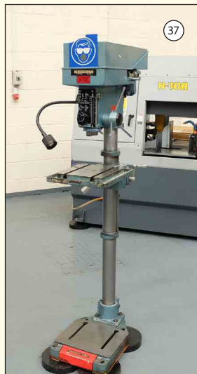
MEDDINGS MF4/3: Pillar Drill. No. 2 MT. Speeds 80-4000rpm. Table Size 11" X 10". £1,250
