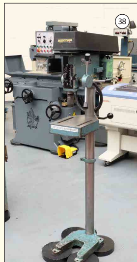
MEDDINGS Model DTF: Pillar Drill. Speeds 500-4000rpm. Throat 7 1/2". 1 1/2" Drill Chuck. 3 Phase. £750
