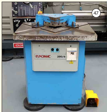
EUROMAC Type 200/6: Hydraulic Sheet Metal Corner Notcher. Capacity 200mm x 6mm (8" x 1/4"). £2,750
