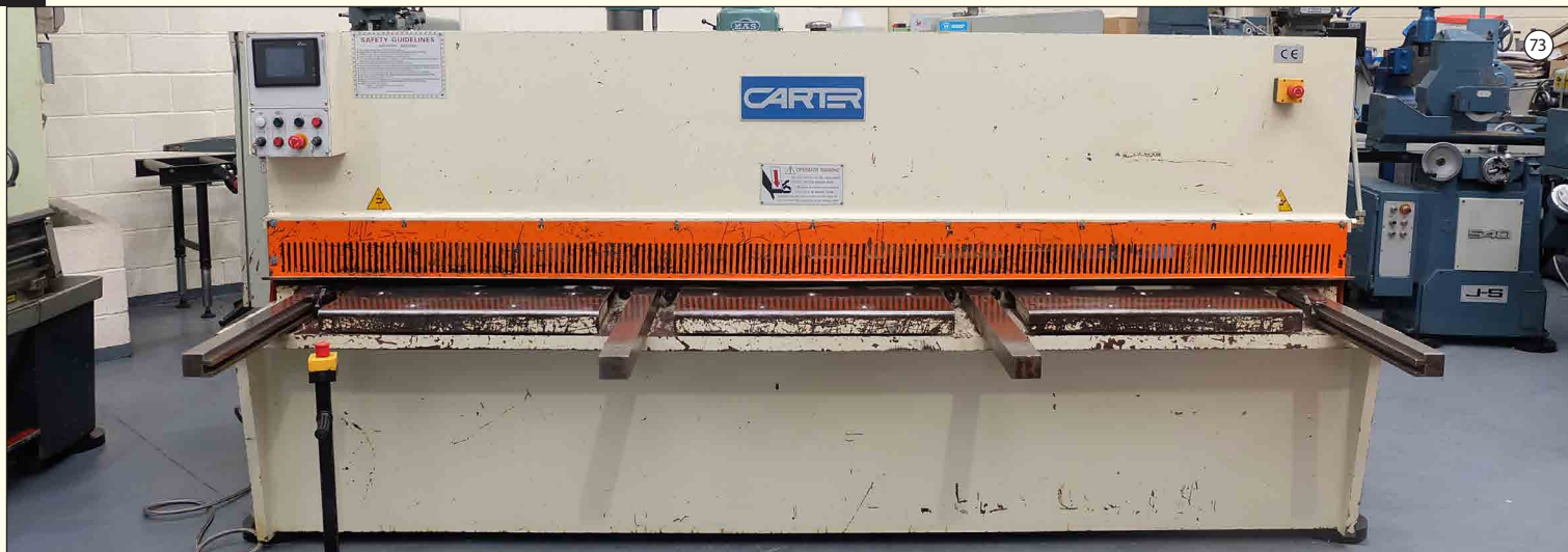
CARTER MODEL QC12K-6x3200: Hydraulic Power Guillotine. Capacity 3200mm x 6mm. N C Power Back Gauge 800mm. Front Supports & Rear Hydraulic Lifting Sheet Support. Motor Size 7.5KW/ Year 2007.
