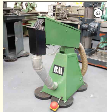
MULTITOOL MODEL BM7552: Pedestal Linisher. Belt Width 75mm. 3 Phase Motor. £795
