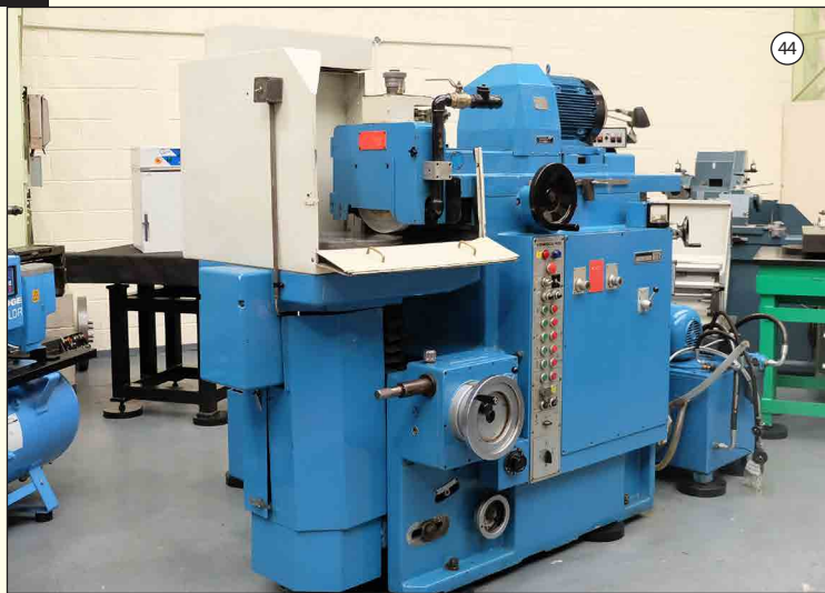
ABWOOD Type RG1: Tool Room Ring Grinder. Table Size 500mm. Magnetic Chuck 500mm. Max Spindle Speed 2870rpm.
