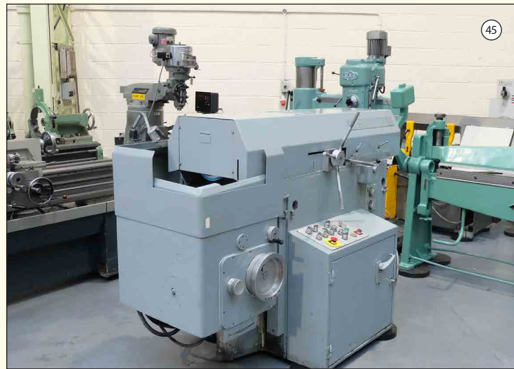
SNOW Model RT 400: Ring Grinder. Table Size 400mm Diameter. Max Height Under Wheel 200mm. Grinding Wheel Size 350mm x 25mm. Table Speeds 70-250rpm. With 400mm Electro Mag Chuck.
