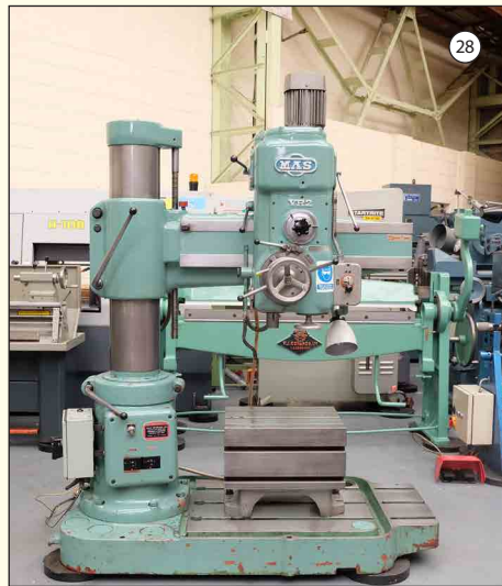
MAS TYPE VR2: 3' Radial Arm Drill. Speeds 90-4500rpm. Spindle Taper No. 3 Morse. Drilling Depth 8 1/4". Power Feed to Spindle. Box Table 20" x 16" x 16".
