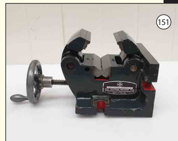
ELLIOTT: Self Centering Pipe Vice. Width of Jaws 4 3 / 8 ". Opening of Jaws 3 1 / 8 ". £425
