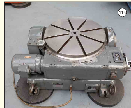
HERBERT LINDLER: Precision Tool Room Motorised Rotary Table. 440mm Diamater. Motor 0-15kw/110 Volt.
