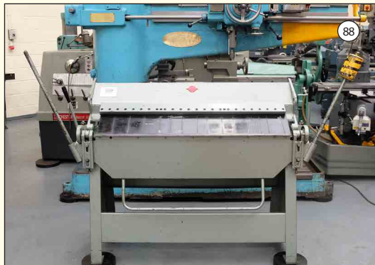
SELSON BESCO Model B&P 416: Manual Box & Pan Folding Machine. Capacity 1270mm x 1.5mm or 50" x 16swg. 16 Pieces of Tooling: Total Length 1270mm. £1,650
