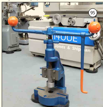
SWEENEY BLOCKSIDGE No5: Fly Press. Throat 5". Daylight 7". £575
