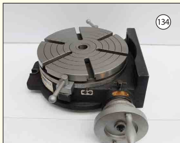
VERTEX: TEE Slotted Rotary Table. 12" Diameter.
