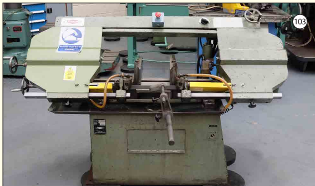
JAESPA W260: Horizontal Bandsaw. Capacity Round Bar 260mm.
