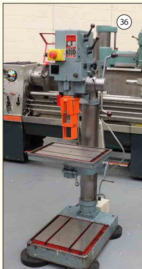
MEDDINGS S32M: Geared Head Pillar Drill. Speeds 70-1220rpm. No.3 MT. Cap 32mm. Power Feed. £1,850
