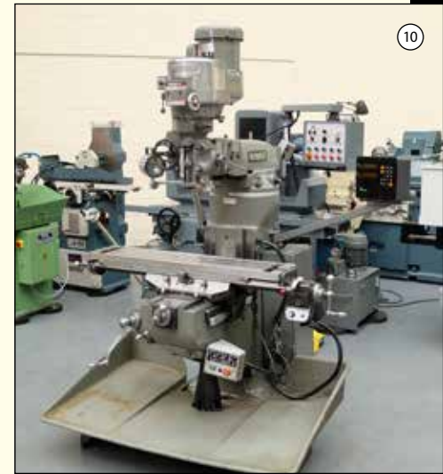
BRIDGEPORT Type BR2J2: Varispeed Turret Milling Machine. Spindle Taper R8. Spindle Speeds 50-3250rpm. Table 42" x 9". Power Feed to Table. 2 Axis DRO. £5,250
