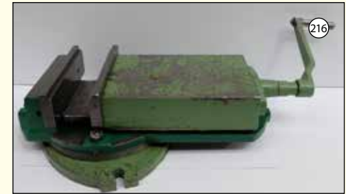
SWIVELLING MACHINE VICE: Max Jaw Opening 250mm. Jaw Width 300mm. Jaw Height 90mm.
