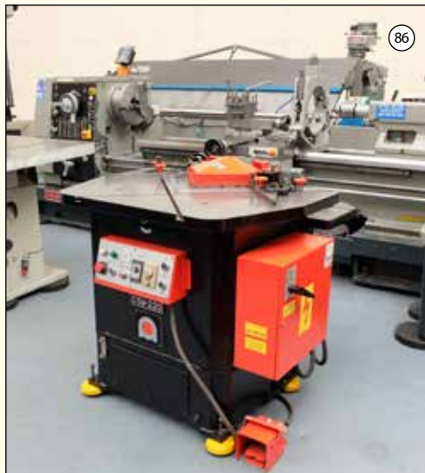
AMADA Type CSW-220: Hydraulic Sheet Metal Corner Notcher. Cap 200mm x 2mm Mild Steel, 200mm x 1.5mm Stainless. With Rear Square Notcher: 100mm x 50mm. £2,950
