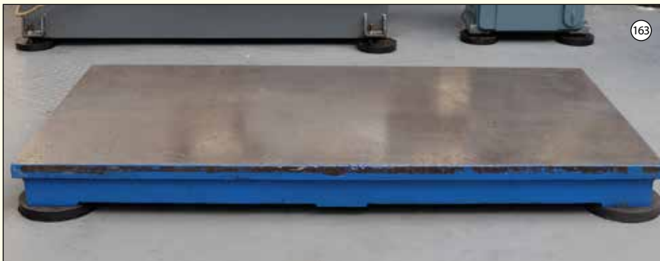
CAST IRON: Surface/Welding Floor Plate. Size 7' 6" x 45".
