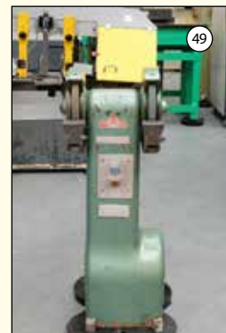
RJH BISON: Double Ended Pedestal Grinder. Wheel Size 250 x 25 x 20mm. £425
