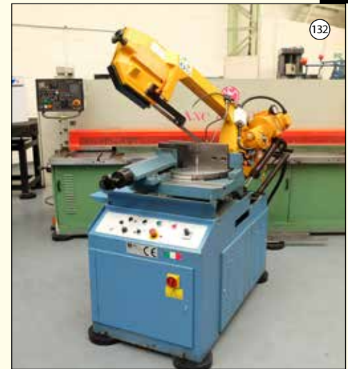
ANBAS Type ZAC 330 VA: Double Mitre Horizontal Bandsaw. Hydraulic Assisted Vice. Power Rise & Fall. Max Diameter 330mm.
