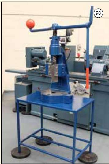
NORTON No. 65: Fly Press on Steel Stand. Throat 6". Daylight 9".
