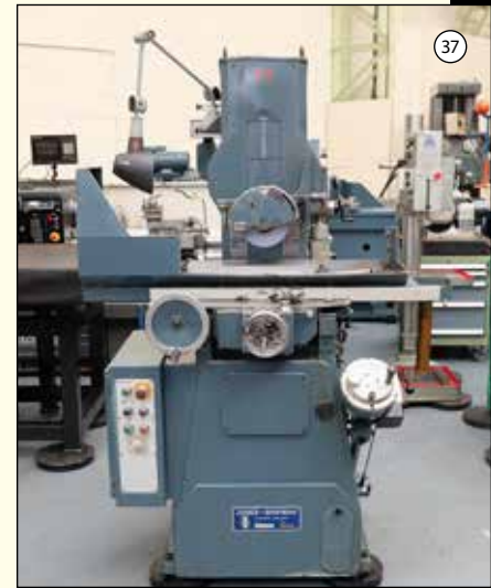
JONES & SHIPMAN 540L: Tool Room Surface Grinder. Capacity 18" x 6". Height Under Wheel 16". Long Column. Power Rise & Fall. £6,950
