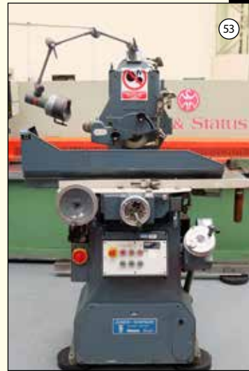
JONES & SHIPMAN 540P: Surface Grinder. Capacity 18" x 6". Power Rise & Fall. Magnetic Chuck 14" x 6". £5,250
