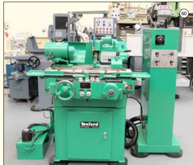
MYFORD MG12-HA: Hydraulic Cylindrical Grinder. Maximum Grinding Capacity 3" Diameter. Swing Over Table 5". Max Table Travel 13 3 / 4 ". Capacity Between Centres 12".
