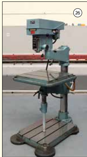
MIDDINGS A10: Articulated Arm Drill. 2 MT. Throat 24". Speeds 80- 4000rpm. Rise & Fall Table. £1,950
