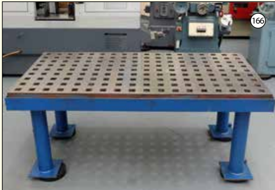
BLACKSMITHS: Cast Iron Surface Table. Size 6' x 6'6" x 5" Thickness. Complete with approx 160 Square Work Holes.
