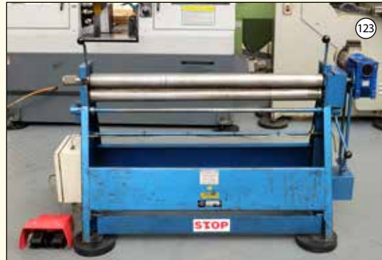
WALTON Type OMR 3: Initial Pinch Powered Sheet Metal Bending Rolls. Length of Rolls 50". Diameter of Rolls 3".
