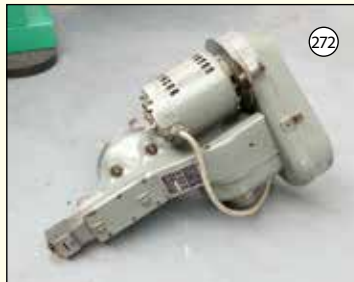
BRIDGEPORT: Slotting & Shaping Head. Stroke: \frac{1}{8} - 4". 6 Speeds: 60 - 350 s/min. £1,250
