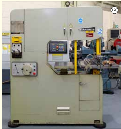
STARTRITE Type 316H: Toolroom Vertical Bandsaw. Throat 36". Daylight 16". Power Cross to Table. Variable Speed. Blade Welding Attachment. £2,750
