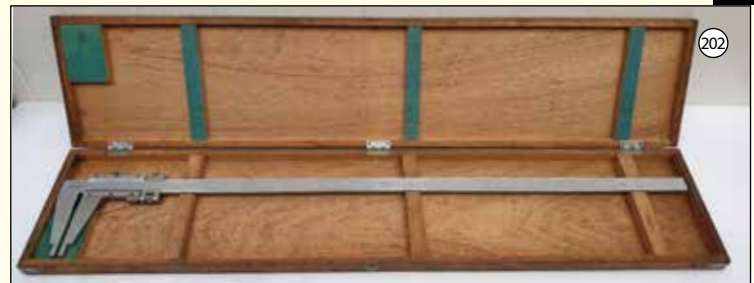
MITUTOYO: Vernier Caliper. Stainless Steel. 1000mm Capacity.
