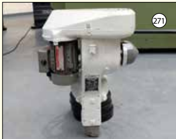
BRIDGEPORT: Slotting & Shaping Head. Stroke: \frac{1}{8} - 4" 6 Speeds: 60 - 350 s/min. £1,250
