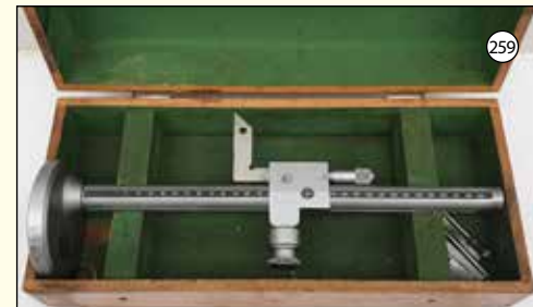
ALL PRECISION ENGINEERING Ltd: Microball Vernier Height Gauge. 300mm Capacity.
