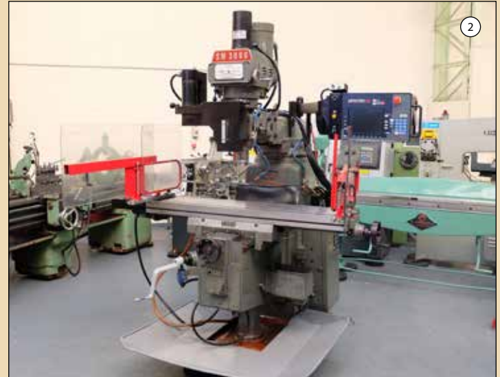
XYZ SM3000: 3 Axis CNC Turret Milling Machine. Prototrak SM Control. Table 1370mm x 300mm. Spindle Taper 40 int. Speeds 70-3600rpm. Power Draw Bar.
