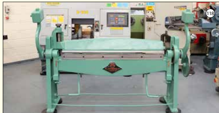
EDWARDS HIGH LIFT: Manual Sheet Metal Folding Machine. Capacity 60" x 14SWG.
