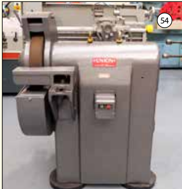
UNION: HD Single Wheel Fetting Grinder. Maximum Wheel Diameter 16" x 3". £950
