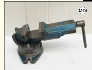
TILTING & SWIVELING MACHINE VICE: Jaw Opening 4 1/4". Jaw Width 5".
