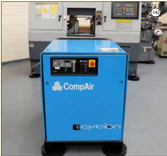
COMPAIR Model Cyclon 111: Rotary Air Compressor. Max Pressure 7.5 Bar. Flow Rate 1.77m 3 /Min. Motor Power 13.59kw. £1,750
