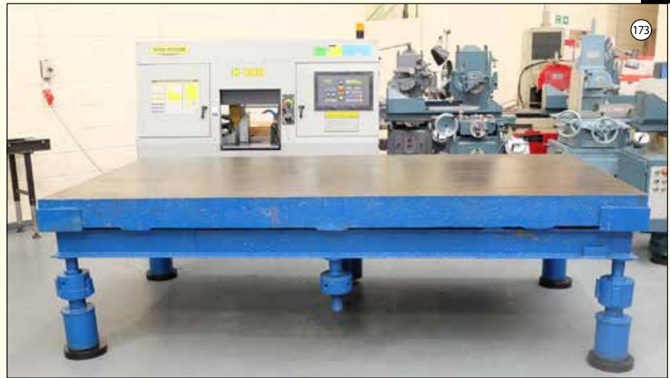
WELDING TABLE: Size 120" x 61" x 35" High. Thickness 6 1/2". Fitted to RSJ's.
