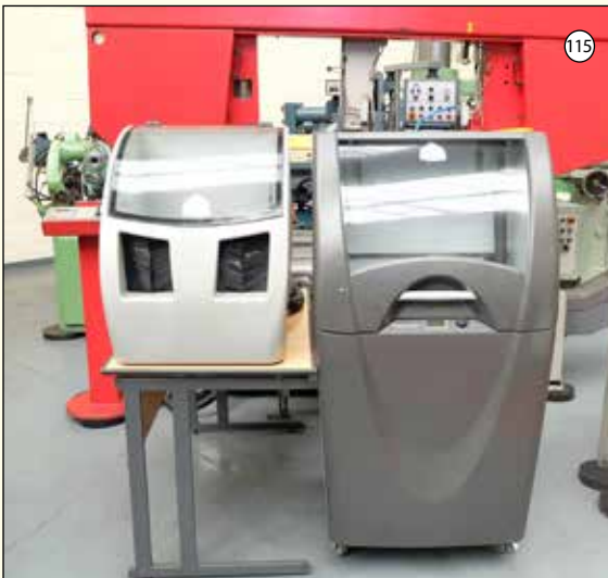
3D SYSTEMS PROJECT 260C: 3D Colour Printer. Max Build Size 236 x 185 x 127mm. Min. Feature Size 0.4mm. Print Heads 2 x CJP. Layer Thickness 0.1mm.
