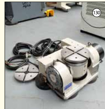
JONES & SHIPMAN: 4th AXIS Tilting Rotary Table. Size 260mm. Height 310mm. 360 Deg Rotation. Type 8414-009DC/306.
