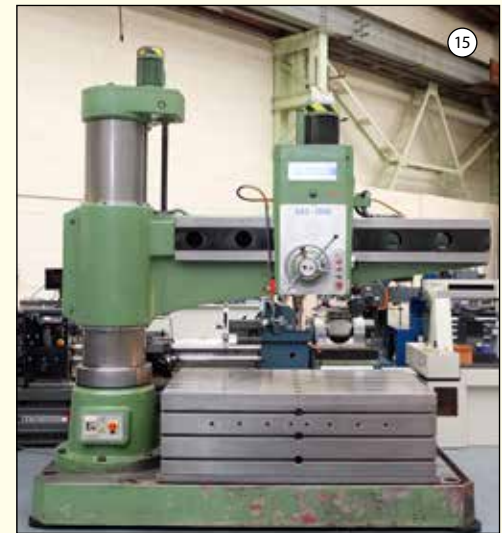
KITCHEN & WALKER Type G63 - 2000: Radial Arm Drill. Radius 2000mm. Spindle 5 MT (3"). Spindle Speeds 20 - 1600rpm. Box Table Size 70" x 43" x 23". £14,250
