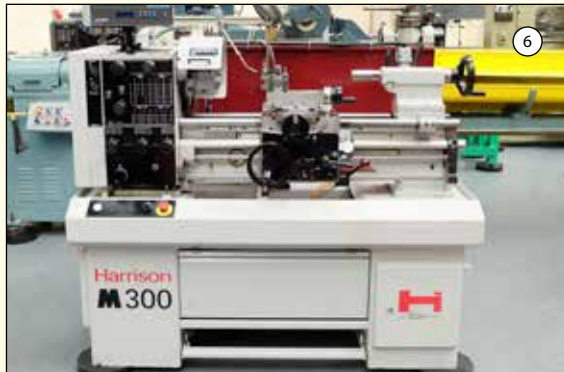
HARRISON M300: Gap Bed Centre Lathe. Swing Over Bed 330mm. Spindle Bore 40mm. Between Centres 635mm. Metric Lead Screw & Dials. Speeds 40 - 2500rpm. 3 & 4 Jaw Chucks. 3 Point Steady. DRO. £11,250
