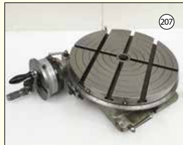
TEE SLOTTED TOTARY TABLE: With Dividing. 380mm Diamater. 120mm Height.
