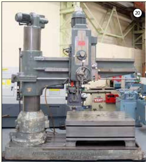
KITCHEN & WALKER Type E3: Radial Arm Drill. Radius 6'. Drilling Capacity 1/4" - 3". Spindle 5MT (3"). Speeds 12 - 1000rpm. Table 50" x 36" x 20" High. DC Brake. Coolant System. £5,750
