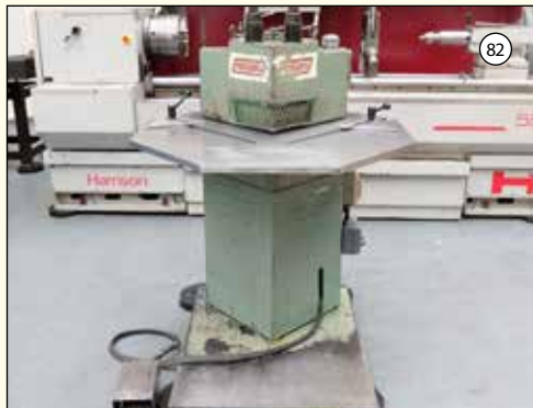
PIERCEALL: Sheet Metal Corner Notcher. Capacity: 200mm x 200mm x 3mm Mild Steel. Table Size 42" x 27". Foot Control.
