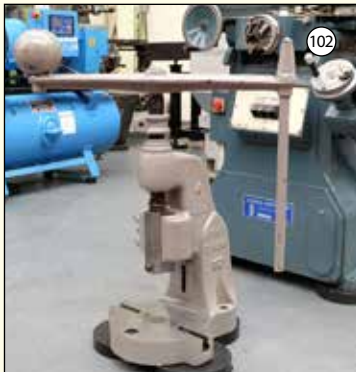
DENBIGH No4: Fly Press. Throat 4 1/2". Daylight 7 1/2". Approx Tonnage 4.
