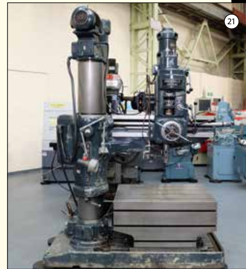
ARCHDALE: 3'6" Radial Arm Drill. 2" Drilling Capacity. Spindle Taper No.4 Morse. Box Table 40" x 30" x 20" High. £3,750
