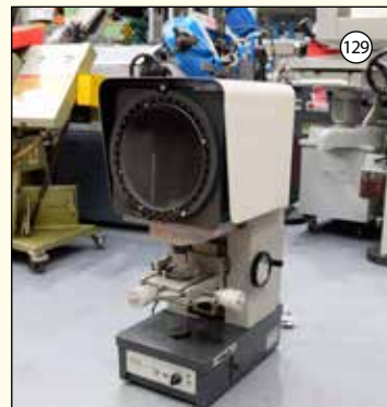
MITUTOYO PJ250C: Shadowgraph. Metric Table Dials: Accuracy 0.005mm. X & Y Axis 0-25mm Travel.
