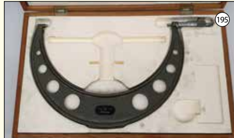
MITUTOYO: Outside Micrometer. Capacity 11" - 12".
