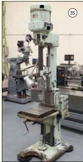
HERBERT: Pedestal Drill. Table 18" x 15". 2 Morse Taper. Speeds 51-2650rpm. £950
