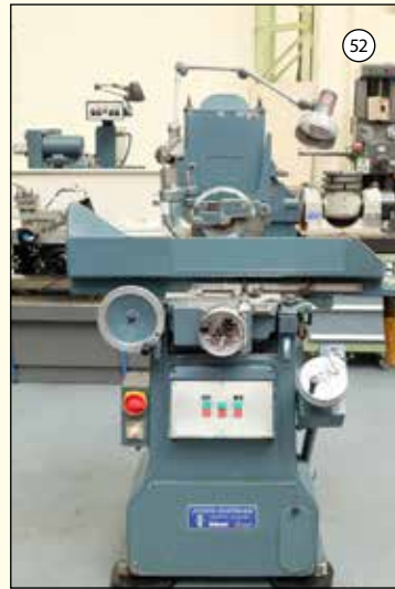
JONES & SHIPMAN 540P: Surface Grinder. Capacity 18" x 6". Power Rise & Fall. Imperial Dials. £3,250
