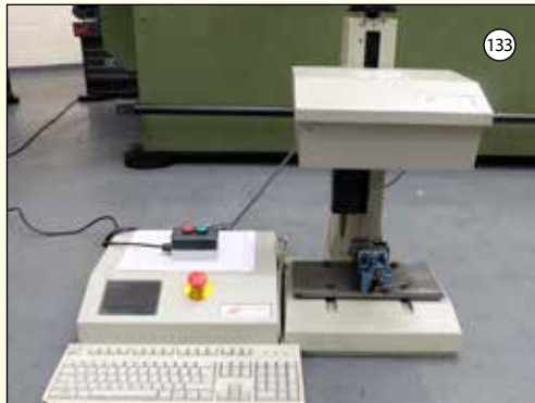
PRYOR MARKTRONIC MULTIDOT 2068: Dot Marking Machine. Variable Force Control. Materials up to 62R. Memory Cap up to 1350 Layouts.
