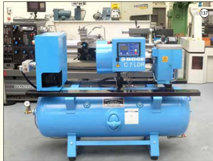
BOGE Type C-7-LDR 270: Rotary Screw Air Compressor. Flow Rate 0.728 m 3 /min. Max Pressure 10 Bar. Motor Speed 3000rpm. Motor Power 5.5kw. CFM 25. BWB 270 ltr Air Receiver Year 2013.
