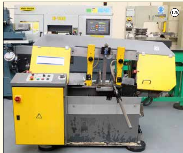
BEK-MAK BMSY 320: Horizontal Metal Cutting Bandsaw. Capacity Round 300mm.
