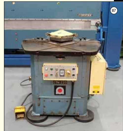
AMADA Type CSW-220: Hydraulic Sheet Metal Corner Notcher. Cap 200mm x 2mm Mild Steel, 200mm x 1.5mm Stainless. With Rear Square Notcher: 100mm x 50mm. £1,950
