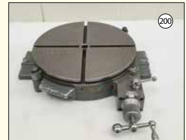
TAYLOR - HOBSON: Tee Slotted Rotary Table. 12" Diameter. £525
