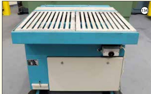
BECK Type BE-TL 100: Vacuum Bench. Work Surface 1000mm x 700mm.
