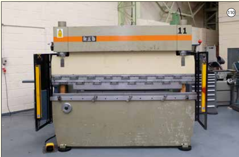
K&B: Down Stroke Hydraulic Press Brake. Capacity 2500mm x 50 Ton. Distance Between Side Frames 2120mm. Manual Back Gauge. Light Guards. Foot Control.
