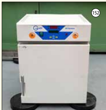
FRATELLI GALLI Model G-2100: Oven. Appature 300mm x 300mm x 250mm Deep. Max Temp 300Deg, Single Phase. £500
