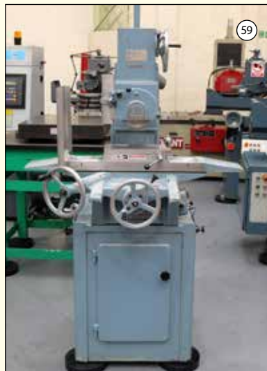
EXE: Toolroom Precision Manual Surface Grinder. Table Capacity 12" x 6". Fitted to EXE Pedestal Cabinet.
