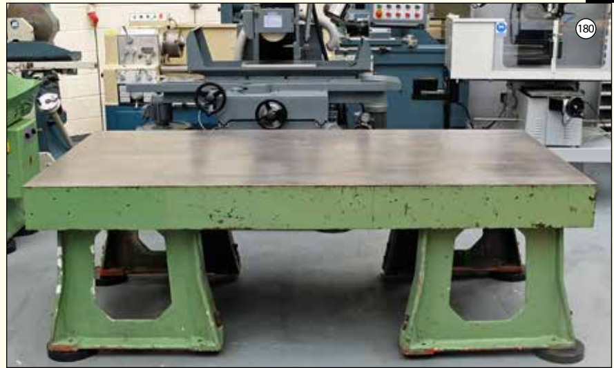
CAST IRON: Surface Table. Size 8" x 4'. Overall Height 31".
