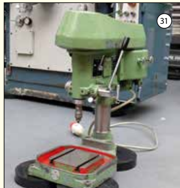
FLOTT Type TB6: High Speed Bench Drill. Throat 6 1/2". Capacity 1/4". Tee Slotted Base 12" x 9". Speeds 450 - 9000rpm. £550
