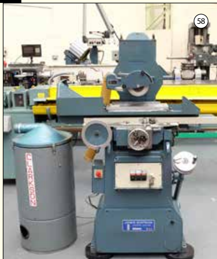
JONES & SHIPMAN 540: Surface Grinder. Capacity 18" x 6". With Dust Extractor.
