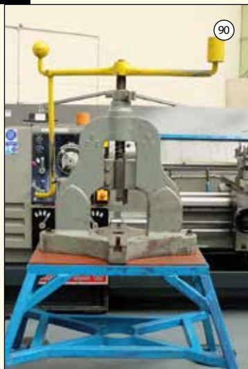
DENBIGH 6 DS: Double Sided Fly Press. 12" Between Sides. 9" Daylight. Centre to Side 6". Bar Press Holes. £750
