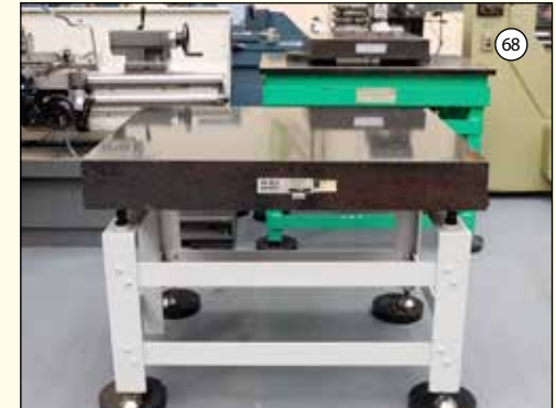
WBJ: Granite Surface Table. Grade 1. Surface Size 48" x 36". Thickness 6". On Leveling Stand.
