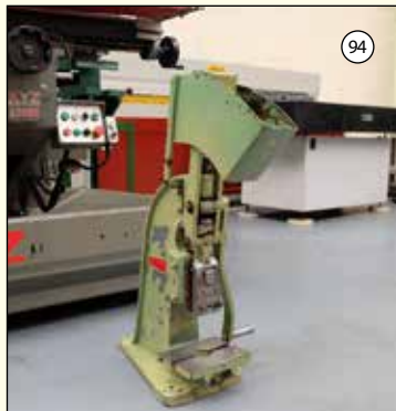
STANEL: Bench Type Toggle Press. Daylight 5 1/4". Throat 3 1/4". Stroke 1 1/8". Table Size 7 3/4" x 6". £125
