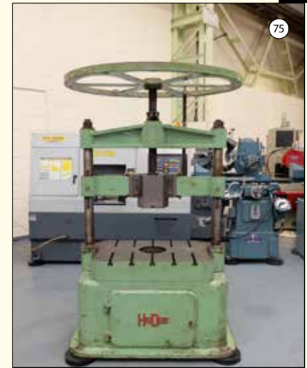
HAZELWOOD & DENT: Model 36 SCP2 Heavy Duty Fly Press. 36" Between Columns. 20" Daylight. Table Size 36" x 24". 7" Hole in Table. £1,750
