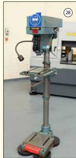
MIDDINGS MF4/3: Pillar Drill. No. 2 MT. Speeds 80-4000rpm. Table Size 11" X 10" £1,250
