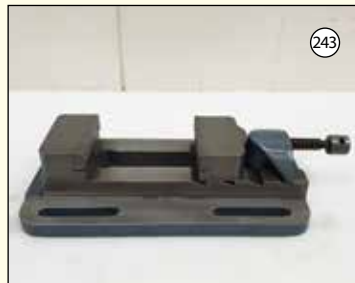
JONES & SHIPMAN: Rack Vice. Max Opening 5". Jaw Width 4". Jaw Depth 1 1/2".
