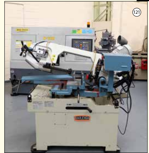
BAILIGH Type BS350M: Horizontal Metal Cutting Bandsaw. Capacity Round 240mm. £2,950
