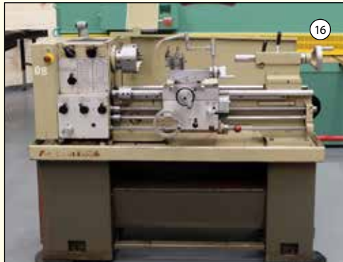
HARRISON M300: Gap Bed Centre Lathe. Swing Over Bed 300mm. Swing In Gap 430mm. Between Centres 700mm. Speeds 40-2500rpm. £5,250
