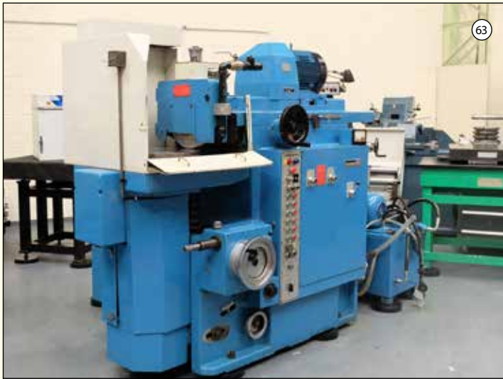
ABWOOD Type RG1: Tool Room Ring Grinder. Table Size 500mm. Magnetic Chuck 500mm. Max Spindle Speed 2870rpm.
