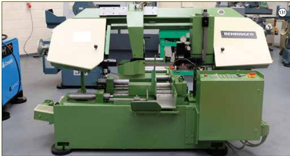
BEHRINGER Type HBP-320A: Automatic Horizontal Bandsaw. Capacity 320mm. Blade Speed 15-180 m/min. Blade Size 4850 x 34 x 1.1mm.
