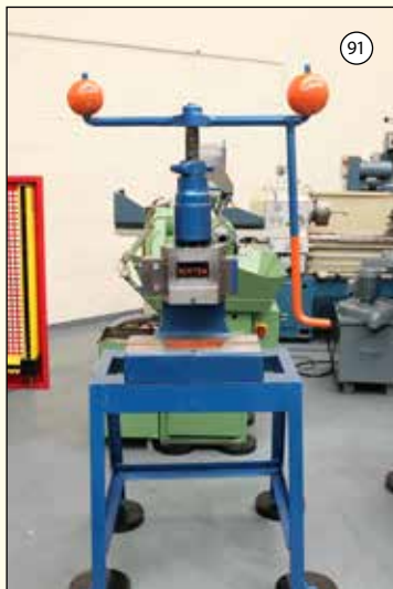
NORTON No. 4GP: Fly Press On Stand. Table Size 19" x 10". Throat 5". Daylight 7". Table Throughhole 8" x 3". £950
