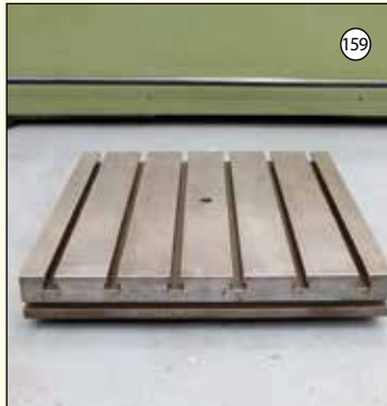
TEE SLOTTED: Cast Iron Plate. 6 x Tee Slots. Size 36" x 36" x 5".
