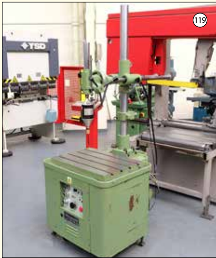
ELECTRO ARC 2DBT: Tap & Bolt Disintegrator. Table 26" x 18", Swivel Head 90°. Movement: Quill 26" x 8", Vertical 26" x 30", Horizontal 26" x 26". With 28V LBH Head. £2,250
