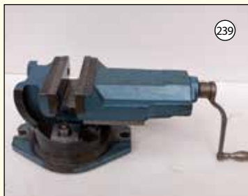
Milling Machine Vice: Tilting & Swiveling.
