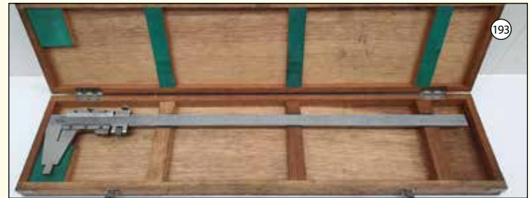
MITUTOYO: Vernier Caliper. Capacity 600mm.
