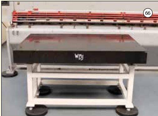
WBJ: Granite Surface Table. Surface Size 1500mm x 1000mm. On Leveling Stand.
