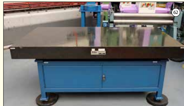
WBJ: Granite Surface Table on Stand with Cupboard. Surface Size 2000mm x 1000mm. Grade 0. With 8 Clamp Studs.
