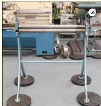
EDWARDS: Initial Pinch Sheet Metal Rolls. Length of Rolls 30". Diameter of Rolls 1 3/4".
