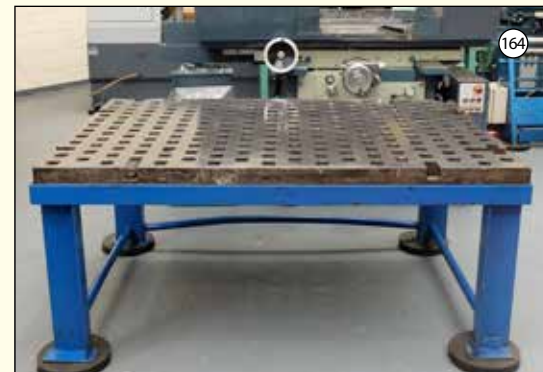
BLACKSMITHS: Cast Iron Surface Table. Size 6' x 4' x 5" Thickness. Complete with approx 200 Square Work Holes.
