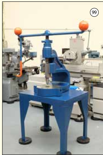
NORTON No 8A: Fly Press on Stand. Throat 14 1/2". Daylight 8 1/2".
