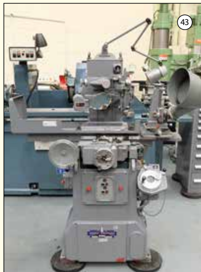
JONES & SHIPMAN 540AP: Tool Room Surface Grinder. Cap 18" x 6". Imperial Dials. Power Rise & Fall. Auto Down Feed. Optidress & Scope. £4,750
