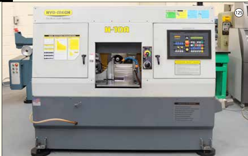
HYD-MECH H-10A: Automatic Horizontal Band Saw. Capacity @ 90 Degrees Rectangular 10" x 10". Capacity Round 10". High Speed Shuttle Feed Indexing up to 24". Blade Size 1 1/4". Main Motor 5hp. With Chip Conveyor. Year 2012.
