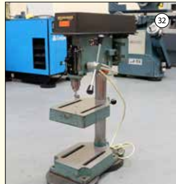
MIDDINGS DB: Bench Drill. Spindle 1/2". Speeds 500-4000rpm. Single Phase. £325
