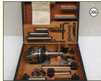
KURODA UFB-4: Boring & Facing Head. 40 Int Taper. 5 \frac{1}{8} " Drawbar Thread £1,450
