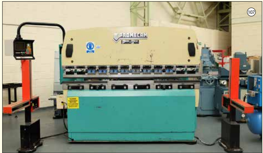
PROMECAM Type RG-65-25: Hydraulic Upstroke Press Brake. Capacity 2500mm x 65 Ton. Power Back Gauge. New Autobend 7 Fitted in 2010. Light Guards & Tooling.
