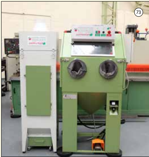
LAMPUGNANI LC-05: Sand Blasting Machine. Max Pressure 8 Bar. Internal Dimensions 800 x 600 x 700mm. Extraction Unit. Dust Collection Cabinet. Work Hours 211. £2,950
