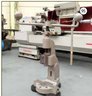
SWEENEY BLOCKSIDGE Type 6T: Fly Press. Throat 5". Daylight 12". £525
