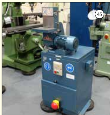
RJH: Vertical Bandfacer on Dust Extractor. Belt Size 100mm x 915mm. Motor 0.75kw. 3 Phase 415V. £1,750
