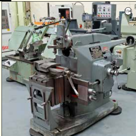
ELLIOTT 18" MAJOR: Shaping & Slotting Machine. Capacity 18". Strokes 12-110/min. 6 Speeds 4-125 fpm. Feeds 0 - 0.060. Table Size 18" x 12". Swivel Vice 9 1/4 "
