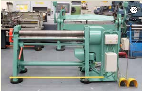
F.J. EDWARDS: Initial Pinch Power Rolls. Length of Rolls 48". Diameter of Rolls 4".
