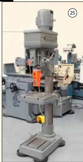
MIDDINGS: Heavy Duty Pillar Drill. Table 17" x 15". Speeds 90-1570rpm. Throat 11". 3MT. Power Feed. £2,950
