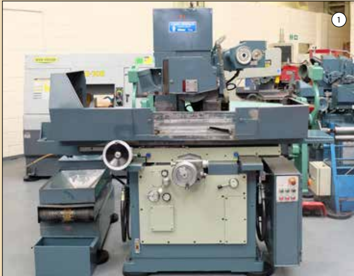
JONES & SHIPMAN Type 1415: Toolroom Surface Grinder. Capacity 27" x 12". Distance Under New Wheel 11 3 / 4 ". Power Rise & Fall to Wheelhead. With Magnetic Chuck & Coolant Tank.
