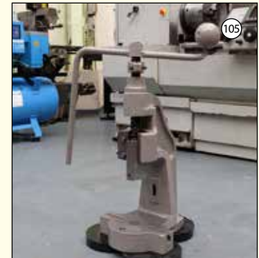
NORTON Type 2L: Fly Press. Throat 5". Daylight 10".
