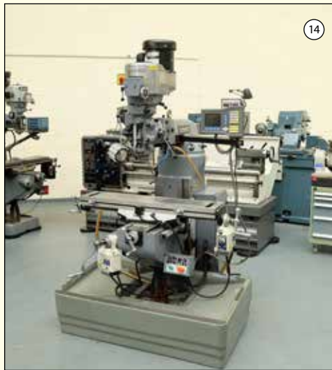
BRIDGEPORT BR2J2: Variable Speed Turret Milling Machine. Table 42" x 9". BE30 Quick Change Spindle. Speeds Up To 3250rpm. 3 Axis DRO. Remanufactured 2009. £7,950
