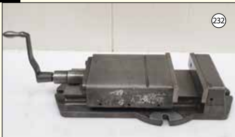
MACHINE VICE: Max Jaw Opening 205mm. Jaw Width 210mm. Jaw Depth 55mm.
