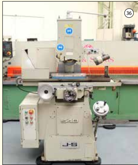
JONES & SHIPMAN 540L: Tool Room Surface Grinder. Capacity 18" x 6". Height Under Wheel 16". Long Column. Power Rise & Fall. £6,950
