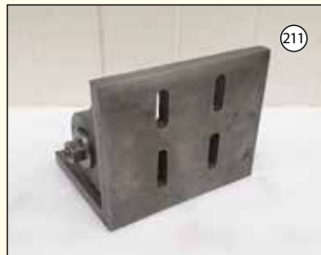
UNION: Adjustable Angle Plate. 7" x 10". 90 Degrees Rotation. Base 8" x 10". £275
