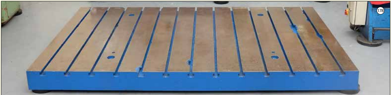
TEE SLOTTED: Floor Plate. Size 10' x 6' x 8" Thickness. 13 x Tee Slots.
