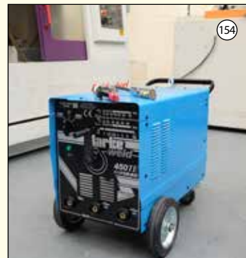
CLARKE 450TE TURBO: Arc Welding Machine. Cap. 40-400am. Accepts Electrodes 1.6-6mm. Power Input 230/400v. £425
