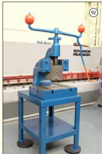
SWEENEY & BLOCKSIDGE: Deep Throat Fly Press. Tee Slotted Table 25" x 19". Daylight 9 3/4". Throat Depth 15". Stroke 6". £1,450
