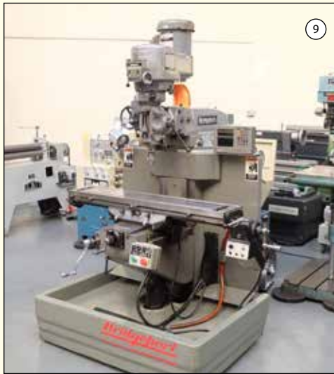
BRIDGEPORT Type BR2J2: Varispeed Turret Milling Machine. Spindle Taper R8. Spindle Speeds 50-3250rpm. Table 48" x 9". Power Feed to Table. 2 Axis DRO. £9,250
