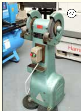
RJH Model M: Double Ended Pedestal Tool Grinder. Wheel Size 10" x 1". £275
