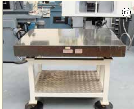
WBJ: Granite Surface Table. Surface Size 4' x 3'. Grade 1. On Leveling Stand.
