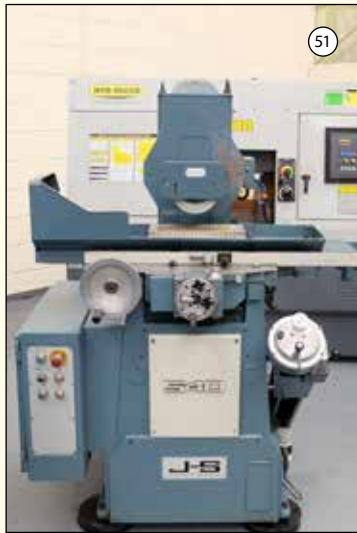
JONES & SHIPMAN 540P: Surface Grinder. Capacity 18" x 6". Power Rise & Fall. Power Rise & Fall to Wheel Head. £7,950
