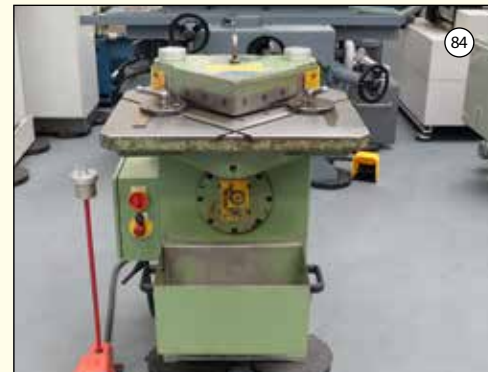
BOSCHERT PN4: Sheet Metal Corner Notcher. Capacity: 225mm x 225mm x 4mm Mild Steel. 225mm x 225mm x 3mm Stainless Steel.
