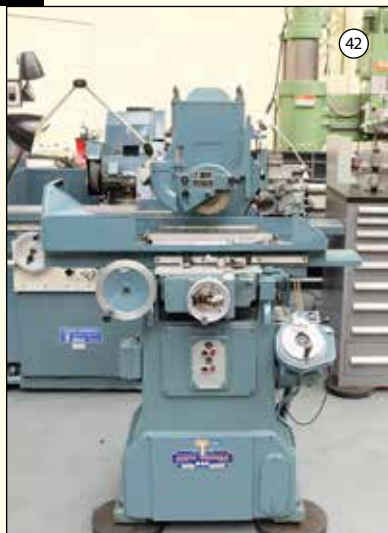
JONES & SHIPMAN 540AP: Tool Room Surface Grinder. Cap 18" x 6". Imperial Dials. Power Rise & Fall. Auto Down Feed. £4,950
