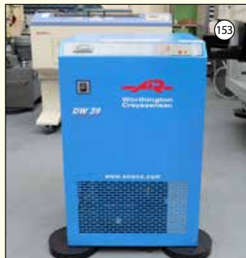
WORTHINGTON CREYSSENSAC Type DW39: Water Chiller. Refrigerment R404A. Power 1KW. Single Phase 230v. £2,750
