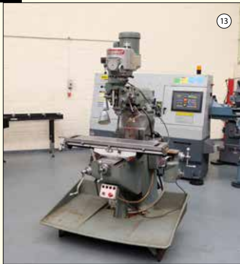
BRIDGEPORT Type BR2J2: Turret Milling Machine. Spindle Taper R8. Variable Speed. Table 42" x 9". Speeds 50 - 3750rpm. Swivel & Tilt Head. Power Feed to Table. £2,750
