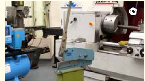
KINGSLAND TYPE A94: Hand Cropper. Plate Size 250mm x 3mm. Round Bar 12mm. Flat Bar 25mm x 5mm.
