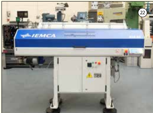
IEMCA TYPE 16 MODEL 80: Short Bar Magazine Bar Feeder. Year 2008.
