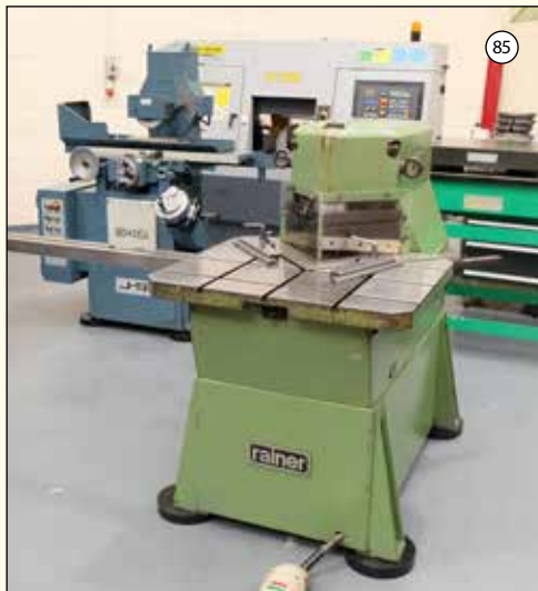
RAINER Type 300/3: Sheet Metal Hydraulic Corner Notcher. Capacity 300mm x 3mm. Table Size 680mm x 840mm. Foot Control. £2,950
