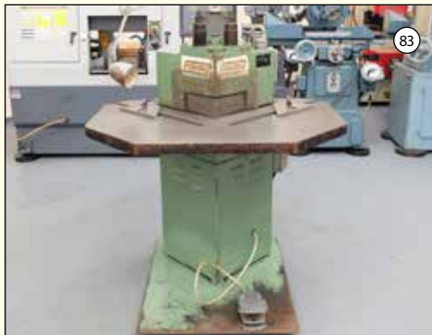
PIERCEALL: Sheet Metal Corner Notcher. Capacity: 200mm x 200mm x 3mm . Table Size 42" x 27". Foot Control.
