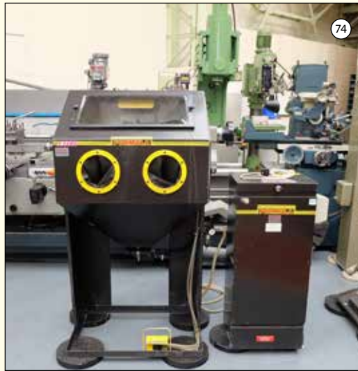
GUYSON Formula F1400: Shot Blast System. Internal Dimensions 800mm x 500mm x 500mm High. With Guyson F21 DC Single Phase Dust Extractor. £2,250
