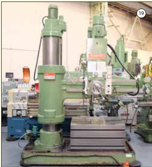
ASQUITH Type OD1 MK2 14/54: Radial Arm Drill. Radius 4'6". Spindle 4 MT (2"). Speeds 40-2040rpm. Power Locking. Box Table 40" x 30" x 20". DC Telescopic Safety Brake. £9,950
