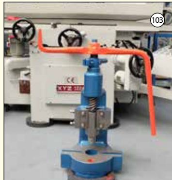
SWEENEY & BLOCKSIDE: Fly Press. Daylight 6 1/4". Throat 4 1/2". Stroke 4 1/4".
