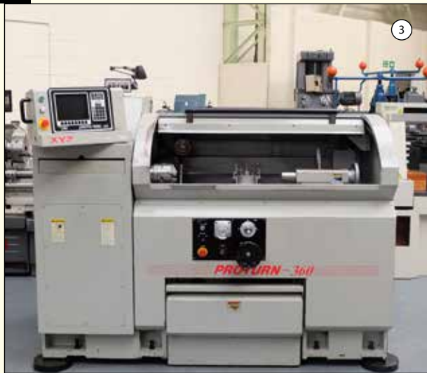
XYZ Protorn 360: CNC Centre Lathe Prototrak LX3 Control. Swing Over Bed 380mm. Swing Over Cross Slide 240mm. Between Centres 750mm. Spindle Bore 45mm. Spindle Speeds 145-4000rpm. Constant Surface Speed. £8,950
