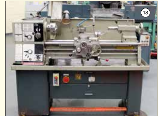
COLCHESTER BANTAM 2000: Centre Lathe. Swing Over Bed 13". Between Centres 30". Spindle Bore 1 3 / 8 " - Spindle Speeds 40-2000rpm, £3,950
