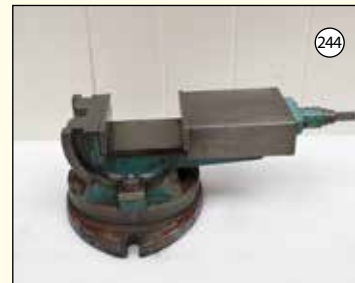
ABWOOD: Tilting, Turning Machine Vice. Max Jaw Opening 5". Jaw Width 6 1/4".
