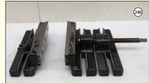
EXTENDABLE CLAMP VICE: Jaw Depth 105mm. Jaw Width 325mm. Extends 180mm
