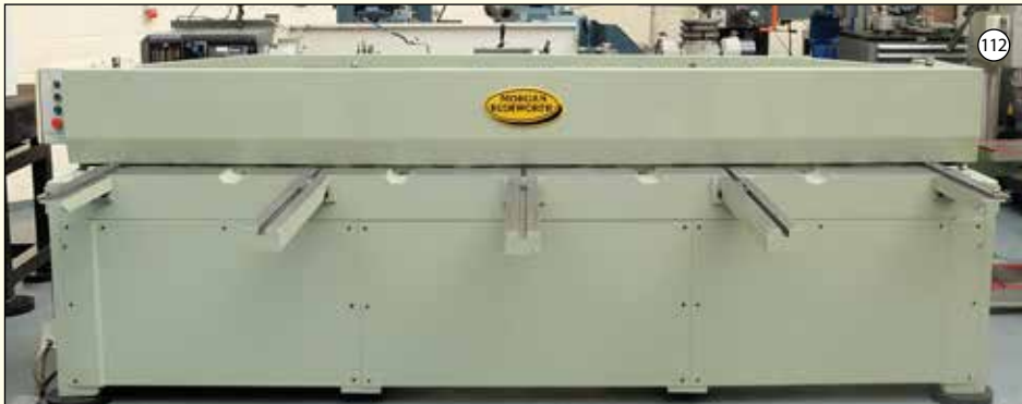
MORGAN RUSHWORTH: Direct Drive Power Sheet Metal Guillotine. Capacity 3000mm x 3mm. Manual Back Gauge.
