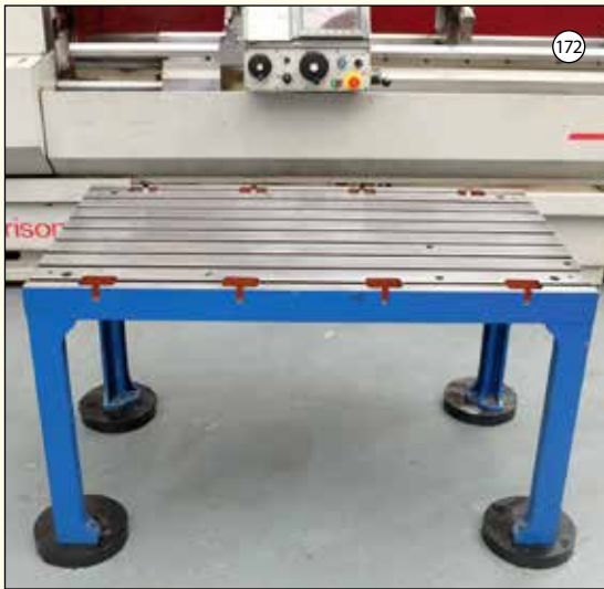
TEE SLOTTED: Light Duty Work Table. Size 48" x 27". 9 Tee Slots.
