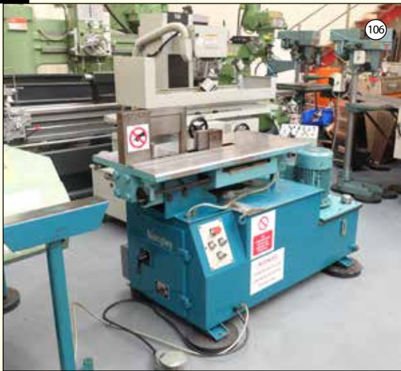
LANGLEY MODEL 800: Horizontal Bending Machine. Table Size 47" x 22". Foot Control. Horizontal Travel 300mm.
