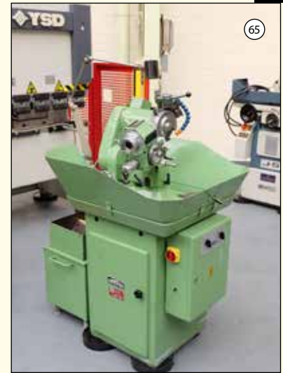
CHRISTEN 1-32/100A: Drill Grinding Machine. Capacity 1 - 32mm. Max Step Length 50mm. Point Angle 60-180 Deg.
