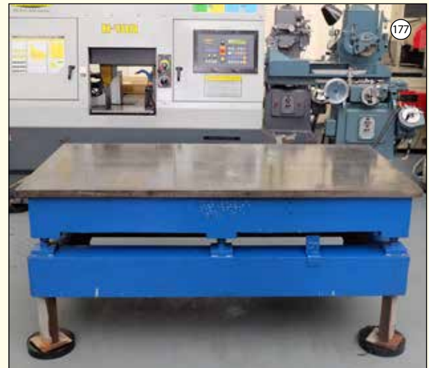
WINDLEY BROTHERS: Cast Iron Surface / Welding Table. Size 6' x 3' x 32" High Fitted to Steel Stand.
