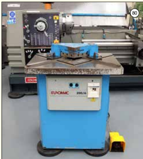
EUROMAC Type 200/6: Hydraulic Sheet Metal Corner Notcher. Capacity 200mm x 6mm (8" x 1/4").
