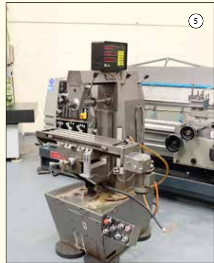
VICEROY AEW: Horizontal Milling Machine. Table 35" x 8". Power Feed in X Axis. Spindle Taper 30 ISO. 2 Axis DRO. £1,650
