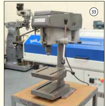
ELLIOTT Model 16: Bench Drill. Cap 13mm. 4 Speeds 460-2900rpm. Drilling Depth 87mm. Table Size 235mm x 235mm. £295
