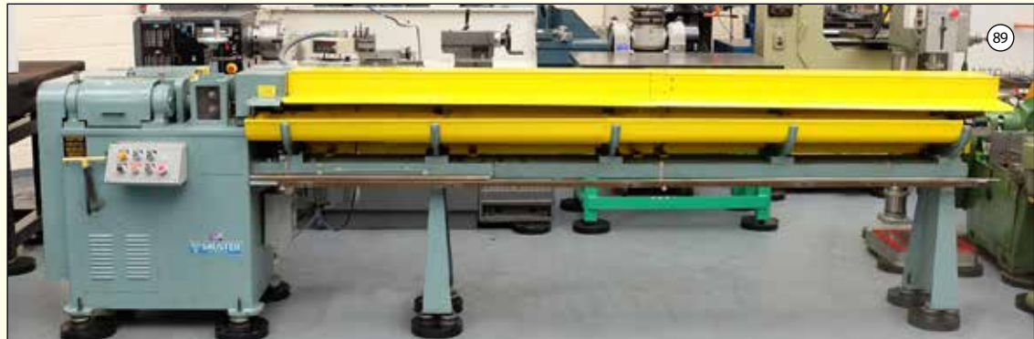
SHUSTER Model 1AVS5: Automatic & Vari-speed Wire Straightening & Cutting Machine. Capacity 1/4" Maximum Diameter. Max Speed 144 Cuts per Min. Variable Speed. Electrically Controlled Cut & Crop. Year 1998. £14,950
