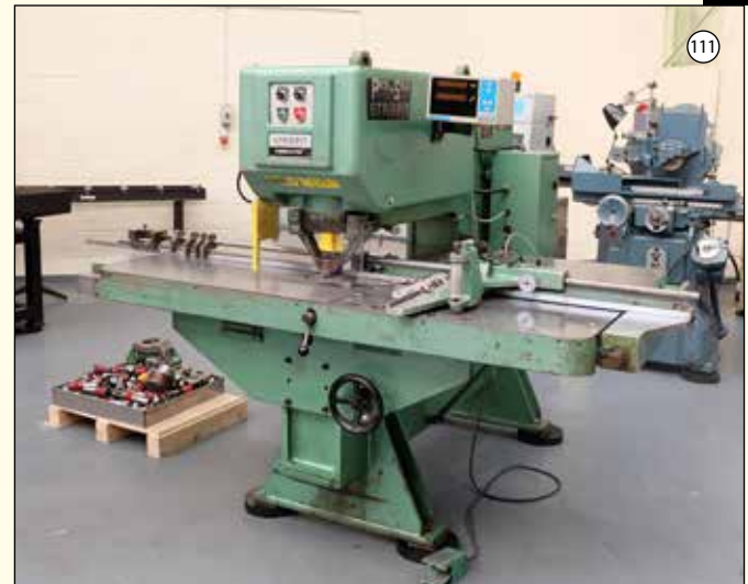
STRIPPIT FABRICATOR: Capacity Punching Table 48" x 40". Copying Table 40" x 32". New Punching Guard. 2 Axis DRO. Selection of Tooling.
