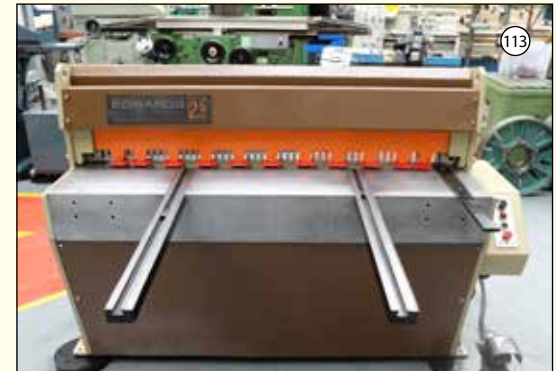
EDWARDS Type DD: Power Guillotine. Capacity 1250mm x 2.5mm. Foot Control. Manual Back Gauge. Front Supports.
