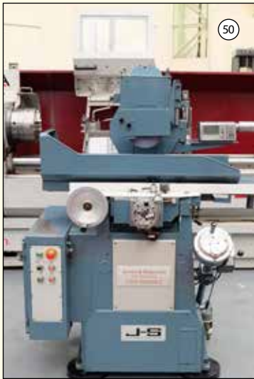
JONES & SHIPMAN 540P: Surface Grinder. Capacity 18" x 6". Power Rise & Fall. DRO on Cross Travel. £6,750
