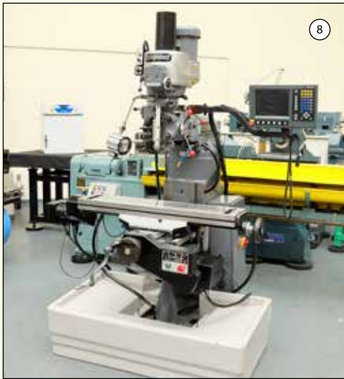
BRIDGEPORT BR2J2: Turret Milling Machine With Acu-Rite PWR 2 Axis CNC System. Table Size 42" x 9". Taper R8. Power Drawbar. 3 Axis DRO. Rebuilt by BMT in 2005. £9,950
