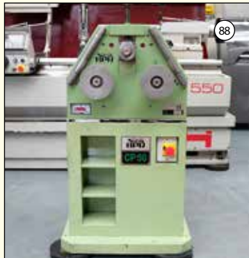
BPR Type CP30: Section Rolls. Two Roll Drive. Shaft Diameter 30mm. Roll Speed 8.5rpm. Capacity Flat 80 x 15mm. £1,450
