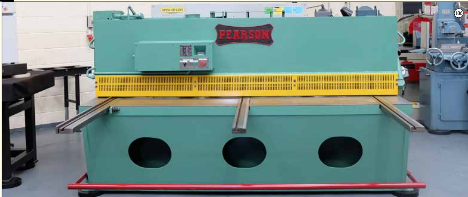
PEARSON TYPE 8 x 25: Hydraulic Guillotine. Capacity 8" x 1/4". Power Back Gauge.
