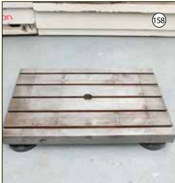
TEE SLOTTED: Machine Table. 5 Tee Slots. Size 48" x 30".
