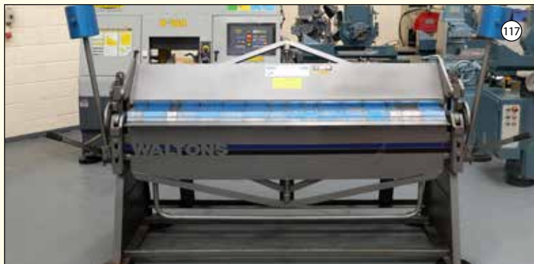
WALTONS TYPE BPFM 80-14: Sheet Metal Box-Pan Manual Folding Machine. 80" x 14SWG.
