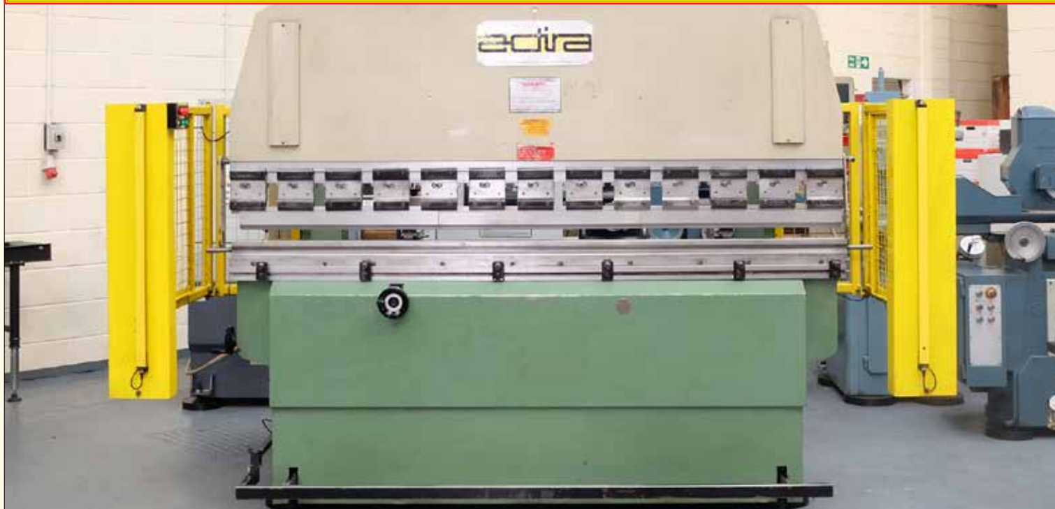
ADIRA Type QHA 8025: Upstroke Hydraulic Press Brake. Capacity 2500mm x 80 Ton. Top & Bottom Tooling. Light Guards. Manual Back Gauge.
