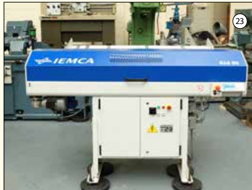
IEMCA TYPE 16 MODEL 80: Short Bar Magazine Bar Feeder. Year 2009.
