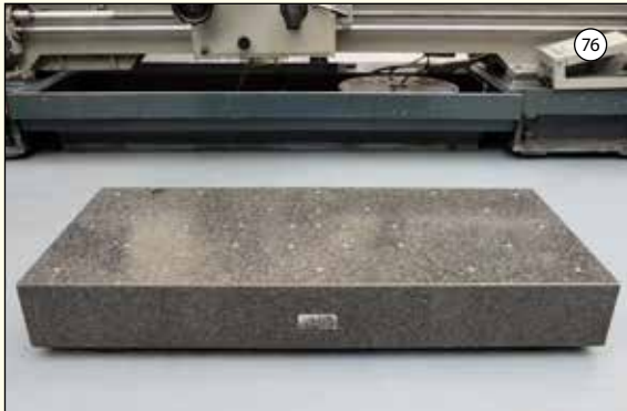
GRANITE TABLE: Surface Size 59" x 26". Thickness 7 1/2". Grade A. With 30 Clamp Studs. £950
