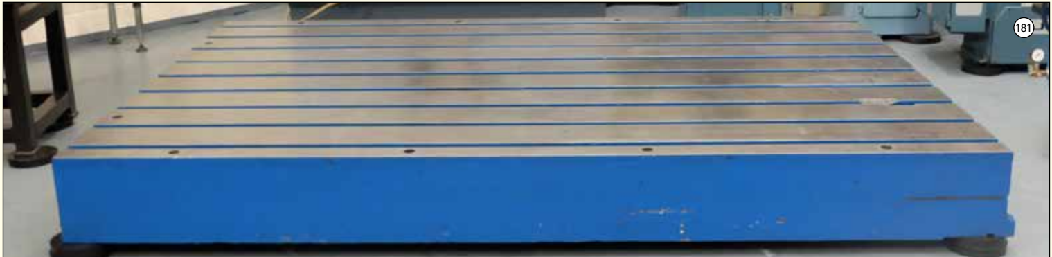
TEE SLOTTED: Cast Iron Floor Plate. Size 10' x 6' 8" x 13 1/2" Thickness.
