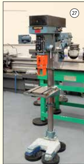
MIDDINGS Type MF5: Pillar Drill. Table 14" x 13" Spindle Taper 3 Morse. Speeds 100-3000rpm. £1,450
