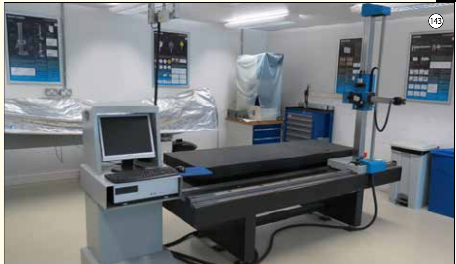
ITP Type HA8: Coordinate Measuring Machine. Fixed to Granite Table Size 2500 x 1150mm. Measuring Table 2000 x 700mm. X Axis 2000mm, Y Axis 700mm, Z Axis 1000mm. Reishaw Probes MH20i & TP20. Software - Axel. £14,950
