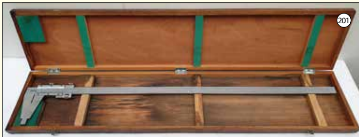
MITUTOYO: Vernier Caliper. Stainless Steel. 1000mm Capacity.
