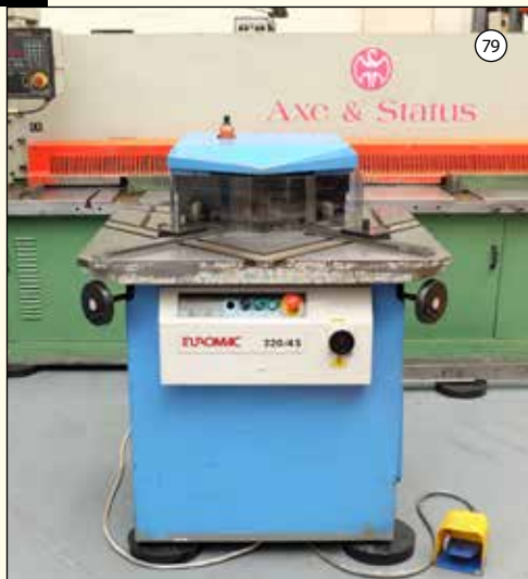
EUROMAC Type 220/4S: Sheet Metal Corner Notcher. Capacity 200mm x 200mm x 4mm. Variable Angle.
