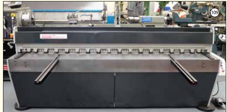
EDWARDS PEARSON Type DD: Power Guillotine. Capacity 2540mm x 3.25mm. Blade Gap Adjustment. Manual Backgauge. Front Supports.
