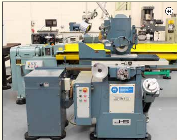
JONES & SHIPMAN 540P: Tool Room Surface Grinder. Capacity 18" x 6". Power Rise & Fall. With Dust Extractor. £7,750
