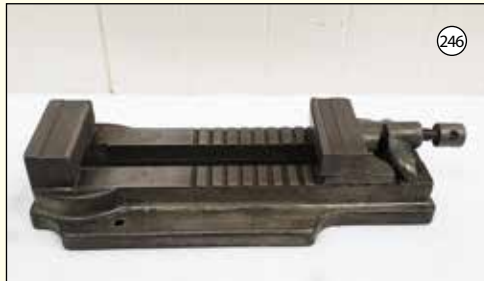
RACK VICE: Max Opening 13 1/4". Jaw Width 6". Jaw Depth 2"
