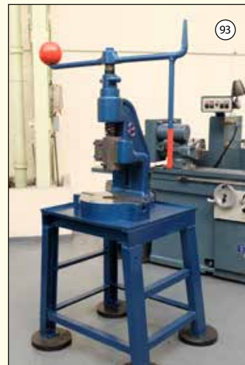
EDWARDS No. 8: Fly Press on Stand. Throat 7". Daylight 9". Stroke 6". £975
