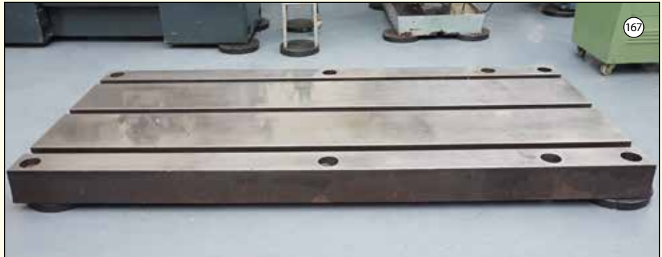
TEE SLOTTED: Bed Plates: Size 96" x 43" x 6" Deep. 3 Tee Slots. Tee Slot Sizes: 1 1/2" Width x 3" Deep. Choice of Two.
