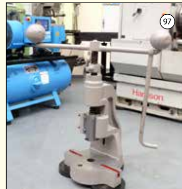
NORTON 4S: Fly Press. Throat 6". Daylight 7". Complete with Press Tool. £495
