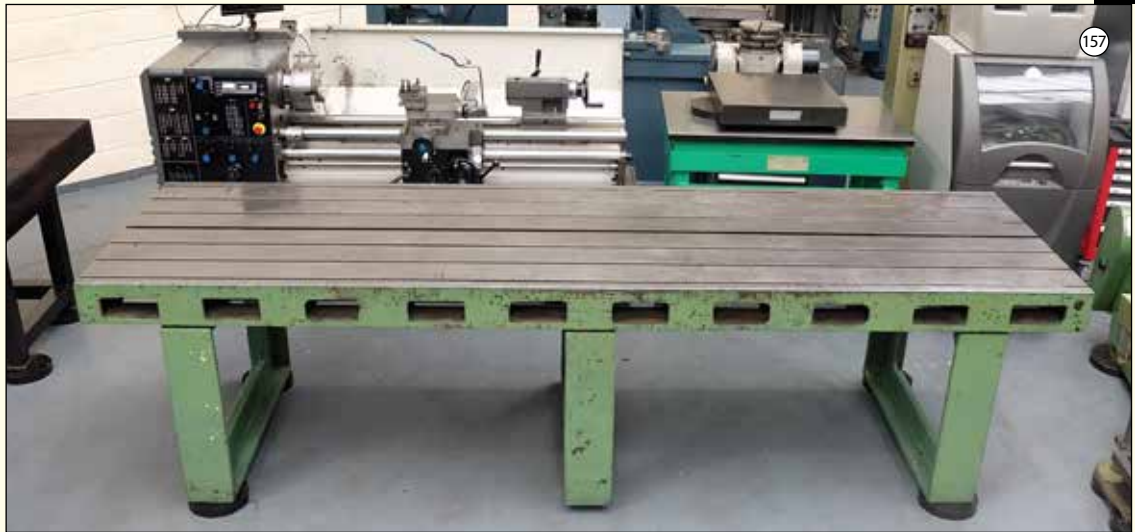
CAST IRON: Surface Table With Central Tee Slot. Size 11' 11 1/2" x 40". Thickness 7". Work Height 38". One Tee Slot in Centre. Six Straight Slots.
