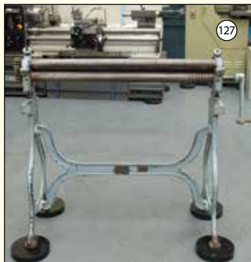
EE Co. Ltd: Initial Pinch Sheet Metal Rolls. Length of Rolls 41 1/2". Diameter of Rolls 2 1/2".
