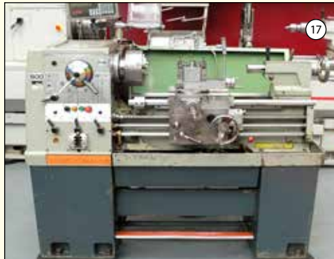
COLCHESTER MASTER 2500: Gap Bed Centre Lathe. Swing Over Bed 13". Swing In Gap 18". Between Centres 30". Speeds 30-2500rpm. 3 & 4 Jaw Chucks. QCTP. 2 Axis DRO. £4,250
