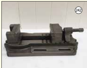
RACK VICE: Max Opening 9 1/2". Jaw Width 6". Jaw Depth 3 1/2".
