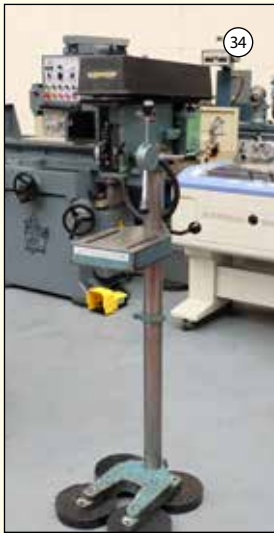
MIDDINGS Model DTF: Pillar Drill. Speeds 500-4000rpm. Throat 7 1/2". 1/2" Drill Chuck. 3 Phase. £750
