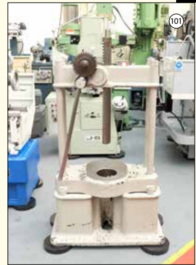
JONES & SHIPMAN: Heavy Duty Geared Broach Press. Between Uprights 24 1/2". Daylight 26 1/2". Hole in Table 6". £950
