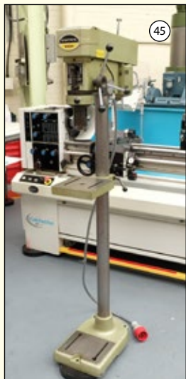
STARTRITE MERCURY: Ten Speed Pillar Drill. 2MT Spindle. Speeds 95-3830rpm. Table Size 9" x 8". £795
