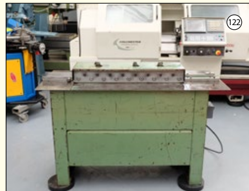
LOCKFORMER: Floor Standing Sheet Metal Rollforming Machine. Capacity 20swg.
