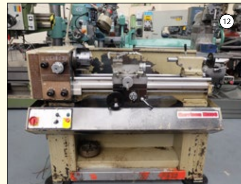
HARRISON M250: Tool Room Centre Lathe. Speeds 40- 500rpm. Swing Over Bed 250mm. Distance Between Centres 800mm. Spindle Bore 35mm. 3 & 4 Jaw Chucks.
