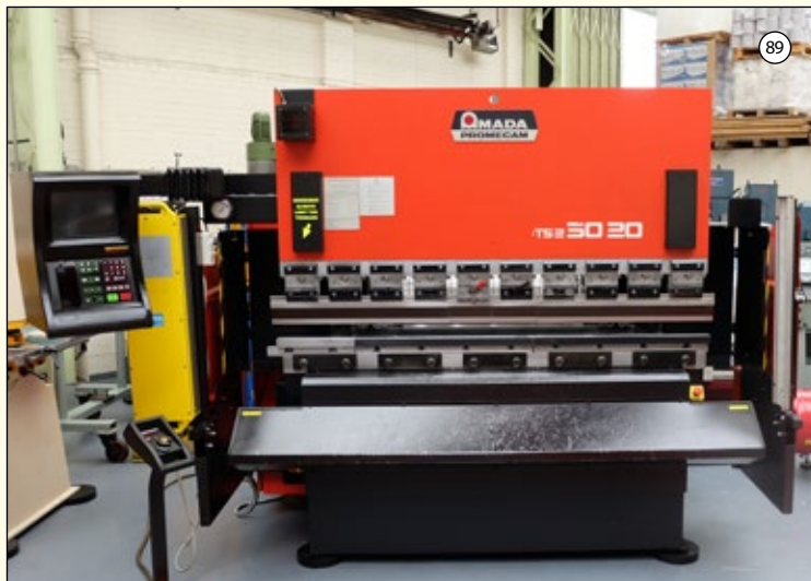
AMADA PROMECAM ITS2: Hydraulic Upstroke Press Brake. Capacity 2000mm x 50 Ton. Open Height 370mm. Stroke Length 100mm. Throat Depth 400mm. Operateur Type OP-4X CNC Control. Power Back Gauge. Front Light Guards. Top & Bottom Tooling. Run Hours 66129. £14,000
