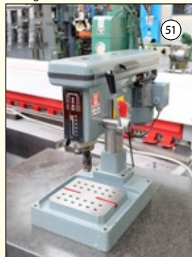
WORNER Type B4: High Speed Bench Drill. Drill Size 0- 5/32 ". Speeds 650-12,000rpm. £575
