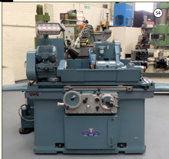
JONES & SHIPMAN Type 1300 EIT: Cylindrical Grinder. Capacity 27" x 10". Double Swivel Wheel Head. Internal Grinding Spindle. 3 & 4 Jaw Chucks. Magnetic Chuck. Ex University.
