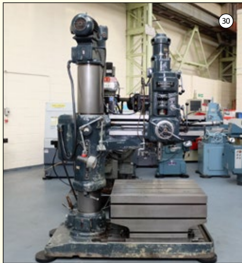
ARCHDALE: 3'6" Radial Arm Drill. 2" Drilling Capacity. Spindle Taper No. 4 Morse. Box Table 40" x 30" x 20" High.
