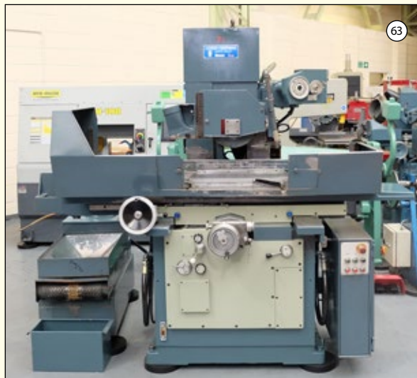
JONES & SHIPMAN Type 1415: Surface Grinder. Capacity 27" x 12". Distance Under New Wheel 11 3/4". Power Rise & Fall to Wheelhead. Mag Chuck & Coolant Tank. £11,750
