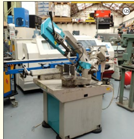
IMET T BS 280/60 ECO: Manual Pull Down Horizontal Bandsaw. Cap 280mm Dia Tube. Single Mitre up to 60 Degrees.
