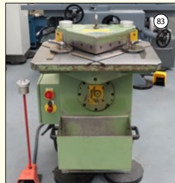
BOSCHERT PN4: Sheet Metal Corner Notcher. Capacity: 225mm x 225mm x 4mm Mild Steel. 225mm x 225mm x 3mm Stainless Steel.
