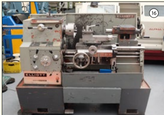
ELLIOTT OMNISPEED Model MS/30/2500: Gap Bed Centre Lathe. Swing Over Bed 15 1/2". Swing in Gap 21 1/2". Between Centres 24". Speeds 30-2500rpm. 3 & 4 Jaw Chucks. 2 & 3 Point Steadies. £3,950
