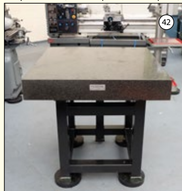
WBJ METROLOGY: Granite Surface Table. Surface Size 1000mm x 1000mm. Thickness 150mm. £950
