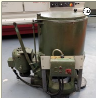
SWARF OIL SPINNER/CENTRIFUGE: Internal Drum Size 300mm Diameter. Depth 300mm. 3 Phase Motor 1 HP.
