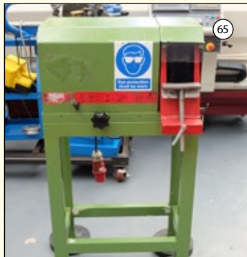
RSA TYPE STL: Single End Deburrer. Wheel Size 10", 3" Wide. Speeds 1500 & 3000rpm. £950
