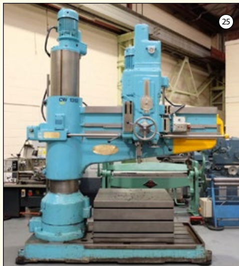
KITCHEN & WADE Type E27 HD: 6' Radial Arm Drill. Arm Radius 72". Drilling Cap 3". 5MT. Speeds 8.5-800rpm. Drilling Depth 18". Box Table 42" x 36" x 22" High. Telescopic Brake. £5,750
