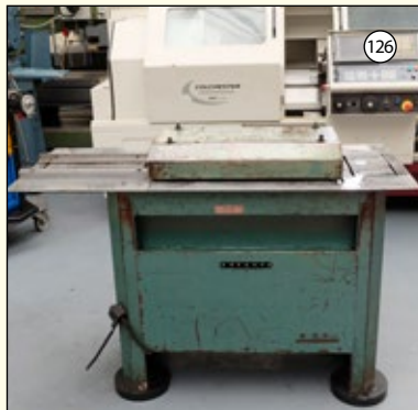
SHORTE: Floor Standing Sheet Metal Rollforming Machine. Capacity 20swg.
