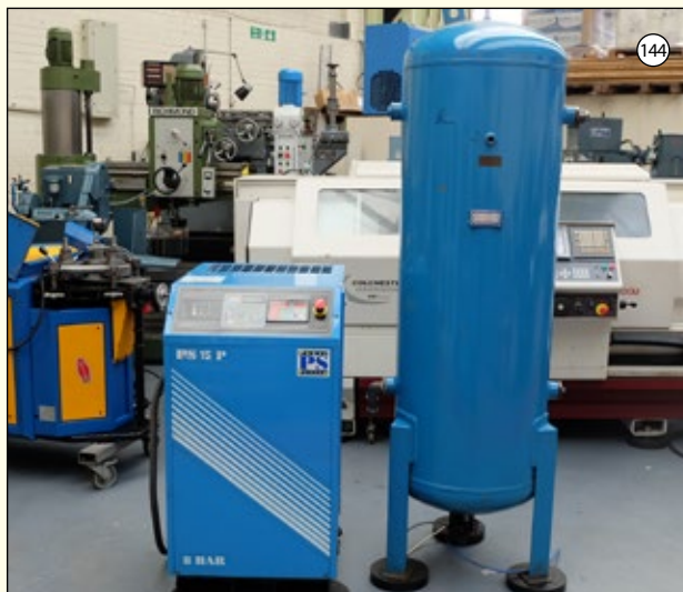
POWER SYSTEMS Model PS 15-8P: Rotary Air Compressor. Motor Size 15kW. Capacity 80 cfm. With 500 Ltr UK Made Vertical Air Receiver. Year 2000.
