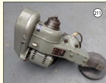
BRIDGEPORT: Slotting Head. Stroke 4". Strokes/Min. 60, 85, 120, 170, 245 & 350.
