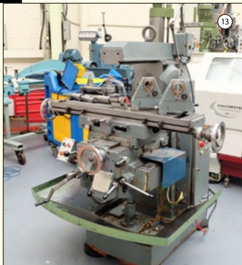
AJAX No.1: Horizontal Milling Machine. Table Size 1100mm x 240mm. Taper 40 ISO. Speeds 48-500rpm. Travel Longitudinal: 750mm, Vertical: 400mm. £2,450
