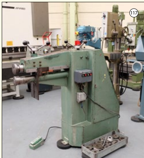
STAVELEY: Powered Swaging Machine. Throat Depth 28". Shaft Size 1 1/4". Foot Control. With Swaging Tools.
