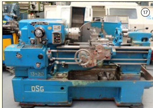
DEAN SMITH & GRACE Type 13-1: Tool Room Centre Lathe. Swing Over Bed 13 1/2". Swing Over Saddle 8 1/4". Between Centres 30". Speeds 24.5-1000rpm. 3 & 4 Jaw Chucks. 3 Point Fixed Steady. £3,750
