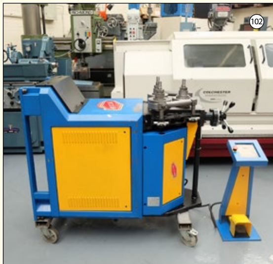
ERCOLINA TYPE CE40MR3: Angle Rolls. Roll Shaft Dia 40mm. Pipe 70mm x 1.5. Flat 50 x 10mm. Angle Capacity 2° x 2° x 1/4". Shaft Speed 10rpm. With 6 Sets of Formers. Year 2001.
