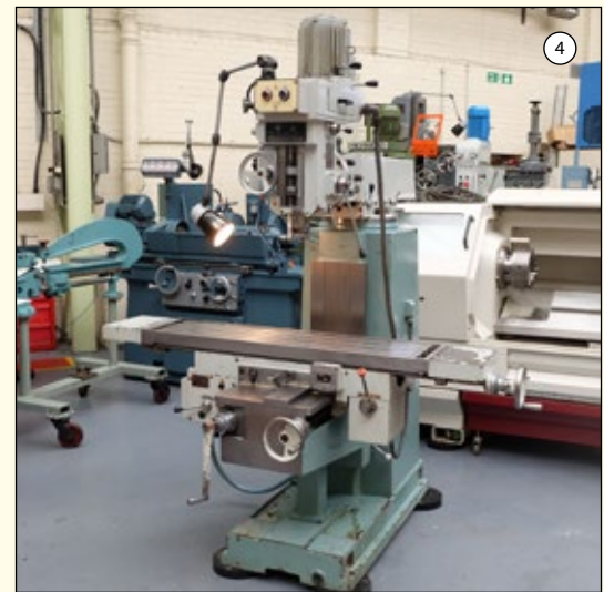
TOS FNK 25: Turret Milling Machine. Table Size 47" x 11 1 / 2 ". Spindle Taper 40 INT. 16 Spindle Speeds 56 - 4500rpm. Imperial Dials. Coolant System, Lo-Vo Light.
