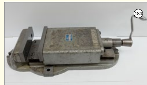
QUICK RELEASE MACHINE VICE: Max Jaw Opening 7 1/2". Jaw Width 6 1/2". Jaw Depth 2". £575
