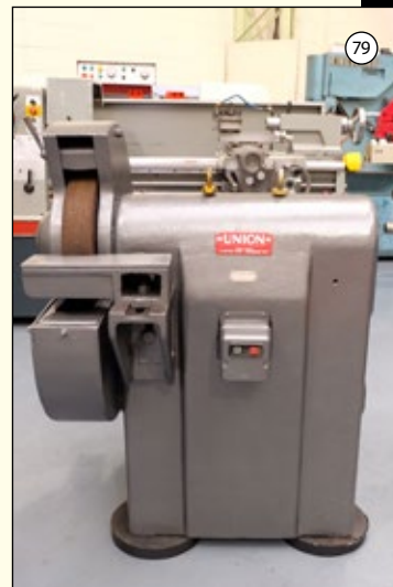
UNION: HD Single Wheel Fetting Grinder. Maximum Wheel Diameter 16" x 3".
