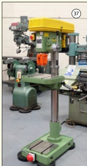
WARCO MODEL DT-25: Floor Standing Pillar Drill. Table 15" x 13". 6 x Speeds 230-2160rpm. £1,750
