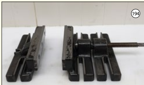
EXTENDABLE CLAMP VICE: Jaw Depth 105mm. Jaw Width 325mm. Extends 180mm £300
