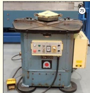
AMADA Type CSW-220: Hydraulic Sheet Metal Corner Notcher. Cap 200mm x 2mm. Rear Square Notcher: 100mm x 50mm. £1,750
