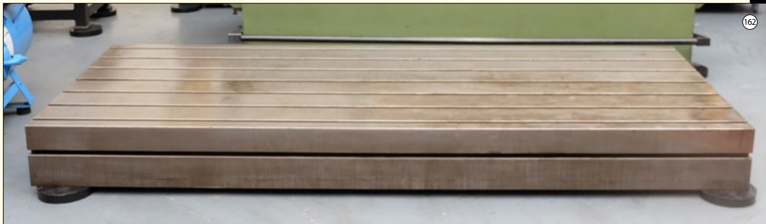
TEE SLOTTED: Machined Floor Plate/Base Plate. 7 x Tee Slots on Surface. 1 x Tee Slot on Front. Size 3300mm x 1200mm x 270mm Thickness.
