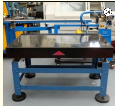
CROWN: Granite Surface Table. Surface Size 5' x 3'. Working Height 34". Grade A. On Steel Levelling Base.
