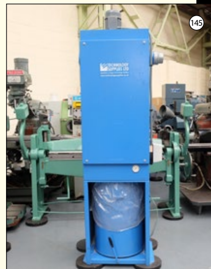
TSPLA Model 530-682: Wood Dust Extractor. Single Phase. Bin Capacity 85l. Height 2120mm.
