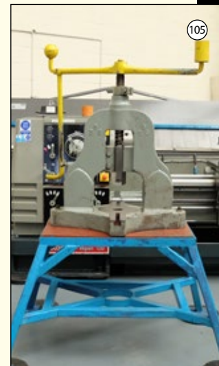
DENBIGH 6 DS: Double Sided Fly Press. 12" Between Sides. 9" Daylight. Bar Press Holes.
