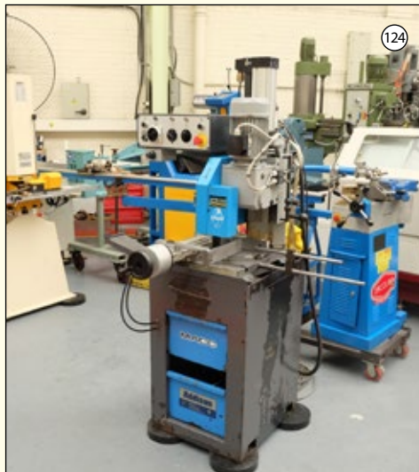
MACC Model NTS 315: Semi-Auto Vertical Cold Saw. Blade Size 315mm Max. Cap Tube & Pipe 100mm. Speeds 33 & 66rpm. Pneumatic Power Vice.
