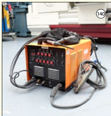
INVERT-R Model TIG200 PAC DC: Portable AC/DC Welding Set. AC/DC Tig Welding. Single Phase. Capacity 10 - 200 Amp. 100% at 154 Amp. £575
