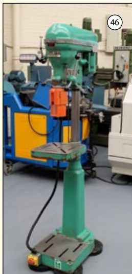
ELLIOTT PROGRESS Type 2G: Pedestal Drill. Cap 7/8 ". Throat 8 1/2 ". Speeds 36-2570rpm. £750
