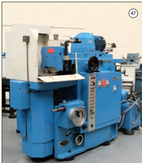
ABWOOD Type RG1: Tool Room Ring Grinder. Table Size 500mm Diameter. Max Spindle Speed 2870rpm. Electro Magnetic Chuck 500mm Diameter. £13,950
