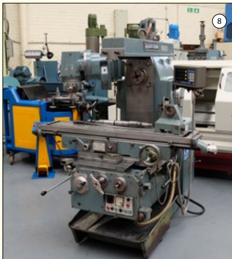
AJAX CLEVELAND No.2: Universal Milling Machine. Table Size 55" x 11". Spindle Taper 40 ISO. Feeds & Rapids. Double Swivel Vertical Head. 3 Axis DRO.
