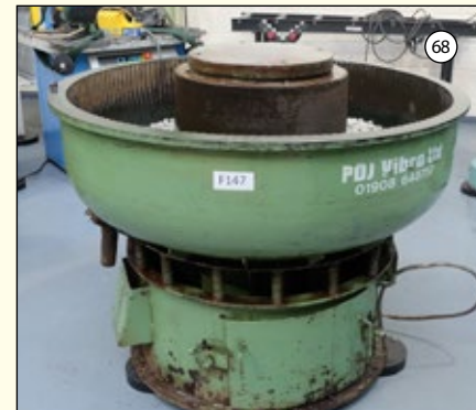
PDJ VIBRO Ltd: Vibratory Circular Bowl Finisher. Capacity 200ltr. Size 1300mm Diameter. Trough Size 300mm. Bowl Height 950mm. £1,950
