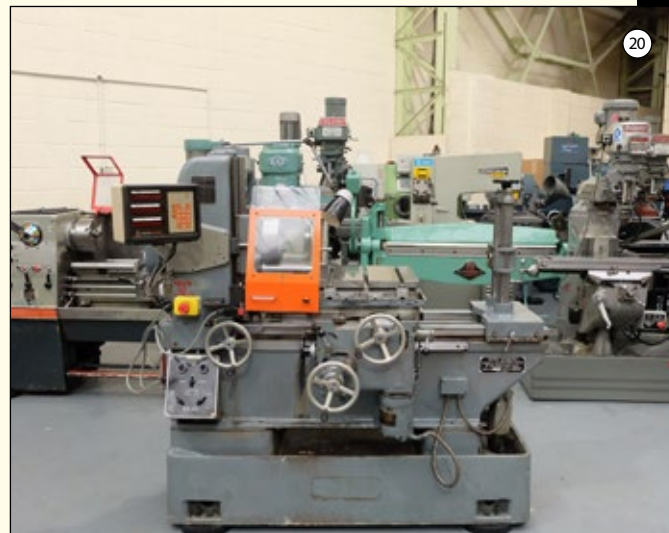
KEARNES S Type FACING CHUCK MODEL: Horizontal Boring Machine. Facing Chuck Cap 8". Main Table Size 16" x 22". Traverse: Longitudinal 24", Transverse 12", Vertical 11". Three Power Feeds to Table. Coolant System & Light. Anilam 3 Axis DRO. £9,750
