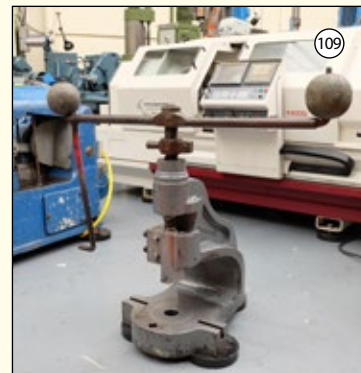
NORTON Type 6DB: Deep Throat Fly Press. Throat 12". Daylight 9".
