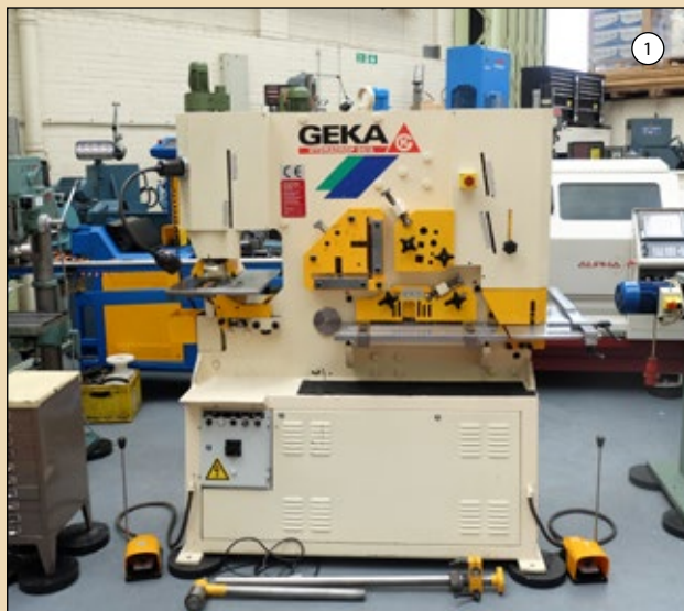
GEKA MODEL HYD 80/A: Universal Steelworker. Punching 40mm Dia x 14mm Thickness. Right Angle 130 x 130 x 12mm. Section Crop 45mm Round & Square. With Touch & Cut End Stop. With Punch & Dies. Excellent Condition. £11,750
