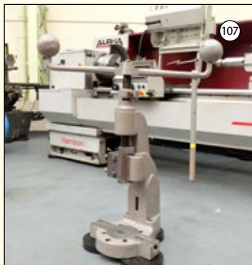
SWEENEY BLOCKSIDE Type 6T: Fly Press. Throat 5". Daylight 12".
