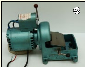
RJH: Bench Top Lapper. 6" Wheel. 0.5HP. Voltage 230/1/50.
