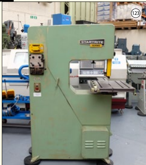
STARTRITE 20 RWS: Vertical Bandsaw. Throat 20". Daylight 10". Speeds 50 - 3000FPM. Blade Welding & Grinding. 3 Phase 1.1KW Motor.
