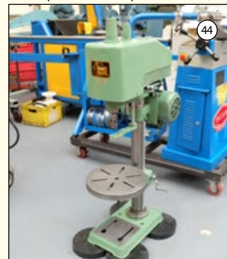
ASTRA Type GWT 30A: Bench Tapping Machine. Throat 7 1/2". Table Diameter 12 1/2". £950
