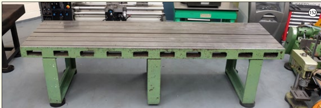
CAST IRON: Surface Table With Central Tee Slot. Size 11' 11 1/2" x 40". Thickness 7". Work Height 38". One Tee Slot in Centre. Six Straight Slots. £1,750
