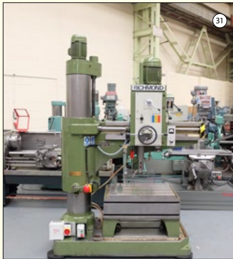
RICHMOND ENVOY: 48" Radial Arm Drill. Radius 48". Spindle Speeds 20-928rpm. Spindle To Base 50". Spindle 4 MT. Spindle Guard. Telescopic Brake.
