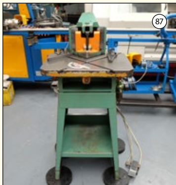
COMACA: Pneumatic Corner Notcher, Foot Control. 120mm x 120mm x 2mm.
