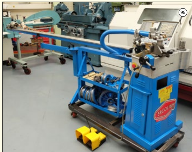
ERCOLINA 060 SUPER BENDER: Tube & Pipe Bending Machine. Bending Capacity 1/4" - 2" Tube. Programmable Bend Angle Display & Spring Back. With 8 Formers & Dies. With A40-P 3 Metre 2 Axis Positioner. Year 2001.
