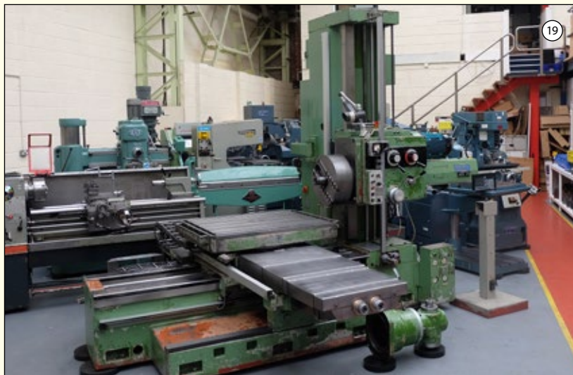
CERUTI Type ABC 75: Wide Bed Horizontal Boring, Milling & Facing Machine. Speeds 15-1500rpm. Spindle Diameter 75mm. Table Size 850 x 1100mm. Cross Traverse 1600mm. Long Traverse 1500mm. Facing Head 450mm. With Swiveling Vertical Milling Head & Tooling. DRO. £16,750
