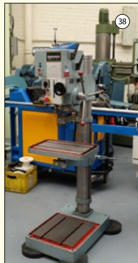
MEDDINGS Type S32 ME: Geared Head Pedestal Drill. 3MT. Speeds 70-2940rpm. £2,250
