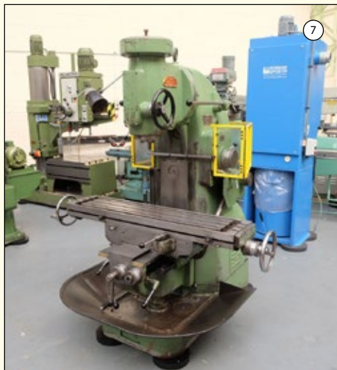
RICHMOND No3V: Vertical Milling Machine. Table Size 48" x 11". Spindle Taper 40 INT. Speeds 30 - 1400rpm. Power Feed to All Axis.
