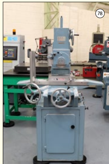
EXE: Precision Manual Surface Grinder. Table Capacity 12" x 6". Fitted to EXE Pedestal Cabinet.
