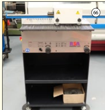
RSA RASAMAX DUO: Sheet Metal Deburrer. 5mm Max Thickness. Speeds 1500 & 3000rpm. Wheel Diameter 250mm. £4,250
