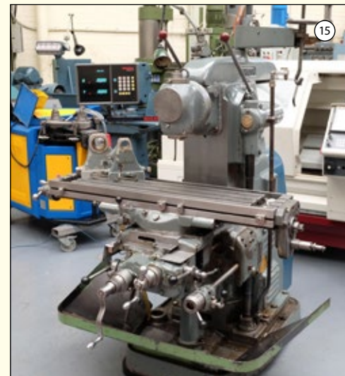
PARKSON Type INA: Universal Milling Machine. Table Size 46" x 10 1/2". Spindle Taper 40ISO. Swiveling Table. Vertical Speeds 56-1510rpm. Swiveling Vertical Head. £2,750
