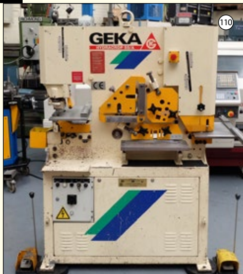
GEKA Model HYD/A: Universal Steelworker. Throat 250mm. Punching 400mm x 10mm Thickness. Shearing 300mm x 15mm. Right Angle 120 x 120 x 10mm. £6,250
