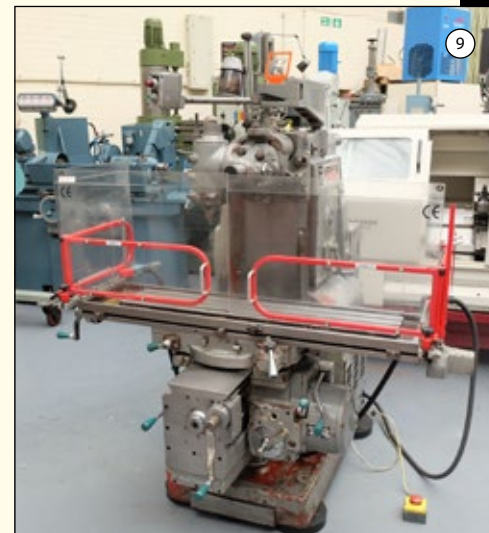
KEARNEY & TRECKER TYPE 205 C-12: Universal Milling Machine. Table Size 52" x 12". Spindle Taper 40 ISO. Speeds 37-1575rpm. Swivel & Tilting Vertical Head.
