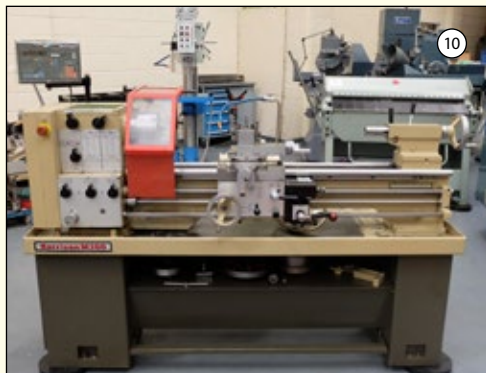
HARRISON M300: Gap Bed Centre Lathe. Swing Over Bed 330mm. Between Centres 1000mm. Spindle Bore 38mm. Speeds 40-2500rpm. QCTP. 3 & 4 Jaw Chucks. Two Axis DRO.
