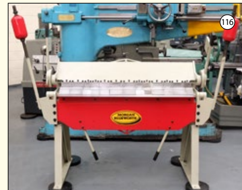
MORGAN RUSHWORTH BPC 1270/2.5: Sheet Metal Box & Pan Folder. Capacity 1270 x 2.5mm. Year 2000. 13 Pieces of Tooling Total Length 1300mm. £1,950
