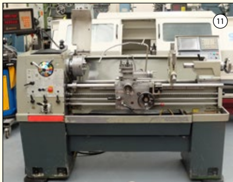
COLCHESTER MASTER 2500: Straight Bed Centre Lathe. Swing Over Bed 13 1/4". Between Centres 40". Spindle Bore 1 5/8". Speeds 25- 2500rpm. 3 & 4 Jaw Chucks. QCTP.
