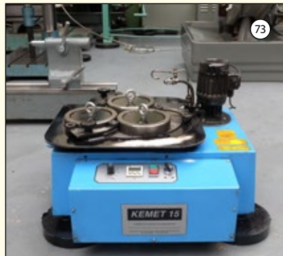
KEMET 15VS: Bench Top Diamond Flat Lapping/Polishing Machine. 380mm Diameter Lapping Table. 240v. Variable Speed. £2,750
