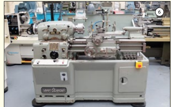
SMART & BROWN 1024: Tool Room Centre Lathe. Swing Over Bed 10". Between Centres 24". Spindle Bore 1 1 / 4 ". Speeds 30-2500rpm. 2 Axis DRO. 3 & 4 Jaw Chucks. Drawbar & Collets. 2 & 3 Point Steadies.
