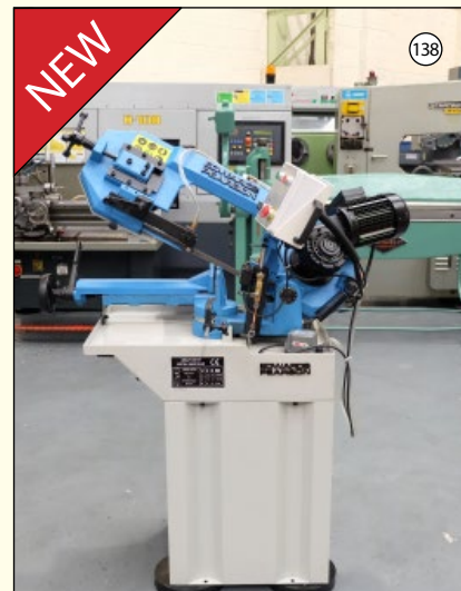
EDWARDS PEARSON MBS210FHE: Gravitational Horizontal Bandsaw. Hydraulic Down Feed. Quick Release Vice Clamping. Cap Round 170 mm. £1,750
