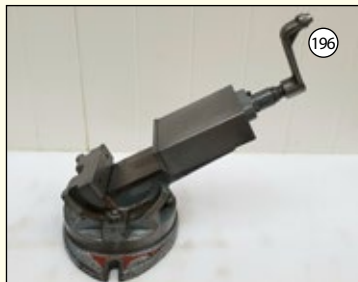
ABWOOD: Tilting & Rotating Vice. Jaw Width 6". Jaw Height 2". £500
