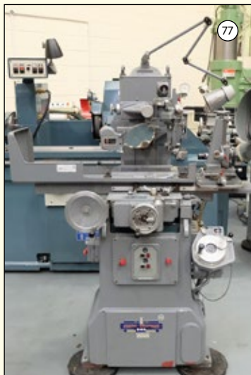
JONES & SHIPMAN 540AP: Surface Grinder. Capacity 18" x 6". Imperial Dials. Power Rise & Fall. Auto Down Feed.
