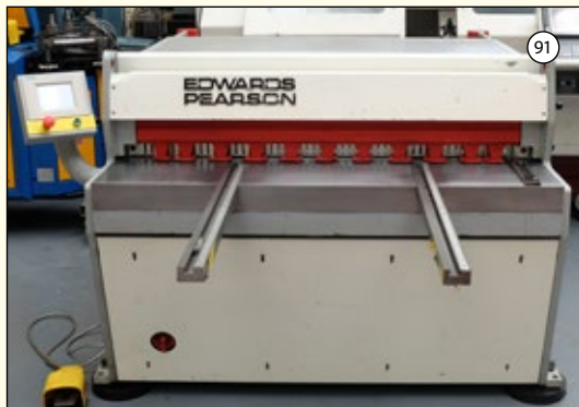
EDWARDS DD Model 3.5/1250: Power Guillotine. Capacity 3.5mm x 1250mm. Blade Gap Adjustment 0.8-4mm. Siemens Simatic DRO. Power Back Gauge. Infra Red Rear Guarding. Year 2002. £7,950
