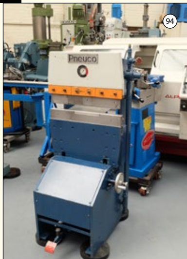
PNEUCO Model 02-15: Pneumatic 15 Ton Upstroke Press Brake. Capacity 24" x 11 SWG.
