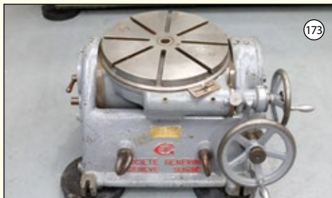
SIP Type P1-5B. Tilting Rotary Table. Diameter 450mm. Work Height 400mm. Tee Slotted. £1,250
