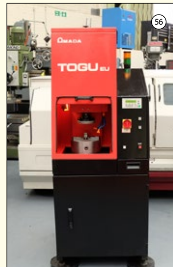
AMADA TOGU-EU: Automated Tool Grinder. Grinding Cap 2mm - 160mm. Speed 3000rpm. Siemens TD200 Programmable Display. £8,250
