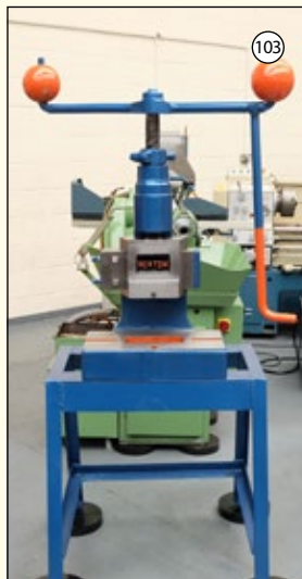
NORTON No. 4GP: Fly Press On Stand. Table Size 19" x 10". Throat 5". Daylight 7".
