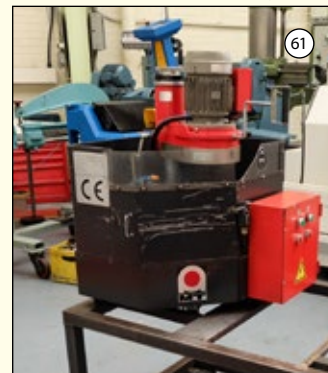
AMADA Type TEG - 160ES: Punch & Die Grinder. Cap 160mm. Kitagawa 165mm Three Jaw Chuck. Coolant System. £2,450
