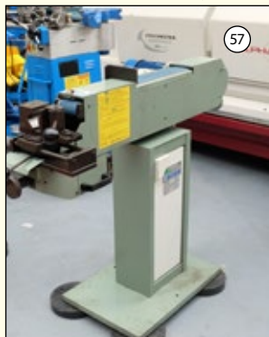
ACETI Model 60: Pedestal Pipe Notching & Finishing Machine. Belt Width 90mm. Flat Surface 380 x 90mm.
