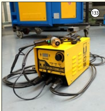
TAYLOR STUDFAST CBM: 8 Stud Welding System. Weld Range: Mild Steel 2-8mm, Stainless 2-6mm. Alluminium 2-6mm. Single Phase.
