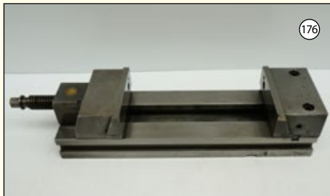
MACHINE VICE: Jaw Width 150mm. Max Opening 260mm. Jaw Height 55mm. £400
