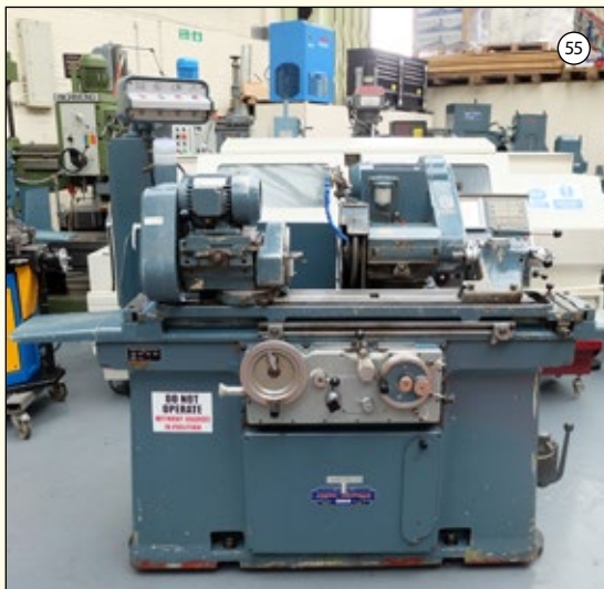
JONES & SHIPMAN Type 1310 EIU: Universal Cylindrical Grinder. Capacity 18" x 8". Wheel Head Speeds 1750 & 2300rpm. Swivel Head with Internal Spindle. Swivel Workhead Speeds 30-415rpm.
