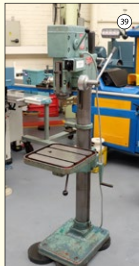
BEREMA GIMA Type P12: Gear Driven Pillar Drill. Spindle 3MT. Speeds 55-1800rpm. £1,650
