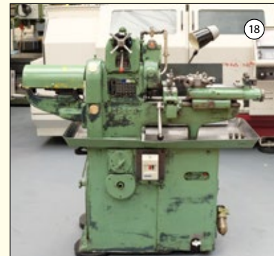
HERBERT No.0 : Capstan Lathe. Capacity 1 1/2". Stroke of Capstan 4". 12 Speeds 140 - 6000rpm. Coolant & Light. Collet Chuck. £1,750
