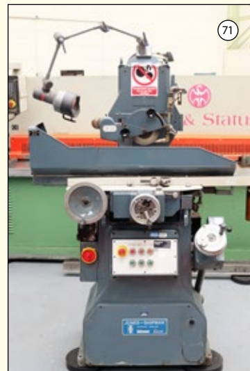
JONES & SHIPMAN 540P: Surface Grinder. Capacity 18" x 6". Power Rise & Fall Head. Dust Extractor. £4,950
