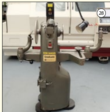
L.R.E. GRADUATE: Short Bed Wood Lathe. Centre Height 250mm. Between Centres 400mm. Speeds 425, 790, 1330 & 2250rpm. £1,250
