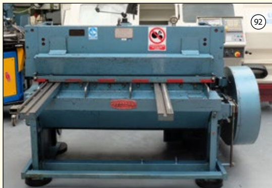
KEETONA: Mechanical Power Guillotine. Capacity 50" x 14 SWG Mild Steel, 50" x 16 SWG Stainless Steel. Manual Back Gauge. Front Supports. Ex. University. £2,250
