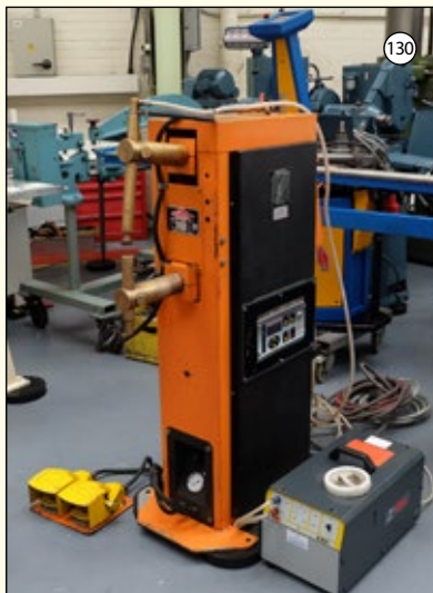
MERITUS Type RNS 30A3: Pneumatic Clamping 30 KVA Sheet Metal Spot Welder. Micro 8 Control. Stel RWC Cooling System.
