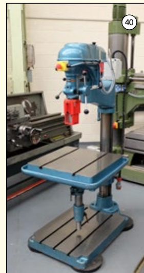
MEDDINGS: Type A10: Articulated Arm Drill. 2MT. Throat 24". Speeds 80-4000rpm. £1,850
