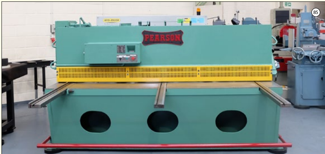
PEARSON Type 8 x 25: Hydraulic Power Guillotine. Capacity 8' x 1/4". Power Back Gauge. Front Supports & Squaring Arm.
