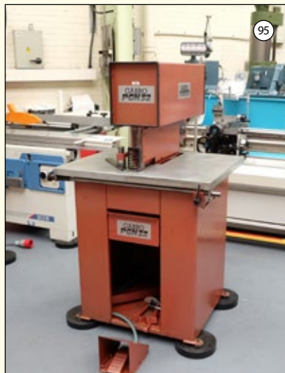
GABRO PGN 32: Pneumatic Sheet Metal Guillotine/ Notcher. Capacity in Mild Steel 3.2mm. Cuts Per Min Approx 25.
