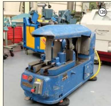
WICKSTEED Model S12 H3: Power Hacksaw. Capacity 12". High & Low Speeds. Swivel Vice. Coolant Pump Replaced with External Pump.
