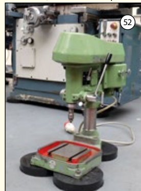
FLOTT Type TB6: High Speed Bench Drill. Speeds 450-9000rpm. Throat 6 1/2 ". Capacity 1/4 ". £425
