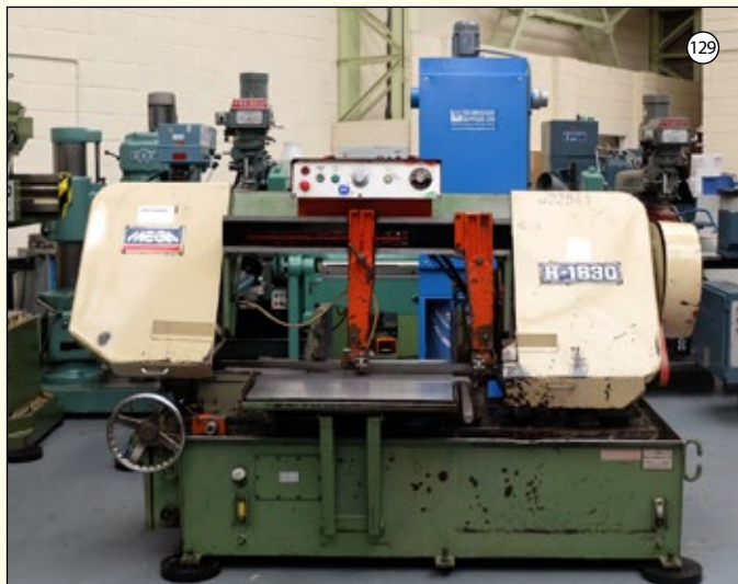
MEGA TYPE H-1830: Semi Automatic Horizontal Bandsaw. Capacity Round 460mm. Capacity Square 430mm. Capacity Rectangle 765mm x 410mm.
