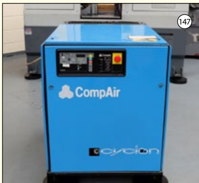
COMPAIR Model Cyclon 111: Rotary Air Compressor. Max Pressure 7.5 Bar. Flow Rate 1.77m3/Min. Motor Power 13.59kw.
