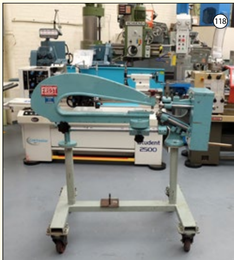
FROST Type 283: Manual Circle Cutter. Max Capacity 56" Diameter. Thickness 16 SWG. Throat 28".
