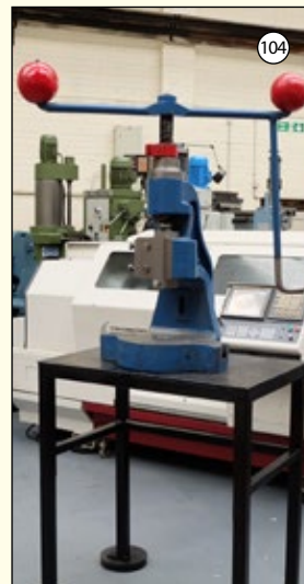
NORTON Type 6S: Fly Press. Throat 6". Daylight 9". Fitted to Steel Stand.
