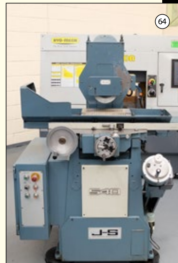
JONES & SHIPMAN 540P: Surface Grinder. Capacity 18" x 6". With Coolant Tank. Power Rise & Fall to Wheel Head. £7,750
