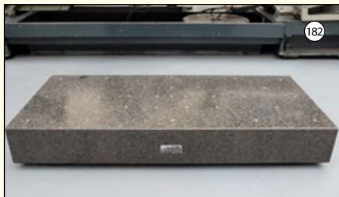
GRANITE TABLE: Surface Size 59" x 26", Thickness 7 1/2", Grade A. With 30 Clamp Studs. £600
