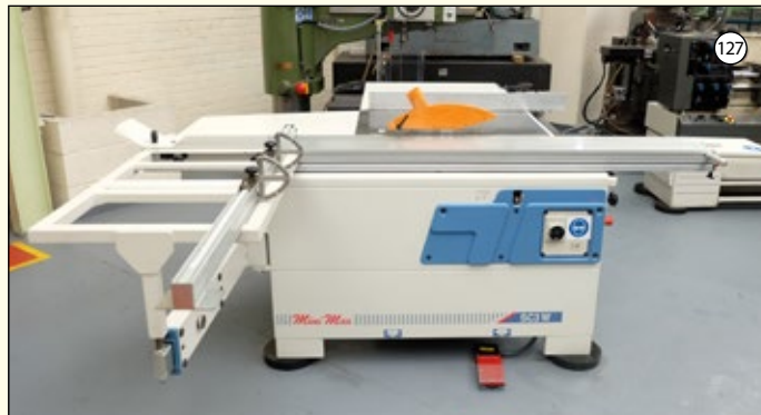
SCM MINI MAX SC/3W: Woodworking Combination Sliding Table Saw. 1750mm Sliding Carriage. 1250mm With of Cut to Parallel Fence. 315mm Sawblade Size. Tilting Blade to 45 Degrees .3 Phase 400V Electrics. Year 2007.
