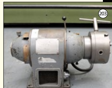
MOTORISED WORKHEAD: 3 Jaw Chuck 160mm. 14" Swing. 2 Speed.
