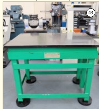
SURFACE FLATNESS LTD: Cast Iron Surface Table. Size 48" x 30". Grade 1. On Steel Stand. £1,750
