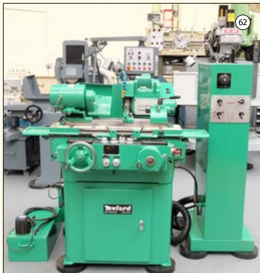
MYFORD MG12-HA: Hydraulic Cylindrical Grinder. Maximum Grinding Capacity 3" Diameter. Swing Over Table 5". Max Table Travel 13 3/4". Capacity Between Centres 12". £5,250
