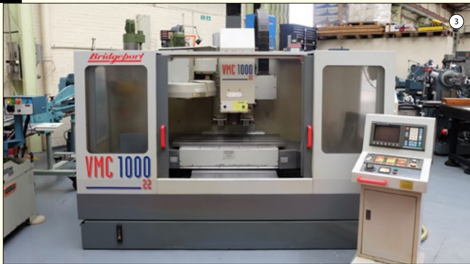
BRIDGEPORT VMC 1000/22: Vertical Machining Centre With FANUC OM-C Control. Table Size 1150mm x 490mm. X Axis Table 1020mm. Y Axis Table 510mm. Z Axis Head 500mm. Spindle Taper BT-40. Spindle Speeds 40-6000rpm. 22 Position ATC. Coolant Tank & Pump. Operation, Programming & Parts Manual.
