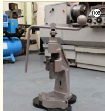
NORTON Type 2L: Fly Press. Daylight 10". Throat 5".
