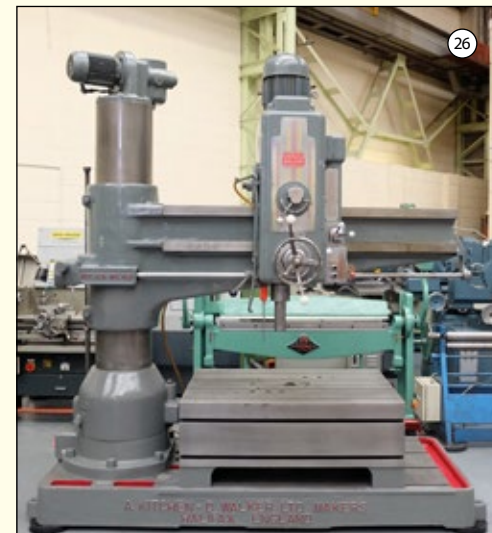
KITCHEN & WALKER Type E3: Radial Arm Drill. Radius 6'. Drilling Cap 1/4" - 3". Spindle 5MT. Speeds 12-1000rpm. Table 50" x 36" x 20" High. DC Brake. Coolant System. £5,750
