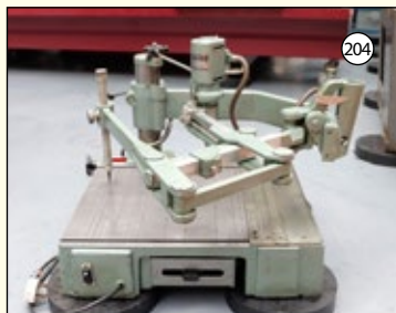
DAVID DOWLING: Bench Top Pantograph. Table Size 20" x 16". Single Phase.
