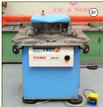
EUROMAC Type 220/45: Sheet Metal Corner Notcher. Capacity 200mm x 200mm x 4mm. Variable Angle.
