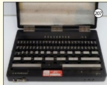
COVENTRY GAUGE & TOOL Co: Complete Imperial Slip Gauge Set. Set of 83.
