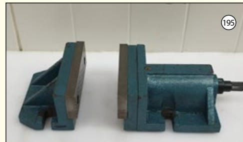
EXTENDABLE CLAMP VICE: Jaw Depth 100mm. Jaw Width 200mm. £450
