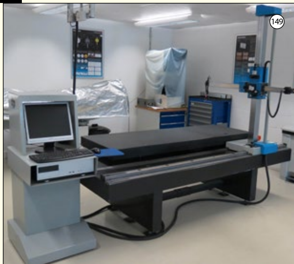
ITP Type HA8: Coordinate Measuring Machine. Fixed to Granite Table Size 2500 x 1150mm. Measuring Table 2000 x 700mm. X Axis 2000mm, Y Axis 700mm, Z Axis 1000mm. Reinsshaw Probes MH20i & TP20. Software - Axel. £13,750
