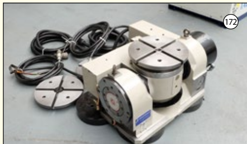
JONES & SHIPMAN: 4th AXIS Tilting Rotary Table. Size 260mm. 310mm High. ype 8414-009DC/306. £3,950
