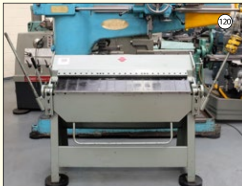
SELSON BESCO Model B&P 416: Manual Box & Pan Folder. Capacity 1270mm x 1.5mm or 50" x 16swg. 16 Pieces of Tooling: Total Length 1270mm.
