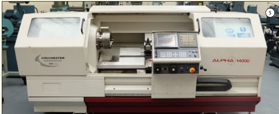
HARRISON ALPHA 1000 SERIES MODEL 1400U: CNC Lathe. Swing Over Bed 400mm. Swing Over Cross Slide 245mm. Between Centres 1250mm. Spindle Bore 55mm. Speeds 15-2500rpm (3 Ranges). Tailstock Taper No. 5 Morse. GE FANUC 21i-TB Touch Screen Control. QCTP. Interlocking Guards.
