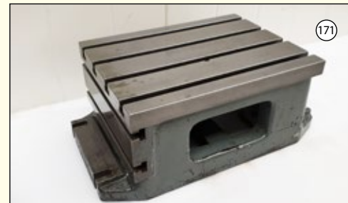
TEE Slotted Riser Block: 400mm x 300mm x 200mm High. £450
