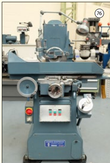
JONES & SHIPMAN 540AP: Surface Grinder. Capacity 18" x 6". Power Rise & Fall. Mag Chuck. Dust Extractor.
