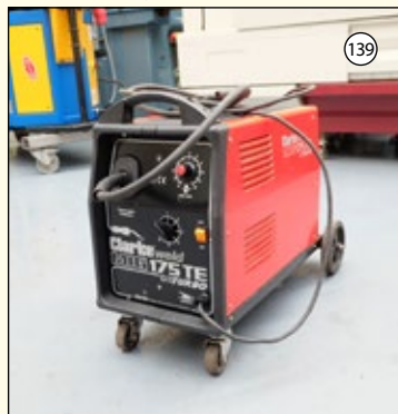
CLARKWELD Model MIG 175TE: Turbo MIG Welding Set. Capacity 30 to 170 Amp. 100% at 65 Amp. Single Phase. £250
