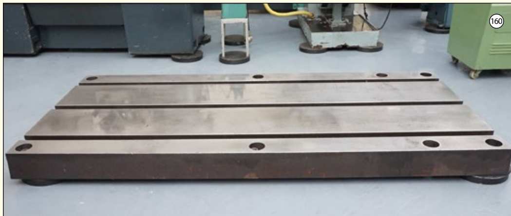
TEE SLOTTED: Bed Plates: Size 96" x 43" x 6" Deep. 3 Tee Slots. Tee Slot Sizes: 1 1/2" Width x 3" Deep. Choice of Two.
