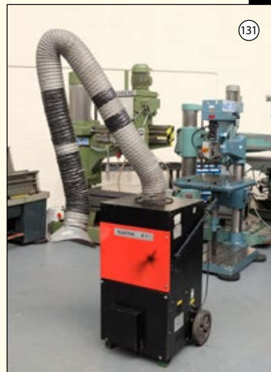
ELECTAC Model E1: Mobile Welding Fume Extractor/Filter. Articulated Suction Boom 2.5 Mtr. 750 Watts. 115 Volts.
