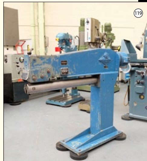
EDWARDS BESCO: Power Seam Closing Machine. Throat Depth 36". Capacity 3/8". Wheel Width 3/4".
