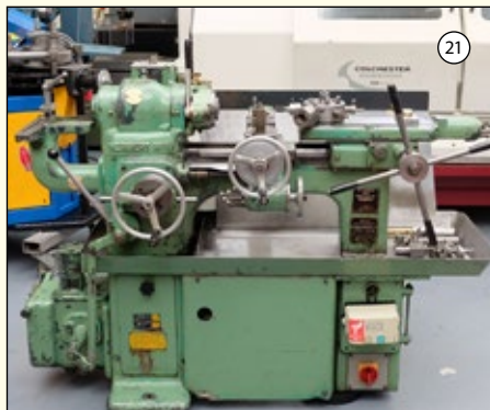
HERBERT No. 1: Capatan Lathe. Capacity 1". Stroke of Capstan 6". 12 Spindle Speeds 57 - 4020rpm. With Collet Chuck. £1,950
