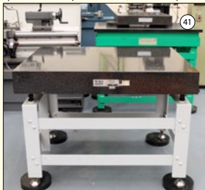
WBJ: Granite Surface Table. Grade 1. Surface Size 48" x 36". Thickness 6". On Levelling Stand. £1,250
