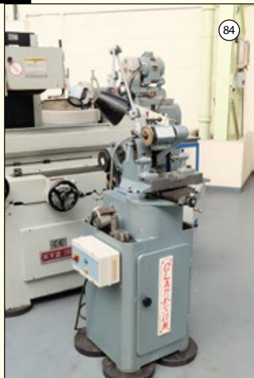
CLARKSON MKII: Tool & Cutter Grinder. Capacity 12" x 6". Pair of Centres. Universal Head.
