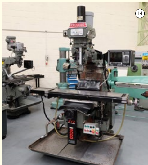
XYZ PRO 3000: Two Axis CNC Milling Machine. Table Size 54" x 12". Speeds 70-3600rpm. Long Travel 32". Cross Travel 17". ProtoTrak MX2 Two Axis Programmable Control. £5,250
