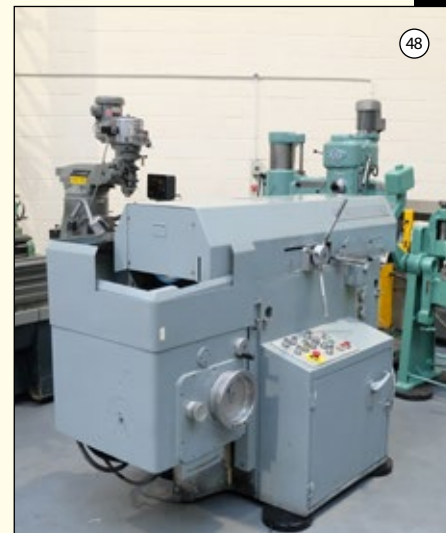
SNOW Model RT 400: Ring Grinder. Table Size 400mm Diameter. Max Height Under Wheel 200mm. Table Speeds 70-250rpm. 400mm Electro Mag Chuck. £8,750
