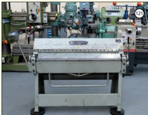
MORGAN RUSHWORTH MODEL 418: Box & Pan Folder. Capacity 4' x 18swg. With Manual Back Gauge.
