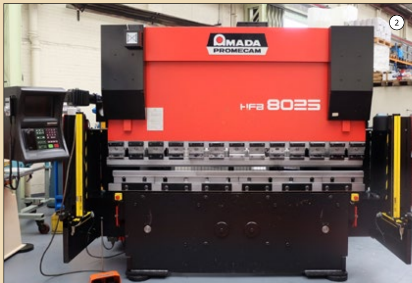
AMADA Model HFB 80/25: Hydraulic Downstroke Press Brake. Capacity 2500mm x 80 Ton. Distance Between Frames 2120mm. Open Height 470mm. Stroke Length 200mm. Throat 420mm. Operateur Type OP-6X CNC Control. Power Back Gauge. Front Light Guards. Tooling £23,950
