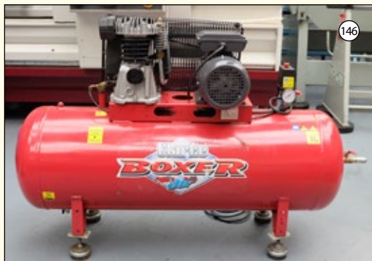
CLARKE BOXER: Garage Type Air Compressor. Model 41P0519. Motor 2.2kW. Single Phase. Air Receiver Size 150Ltr.
