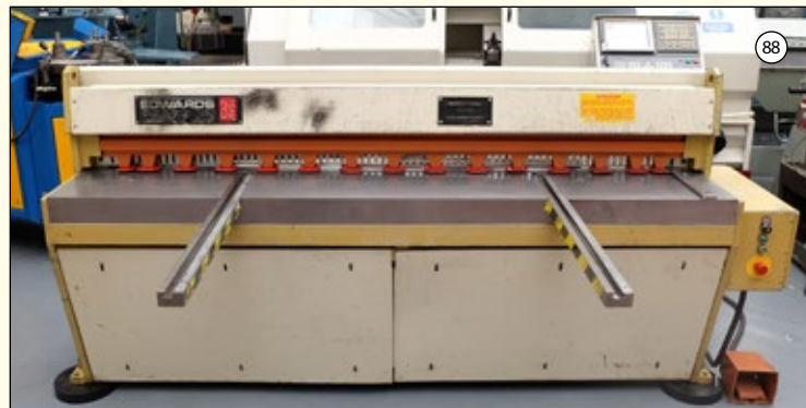
EDWARDS PEARSON DD 3.5/2000: Power Guillotine. Capacity 3.5mm x 2000mm. Blade Gap Adjustment 0.8mm-4mm. Manual Back Gauge. 1000mm Front Supports. Foot Control. Motor Size 7.5kW. Year 1992.
