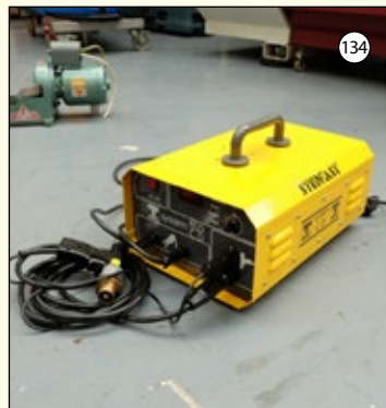
TAYLOR STUDFAST 803 CD: Stud Welding System. Weld Range: Mild Steel 2.5-10mm, Stainless 2.5- 8mm. Alluminium 2.5-7mm. Single Phase.
