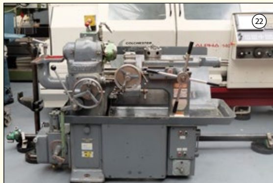
HERBERT No. 1: Capatan Lathe. Capacity 1". Stroke of Capstan 6". 12 Spindle Speeds 57 - 4020rpm. With Bar Feed & Collet Chuck. £2,250
